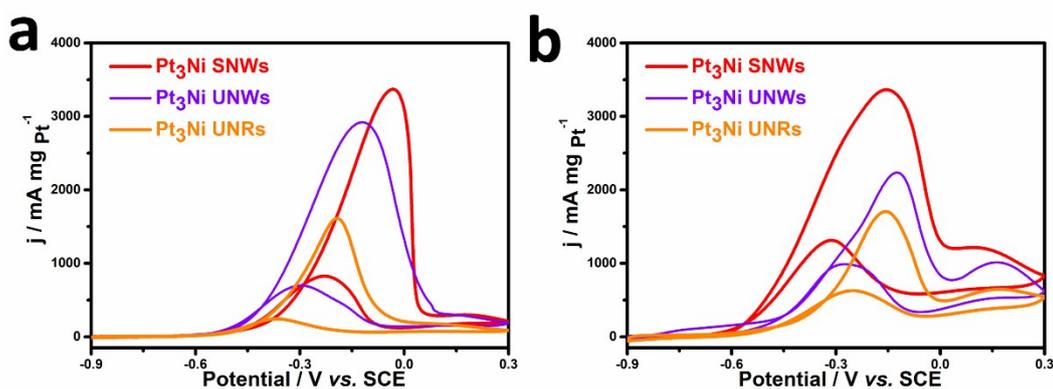
**Fig. S8** CV curves Pt<sub>3</sub>Ni SNWs, Pt<sub>3</sub>Ni UNWs, Pt<sub>3</sub>Ni UNRs catalysts (unloaded on C) operated in (a) 1 M KOH and 1 M EG and (b) 1 M KOH and 1 M glycerol solution.
