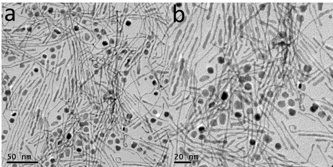
**Fig. S7** TEM images of the products with the same reaction condition as that of Pt<sub>3</sub>Ni UNRs without the addition of glucose.
