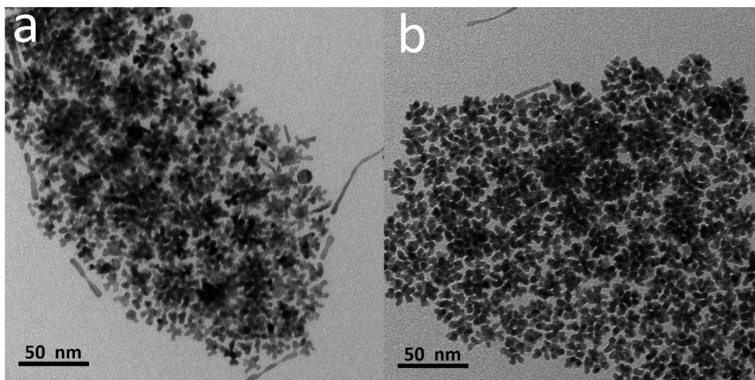
**Fig. S4** TEM images of the products with the same reaction conditions as that of  $\text{Pt}_3\text{Ni}$  SNWs without the introduction of  $\text{W}(\text{CO})_6$ .
