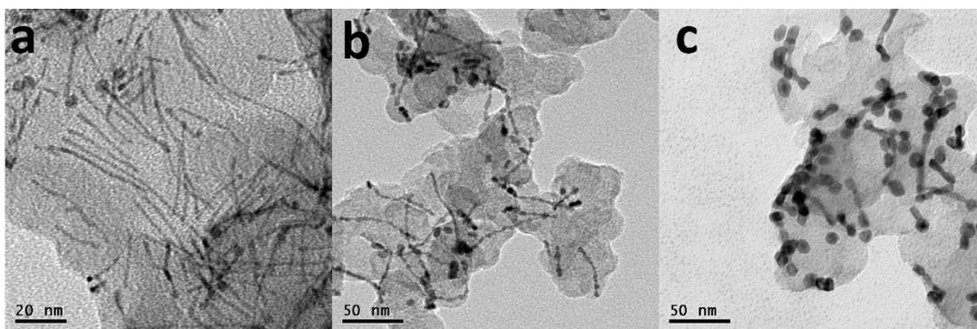
**Fig. S12** Representative TEM images of (a) Pt<sub>3</sub>Ni UNWs, (b) Pt<sub>3</sub>Ni SNWs, and (c) Pt<sub>3</sub>Ni UNRs catalysts after durability tests.
