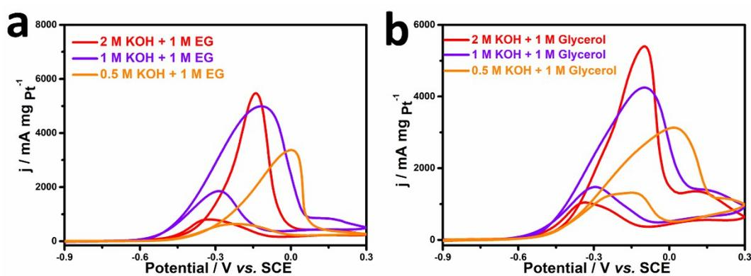
**Fig. S9** CV curves of Pt<sub>3</sub>Ni SNWs catalysts towards (a) EGOR and (b) GOR with
