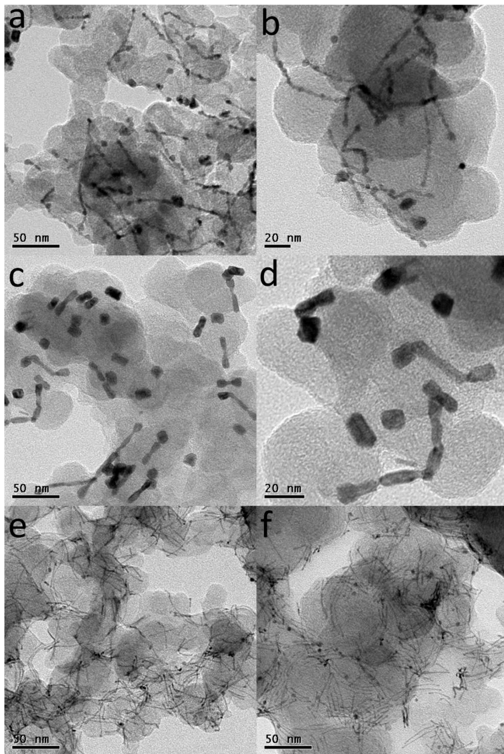
**Fig. S10** Representative TEM images of (a and b) Pt<sub>3</sub>Ni SNWs, (c and d) Pt<sub>3</sub>Ni UNWs, and (e and f) Pt<sub>3</sub>Ni UNRs catalysts before electrochemical measurements.
