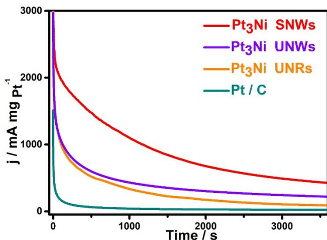
**Fig. S11** CA curves of Pt<sub>3</sub>Ni SNWs, Pt<sub>3</sub>Ni UNWs, Pt<sub>3</sub>Ni UNRs, and commercial Pt/C catalysts recorded in 1.0 M KOH +1.0 M glycerol solution.
