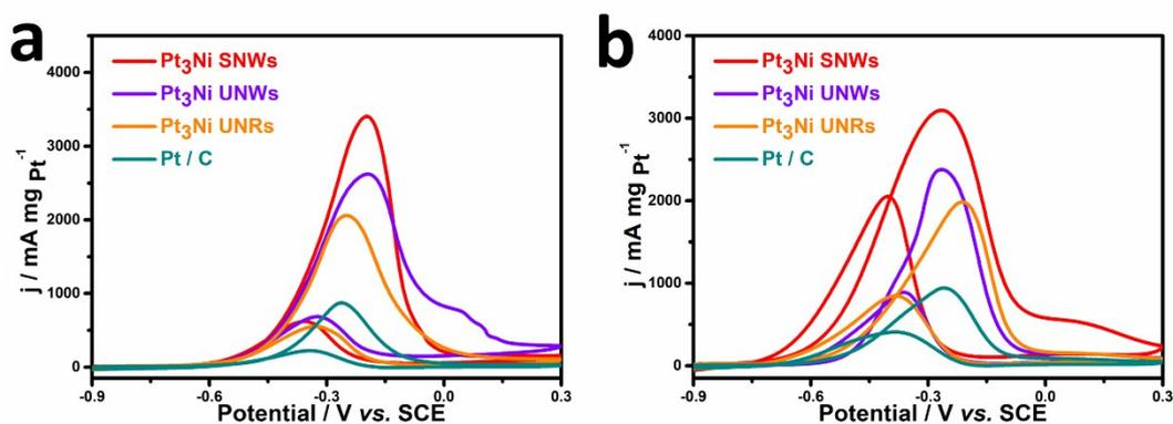
**Fig. S13** CV curves of Pt<sub>3</sub>Ni SNWs, Pt<sub>3</sub>Ni UNWs, Pt<sub>3</sub>Ni UNRs and commercial Pt/C catalysts operated in (a) 1 M KOH and 1 M methanol, (b) 1 M KOH and 1 M ethanol solution.
