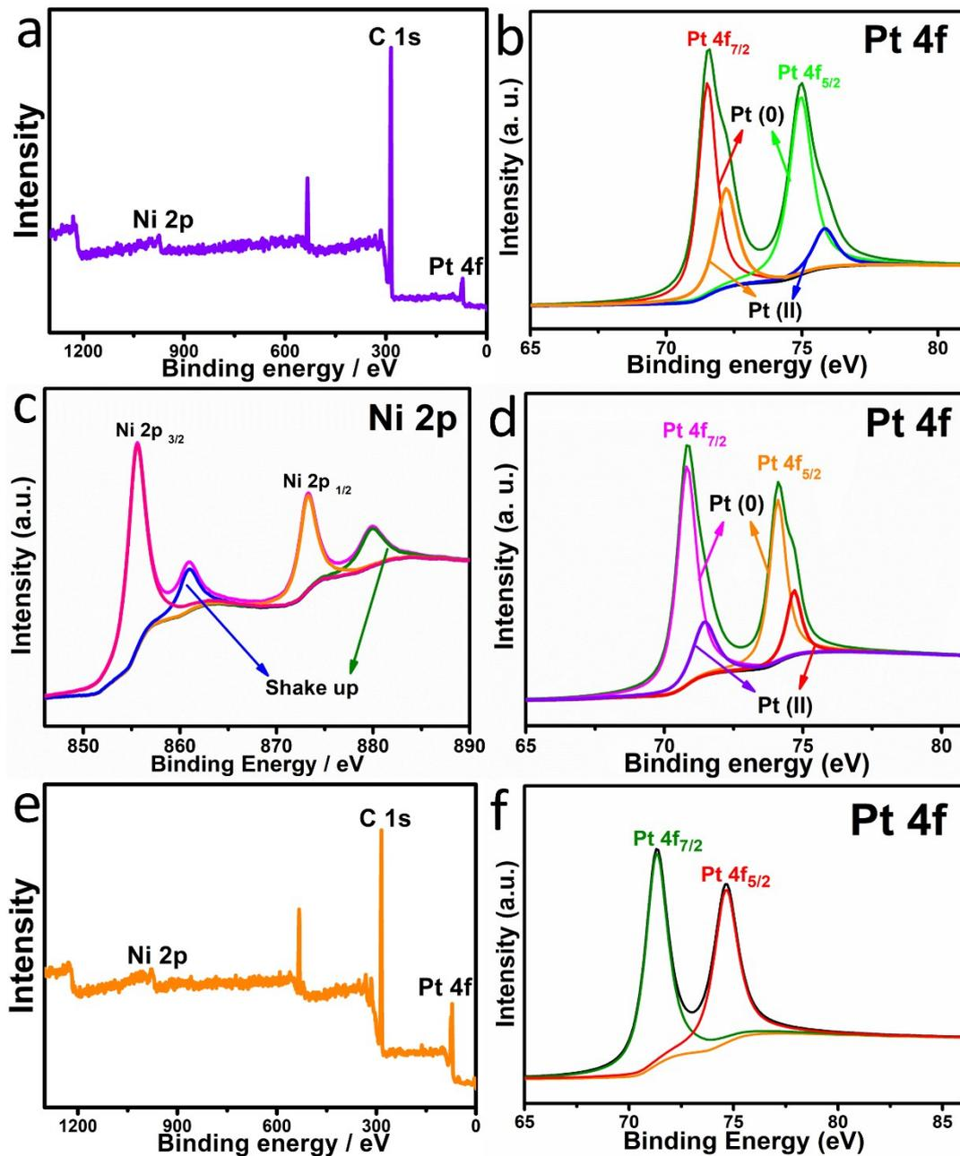
**Fig. S2** XPS spectrum of (a) survey scan, (b) Pt 4f in Pt<sub>3</sub>Ni UNWs, and (c) Ni 2p, (d) Pt 4f in Pt<sub>3</sub>Ni SNWs, (e) survey scan, (f) Pt 4f in Pt<sub>3</sub>Ni UNRs.
