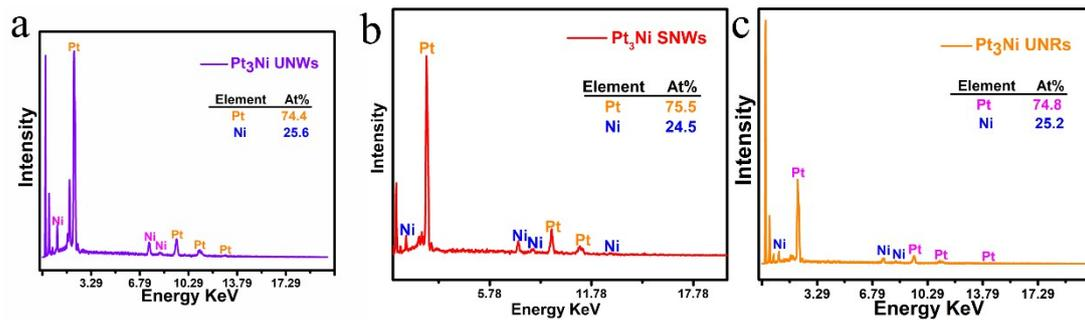
**Fig. S3** SEM-EDX spectrum of (a)  $\text{Pt}_3\text{Ni}$  UNWs, (b)  $\text{Pt}_3\text{Ni}$  SNWs, and (c)  $\text{Pt}_3\text{Ni}$  UNRs.
