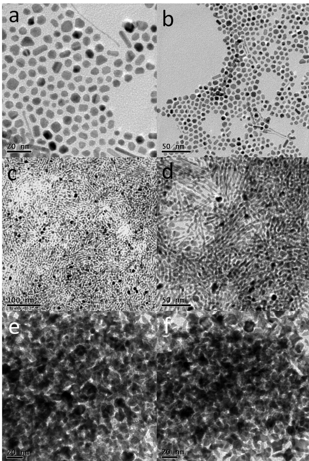
**Fig. S5** TEM images of the products with the same reaction conditions as that of (a and b) Pt<sub>3</sub>Ni UNRs, (c and d) Pt<sub>3</sub>Ni UNWs, and (e and f) Pt<sub>3</sub>Ni SNWs in the absence of CTAC.
