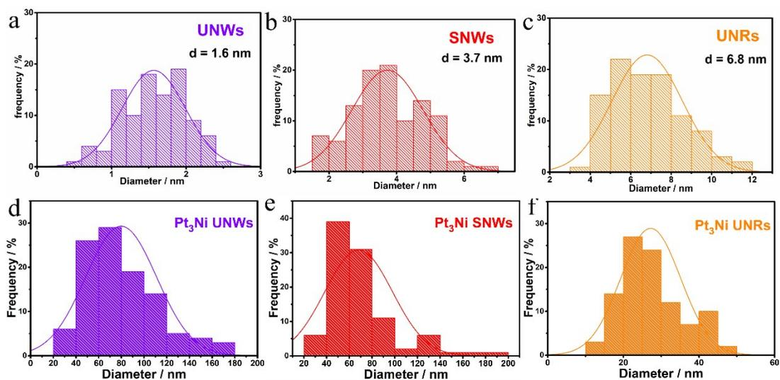
**Fig. S1** Size distribution of (a) Pt<sub>3</sub>Ni UNWs, (c) Pt<sub>3</sub>Ni SNWs, and (e)Pt<sub>3</sub>Ni UNRs in width, and size distribution of (d) Pt<sub>3</sub>Ni UNWs, (e) Pt<sub>3</sub>Ni SNWs, and (f)Pt<sub>3</sub>Ni UNRs in length.
