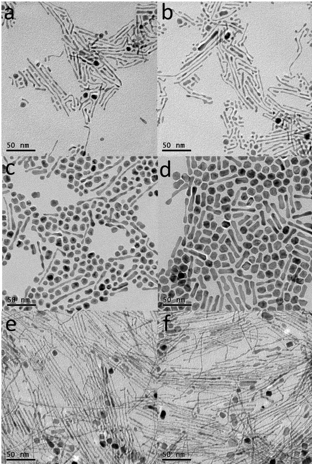
**Fig. S6** TEM images of the products with the same reaction conditions as that of (a and b) Pt<sub>3</sub>Ni SNWs, (c and d) Pt<sub>3</sub>Ni UNRs, and (e and f) Pt<sub>3</sub>Ni UNWs without the addition of ODE.
