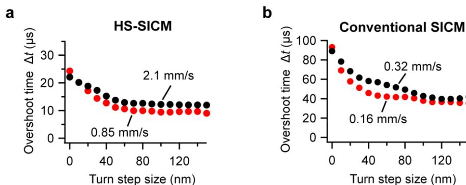
**Figure S1:** Evaluation of the overshoot time from approach curves (example curves shown in Fig. S2) recorded with (a) the HS- and (b) the conventional SICM setup in hopping mode with turn step for different turn step sizes and for two different approach speeds (see red and black curves; approach speed indicated in the graph). Increasing the turn step size beyond  $\approx 70$  nm (HS-SICM) or  $\approx 100$  nm (conventional SICM) does not further decrease the overshoot time.
