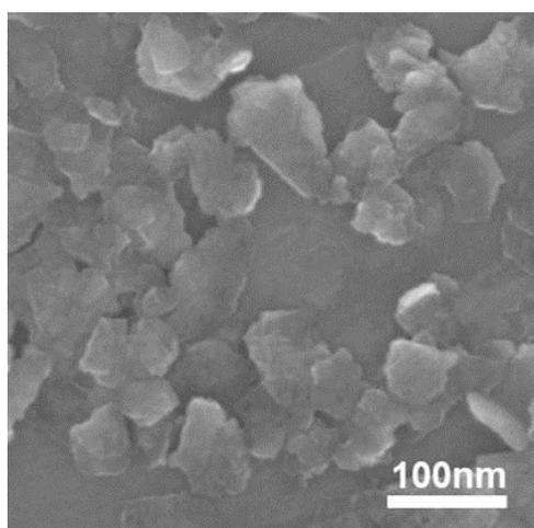
**Figure S1.** FE-SEM image of MoS<sub>2</sub>-PVP NSs.
