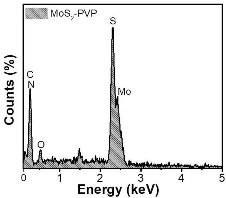
**Figure S4.** EDS spectrum of MoS<sub>2</sub>-PVP NSs.
