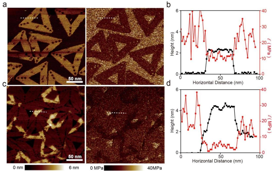
**Figure S2.** AFM PF-QNM images characterizing the mono- and bilayer triangular DNA origamis. (a) Height (nm) (left) and stiffness (MPa) (right) of the monolayer triangular DNA origamis. (b) Cross-sectional profiles of the height and DMT of monolayer DNA origamis. (c) Height (nm) (left) and stiffness (MPa) (right) of the bilayer triangular DNA origamis. (d) Cross-section profiles of height and  $E$  for the bilayer DNA origamis.
