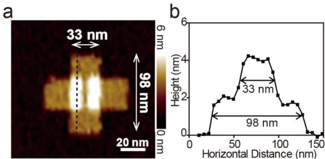
**Figure S1.** AFM PF-QNM images of the shape and dimensions of the cross-shaped DNA origami adsorbed onto the mica surface. (a) Topographic image. (b) Height profile (right) along the black line in (a).
