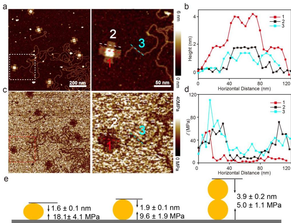
**Figure S5.** PF-QNM images of cross-shaped DNA origamis and lambda DNA showing the height and stiffness with a peak-force of 100 pN. (a) Topographical AFM images (left); enlarged image (right). (b) Height profile in (a, right) marked using colored lines. (c) DMT AFM images. (d) Young's modulus profile of the colored lines (c, right) showing the measured  $E$  of single DNA molecules, mono-, and
