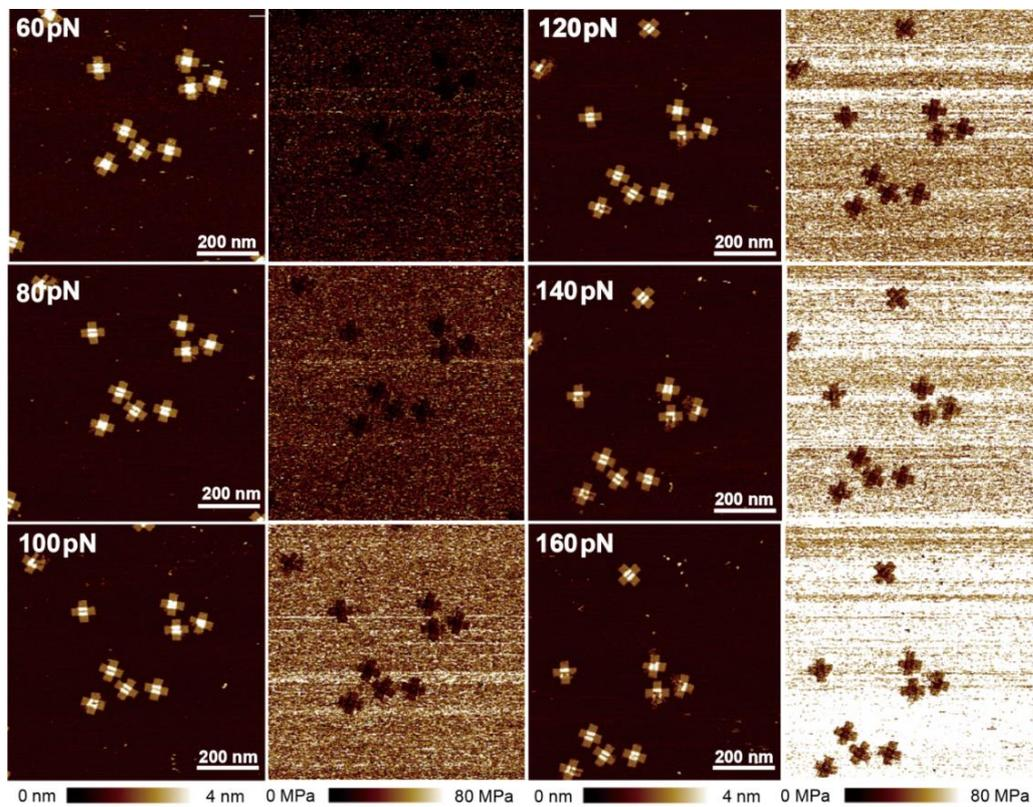
**Figure S3.** AFM PF-QNM images of cross-shaped DNA origamis at different peak-forces at a range of 60–160 pN. Images show the height (left) and stiffness (right) of DNA origamis.
