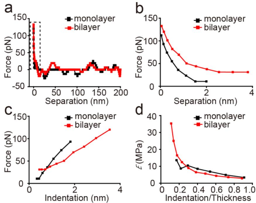
**Figure S4.** Reconstruction processes for the correction of Young's modulus (as described in Biophys. J. 2018, 114, 2923-29032). (a) Original approach curves of force-separation. (b) Enlarged figure marked by the rectangle in a. (c) Corresponding of the force-separation curve in b. (d) Corrected Young's modulus as a function of indentation.
