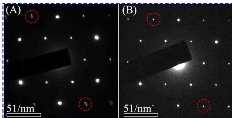
**Fig. S4** The SAED pattern of (A) M-Ti<sub>3</sub>C<sub>2</sub>T<sub>x</sub> and (B) U-Ti<sub>3</sub>C<sub>2</sub>T<sub>x</sub>.
