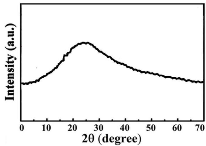
Fig. S7 XRD pattern of SiO<sub>2</sub> nanopowders.
