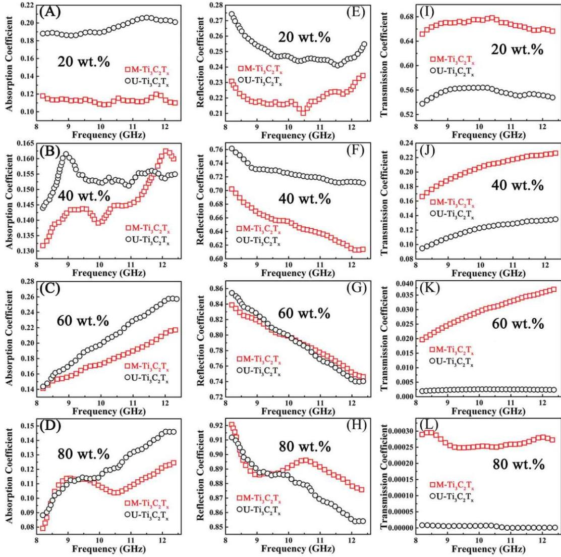
**Fig. S5** (A)-(D) Absorption comparison of the  $M\text{-Ti}_3\text{C}_2\text{T}_x$  and  $U\text{-Ti}_3\text{C}_2\text{T}_x$  at each mass ratio. (E)-(H) Reflection comparison of the  $M\text{-Ti}_3\text{C}_2\text{T}_x$  and  $U\text{-Ti}_3\text{C}_2\text{T}_x$  at each mass ratio. (I)-(L) Transmission comparison of the  $M\text{-Ti}_3\text{C}_2\text{T}_x$  and  $U\text{-Ti}_3\text{C}_2\text{T}_x$  at each mass ratio.
