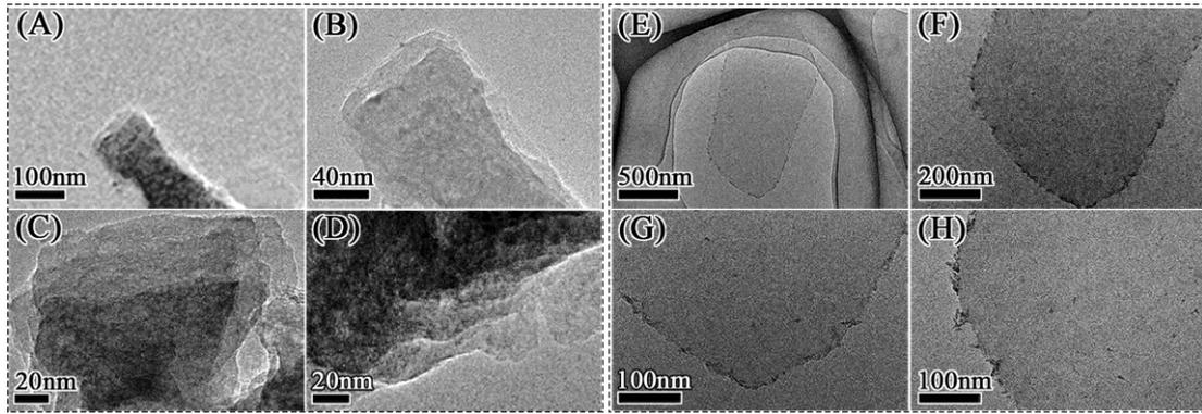
**Fig. S3** (A)-(D) TEM images of M-Ti<sub>3</sub>C<sub>2</sub>T<sub>x</sub>. (E)-(H) TEM images of U-Ti<sub>3</sub>C<sub>2</sub>T<sub>x</sub>.
