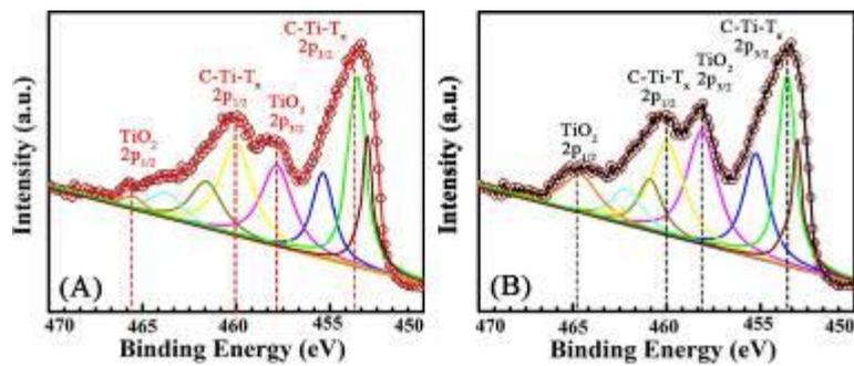
**Fig. S2** Curve fitting of XPS spectra for Ti 2p region in (A) M-Ti<sub>3</sub>C<sub>2</sub>T<sub>x</sub> and (B) U-Ti<sub>3</sub>C<sub>2</sub>T<sub>x</sub>.
