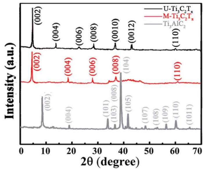
Fig. S1 XRD patterns of M- $\text{Ti}_3\text{C}_2\text{T}_x$  and U- $\text{Ti}_3\text{C}_2\text{T}_x$  and  $\text{Ti}_3\text{AlC}_2$ .
