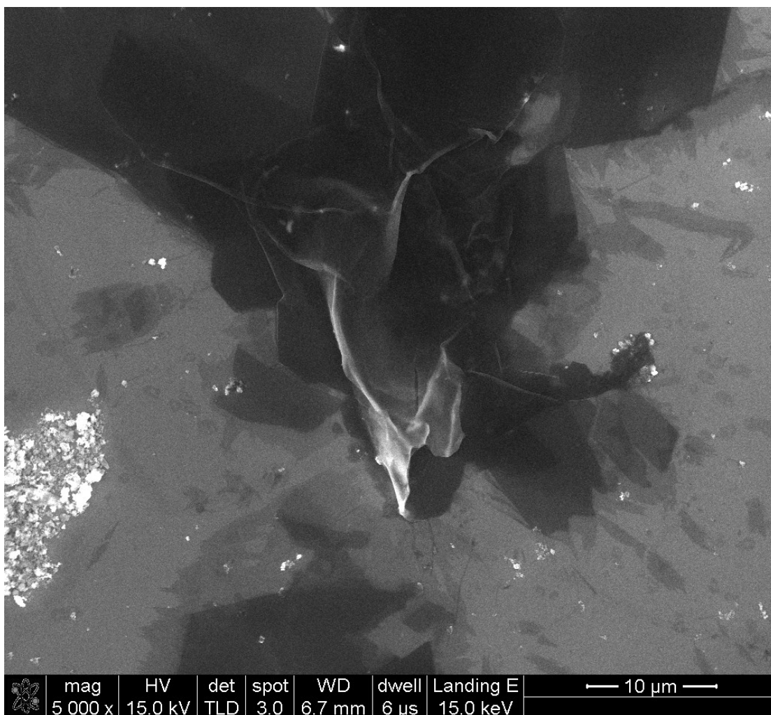
Fig. S4 SEM image of \text{Co}_{0.8}\text{Fe}_{0.2}\text{P} nanosheets at low magnification.
