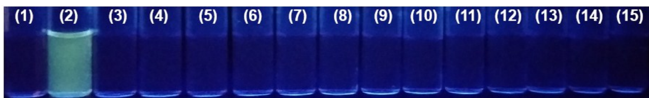
Fig. S8 Changes in fluorescence color of DNPH-NA (10 μM) in the presence of various ROS and anions (120 μM): (1) DNPH-NA only, (2) HOCl, (3) H 2 O 2 , (4) 1 O 2 , (5) ONOO - , (6) ·OH, (7) ·O 2 - , (8) NO 2 - , (9) NO 3 - , (10) PO 4 3- , (11) Pi, (12) SO 4 2- , (13) HCO 3 - , (14) Cl - , (15) F - .
