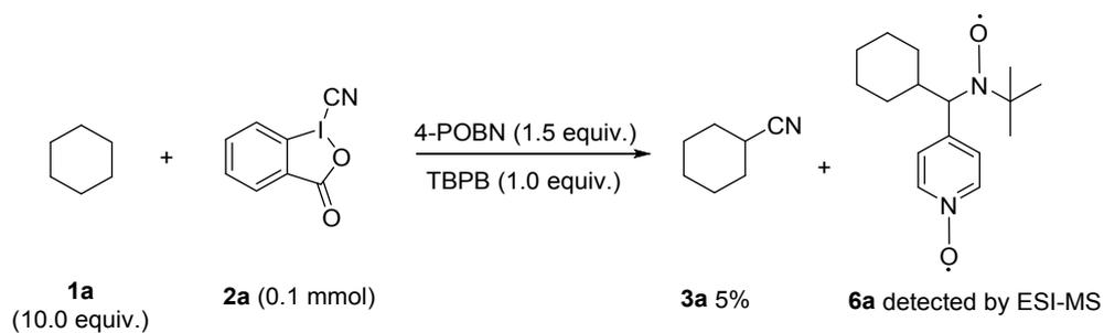
**Scheme S2.** Radical-trapping experiment of cyclohexane.
