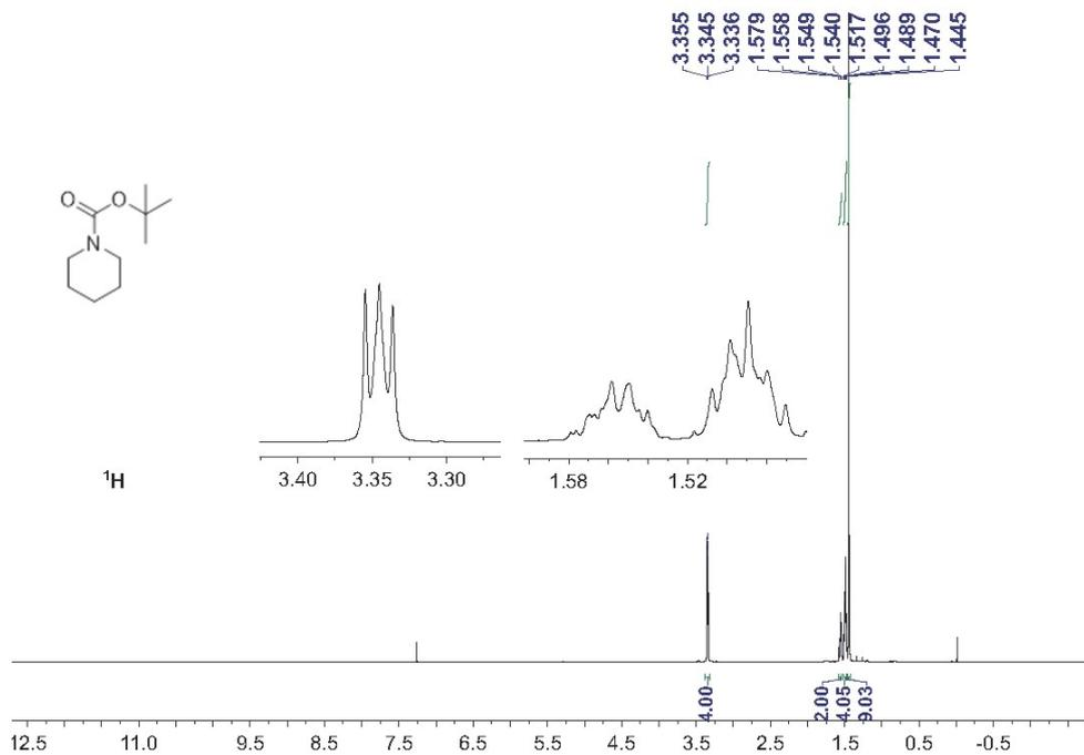
**<sup>1</sup>H NMR (600 MHz, CDCl<sub>3</sub>, 298 K) of 4k**
