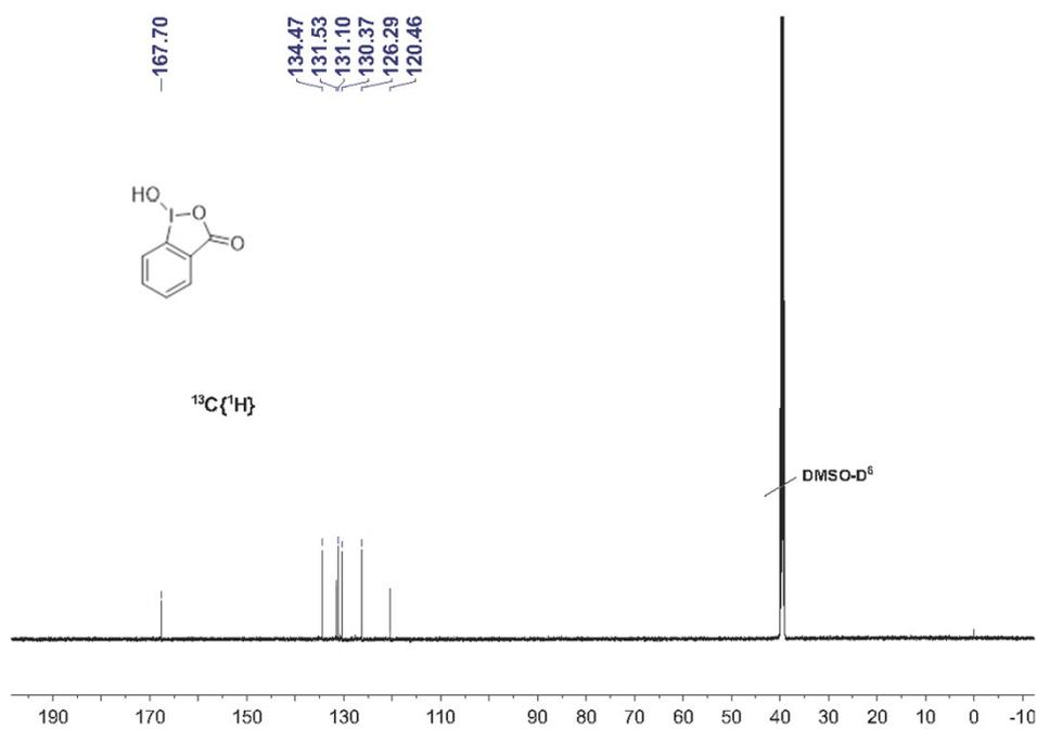
$^{13}\text{C}\{^1\text{H}\}$  (600 MHz, DMSO- $\text{D}_6$ , 298 K) of **2aa**
