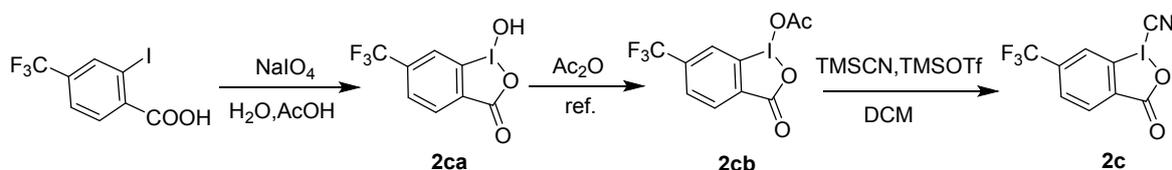
**Scheme S7.** The procedures for the synthesis of **2c**.
