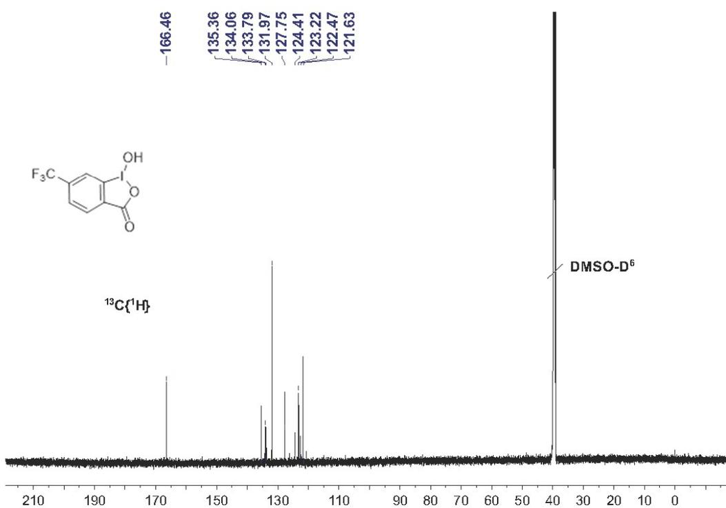
$^{13}\text{C}\{^1\text{H}\}$  (600 MHz,  $\text{DMSO-D}_6$ , 298 K) of **2ca**
