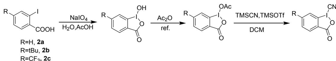
**Scheme S5.** The procedures for the synthesis of cyanation-transfer reagents.
