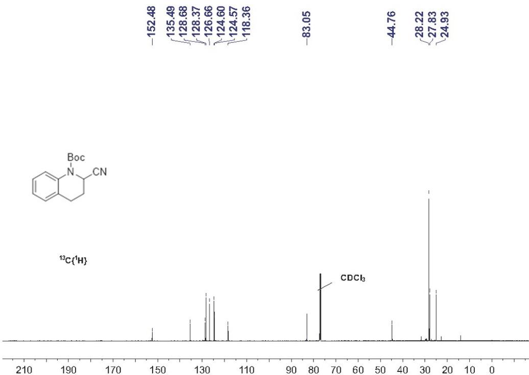
**<sup>13</sup>C{<sup>1</sup>H} (600 MHz, CDCl<sub>3</sub>, 298 K) of 5I**
