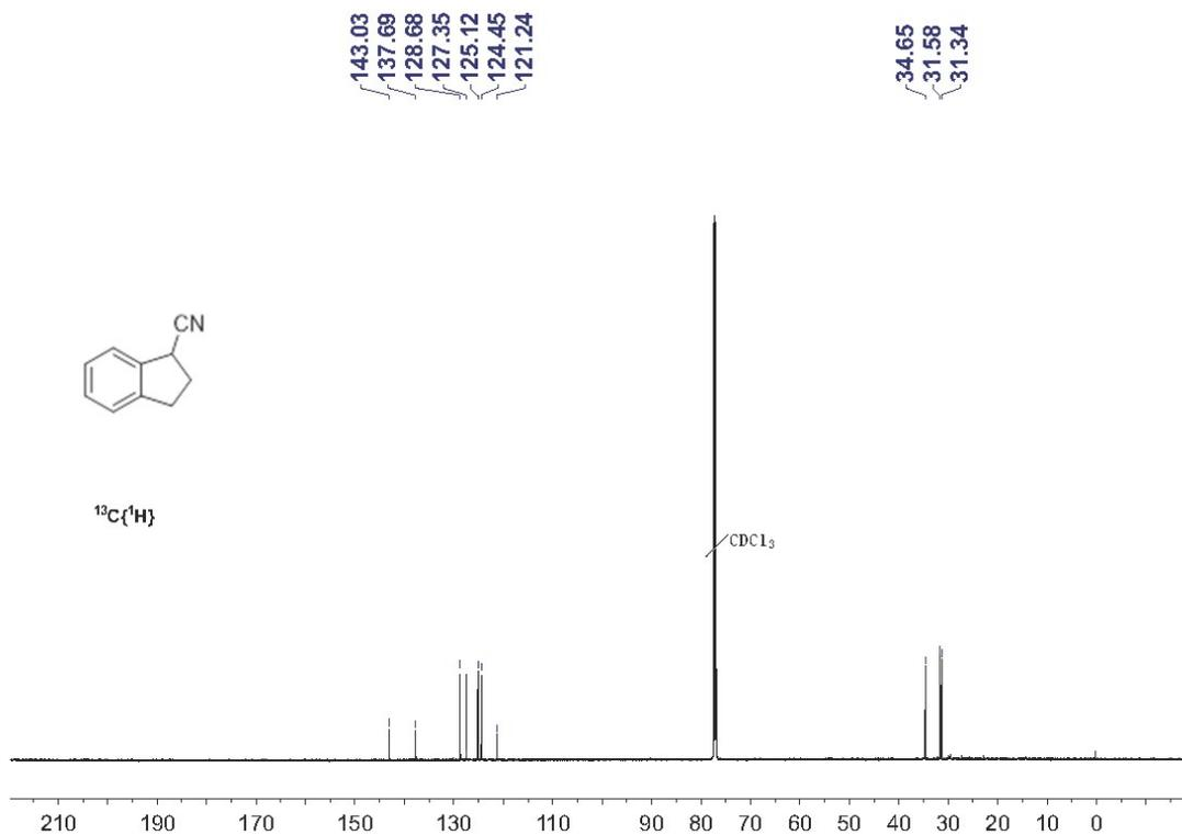
**<sup>13</sup>C{<sup>1</sup>H} (600 MHz, CDCl<sub>3</sub>, 298 K) of 3d**
