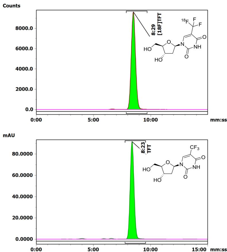
**Figure S3.** Radio-HPLC chromatogram of [<sup>18</sup>F]TFT (retention time 8:29 minutes:seconds) and the corresponding UV profile, after semi-preparative HPLC purification (UV signal is detected earlier than the radio-signal due to the distance between the two detectors). Column: Luna® C18, 4.6 × 150 mm, 5 μM (Phenomenex, UK). Isocratic method 2: eluant A H<sub>2</sub>O, 90%; eluant B CH<sub>3</sub>CN, 10%; flow rate 1 mL/min.
