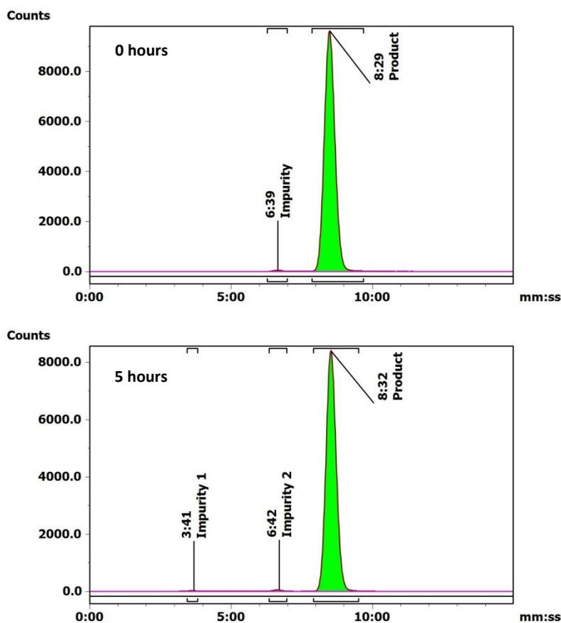
**Figure S5.** Radio-HPLC chromatograms representing  $[^{18}\text{F}]\text{TFT}$  stability after 0 and 5 hours in  $\text{H}_2\text{O}$  at ambient temperature. HPLC details: Luna<sup>®</sup> C18 column,  $4.6 \times 150$  mm,  $5 \mu\text{M}$  (Phenomenex, UK). Isocratic method 2: Eluant A  $\text{H}_2\text{O}$ , 90%; eluant B  $\text{CH}_3\text{CN}$ , 10%; flow rate 1 mL/min.
