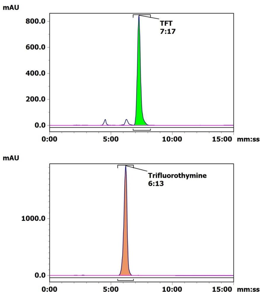
**Figure S6.** HPLC chromatograms showing the UV absorbance signals of the parent compound TFT 5 (retention time 7:17 minute:seconds) and the expected metabolite trifluorothymine (retention time 6:13 minute:seconds). HPLC details:  $\mu$ Bondapak C18 column, 7.8  $\times$  300 mm, 10  $\mu$ m, 125  $\text{\AA}$  (Waters, UK) and isocratic method 4: eluant A  $H_2O$ , 90%; eluant B EtOH, 10%; 3 mL/min flow rate.
