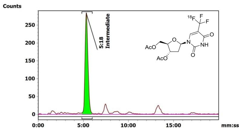
**Figure S2.** Radio-HPLC chromatogram of the radiolabelled intermediate [ $^{18}\text{F}$ ]-4 (retention time 5:18 minutes:seconds, purified using a Sep-pak SPE HLB cartridge only). Column: Luna<sup>®</sup> C18, 4.6 × 150 mm, 5 μM (Phenomenex, UK). Isocratic method 1: eluant A H<sub>2</sub>O, 65%; eluant B CH<sub>3</sub>CN, 35%; flow rate 1 mL/min.
