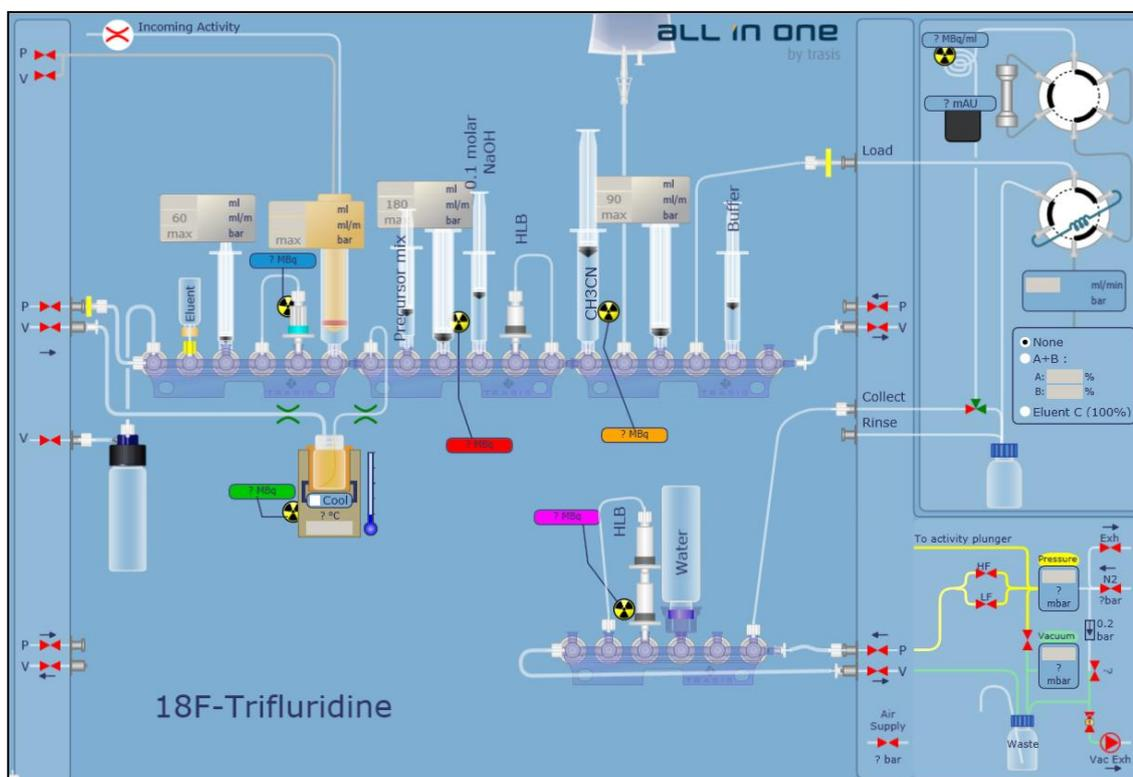
**Figure S1.** Trasis AllInOne automated synthesis cassette setup for the automatic preparation of [ $^{18}\text{F}$ ]TFT.
