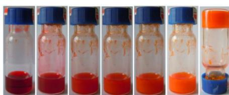
Figure S2 Photographs of TCbzB in o -dichlorobenzene/cyclohexane ( v/v = 1/2 ) during the formation of orange organogel under daylight.
