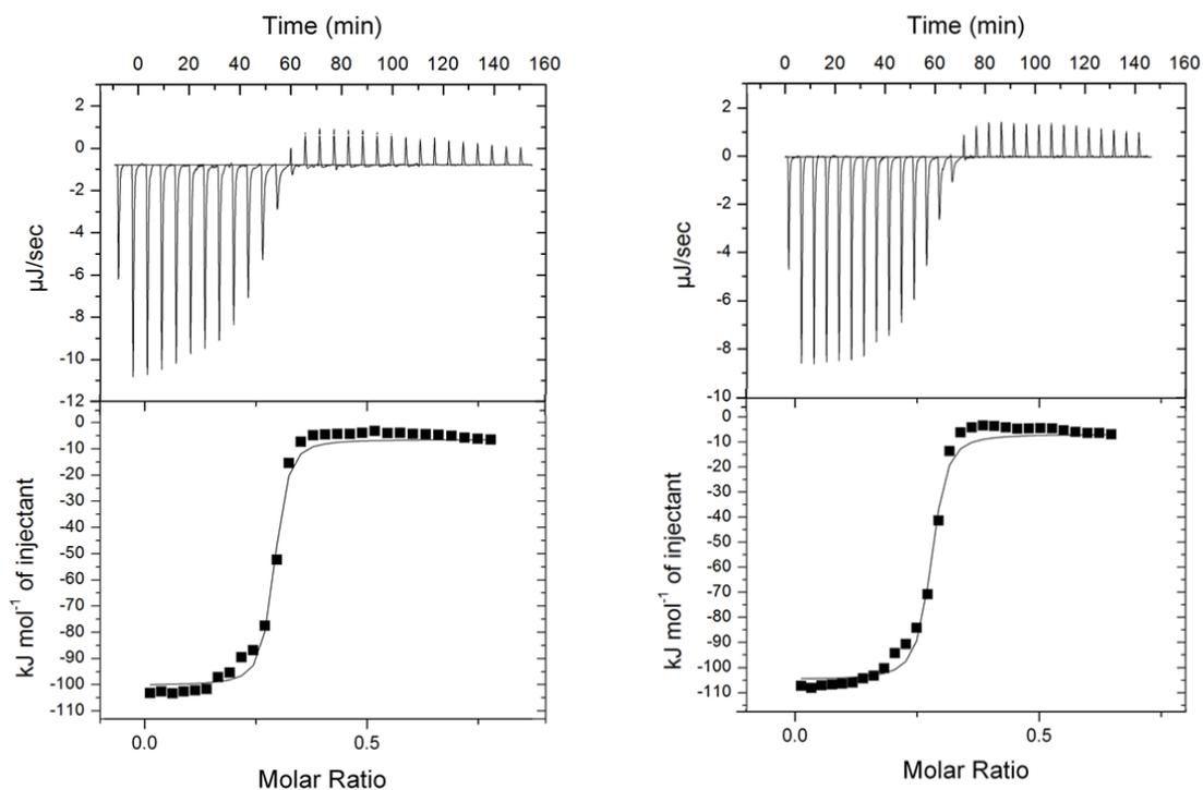
**Figure S1.** Raw ITC data (top) obtained by injections of glycocluster **4b**: TPE-(EG<sub>3</sub>-Gal)<sub>4</sub> (0.36 mM for the left panel and 0.30 mM for the right panel) to a solution of LecA (0.1 mM) and the corresponding integrated titration curve (bottom)
