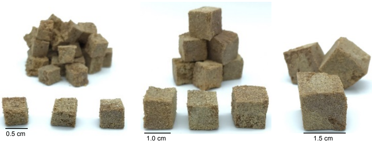
0.5 cm, 1.0 cm and 1.5 cm cubes of sulfur polymer composite containing 70% NPK fertiliser
