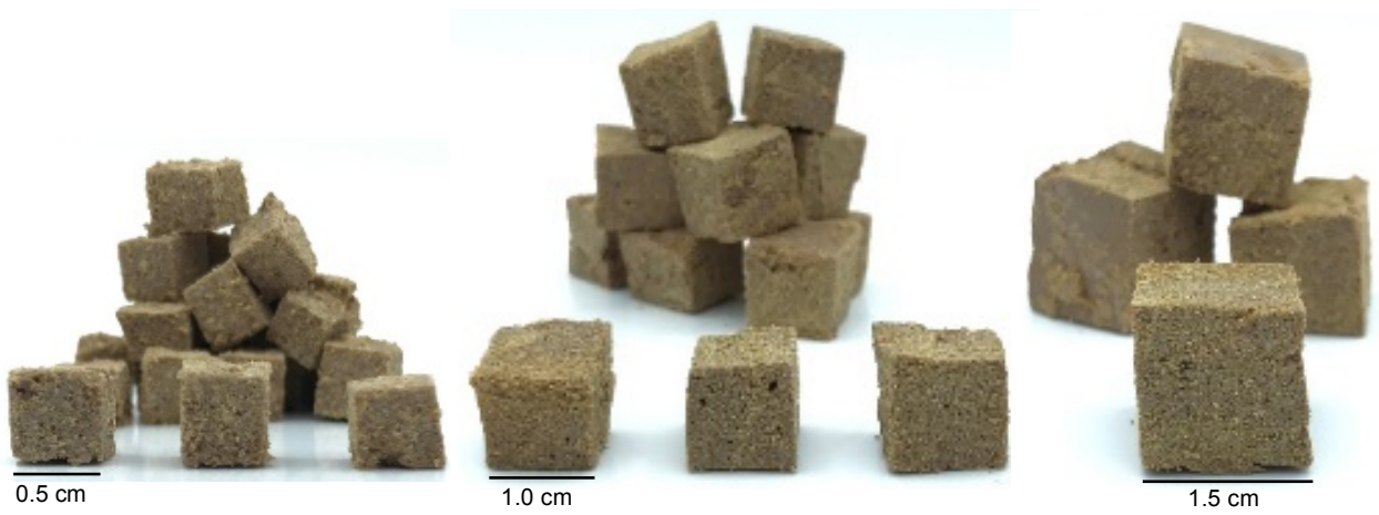
0.5 cm, 1.0 cm and 1.5 cm cubes of sulfur polymer composite containing 60% NPK fertiliser
