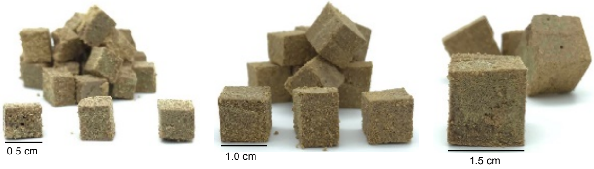
0.5 cm, 1.0 cm and 1.5 cm cubes of sulfur polymer composite containing 50% NPK fertiliser
