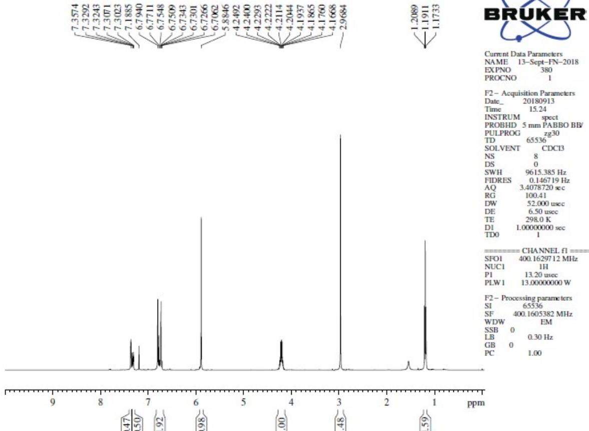
Figure 45: <sup>1</sup>H NMR spectrum of 3w
