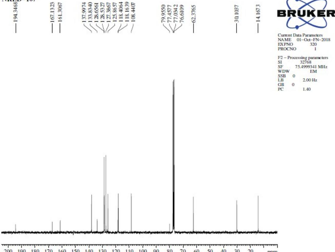
Figure 2:  $^{13}\text{C}$  NMR spectrum of 3a
