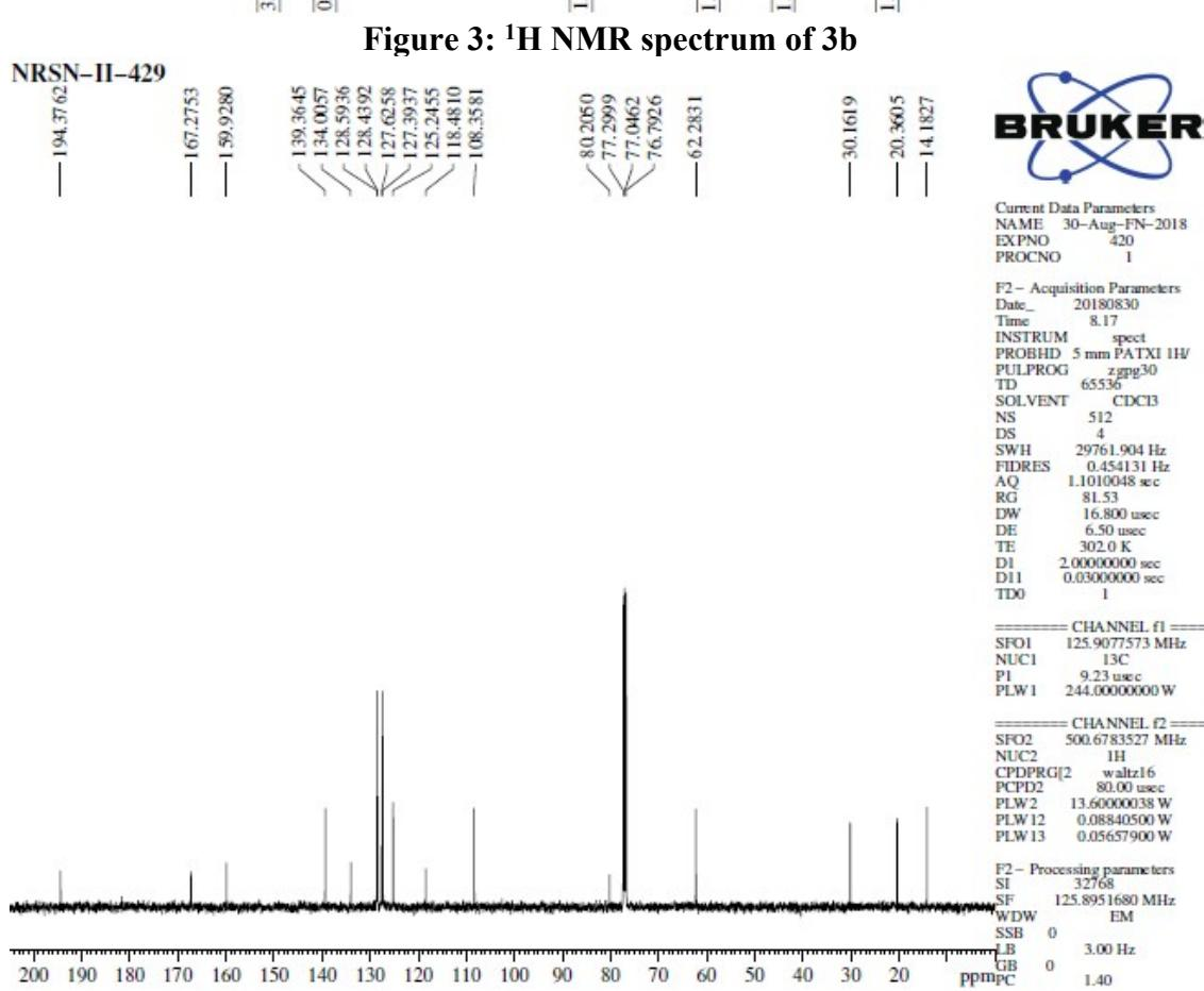
**Figure 4:**  $^{13}\text{C}$  NMR spectrum of 3b
