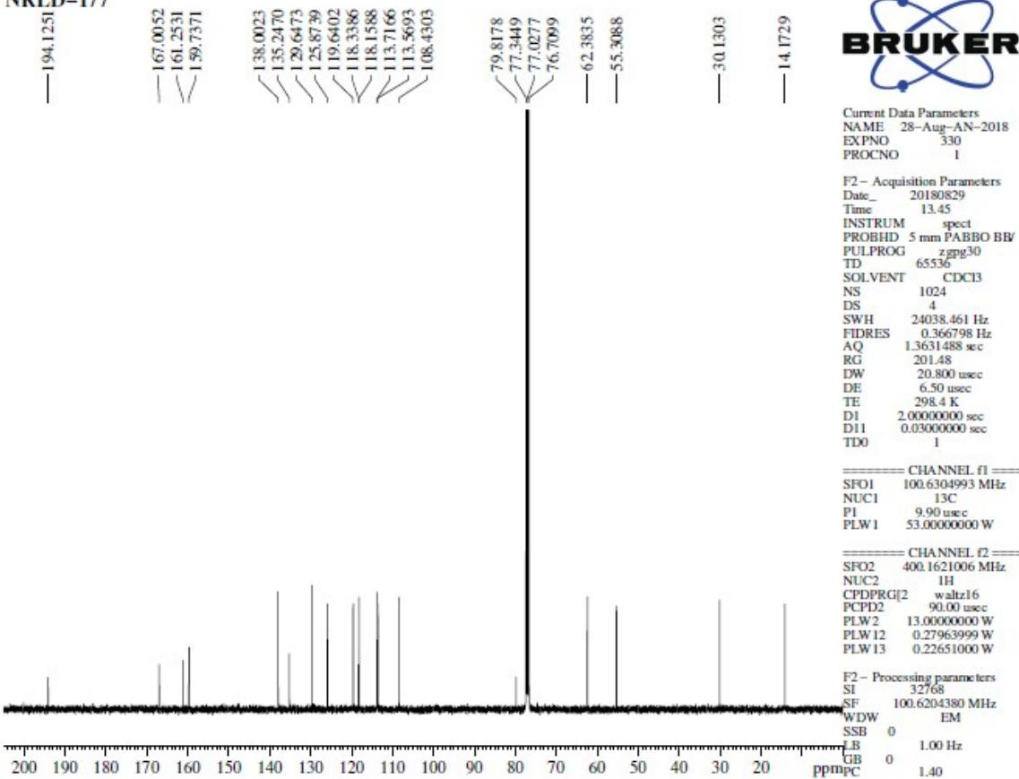
Figure 24: <sup>13</sup>C NMR spectrum of 3l
