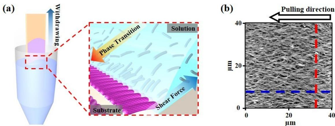
Figure S2 (a) Schematic illustration of self-templating process and (b) the AFM analysis well demonstrate the unidirectionally aligned WHW-phage matrices.
