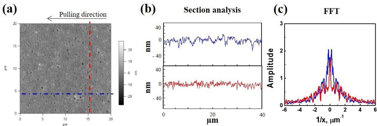
**Figure S4** (a) AFM image of self-assembled nanostructure consisted of wild-type phage. (b) The height profile analysis and (c) fast fourier transform analysis reveals planar structure due to the lack of self-assembly time.
