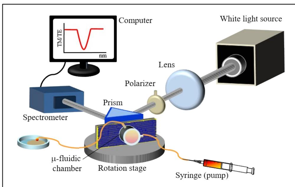
Figure S1 Schematic illustration of experimental set-up for WHW-phage-based SPR sensor.
