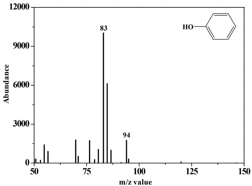
**Figure S9.** GC-MS spectrum showing m/z value 94 that corresponds to molecular ion peak of phenol.
