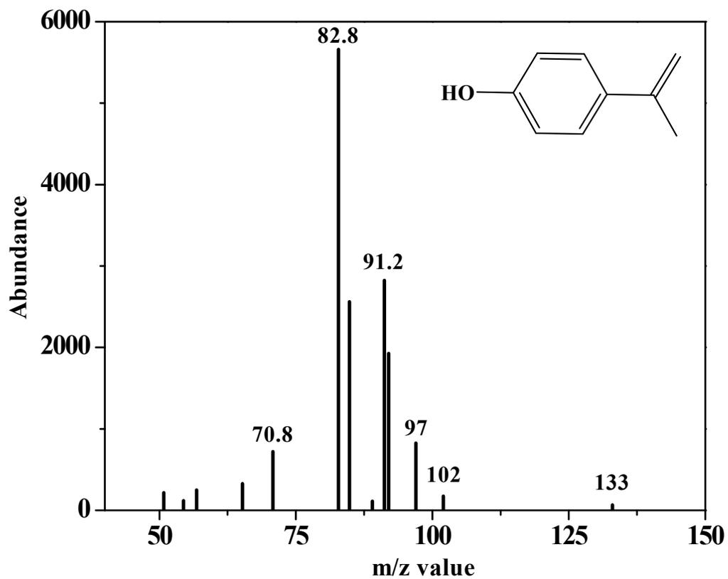
**Figure S7.** GC-MS spectrum showing m/z value 133 that corresponds to molecular ion peak of 4-(prop-1-en-2-yl)phenol.
