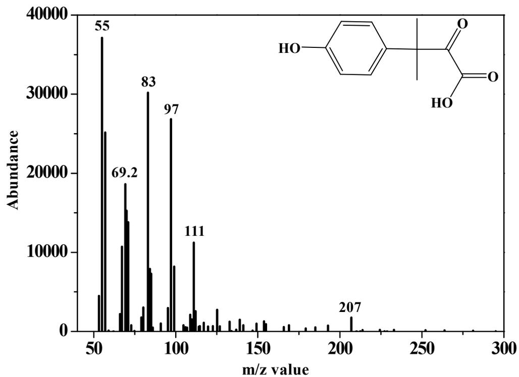
**Figure S5.** GC-MS spectrum showing m/z value 207 that corresponds to molecular ion peak of 3-(4-hydroxyphenyl)-3-methyl-2-oxobutanoic acid.
