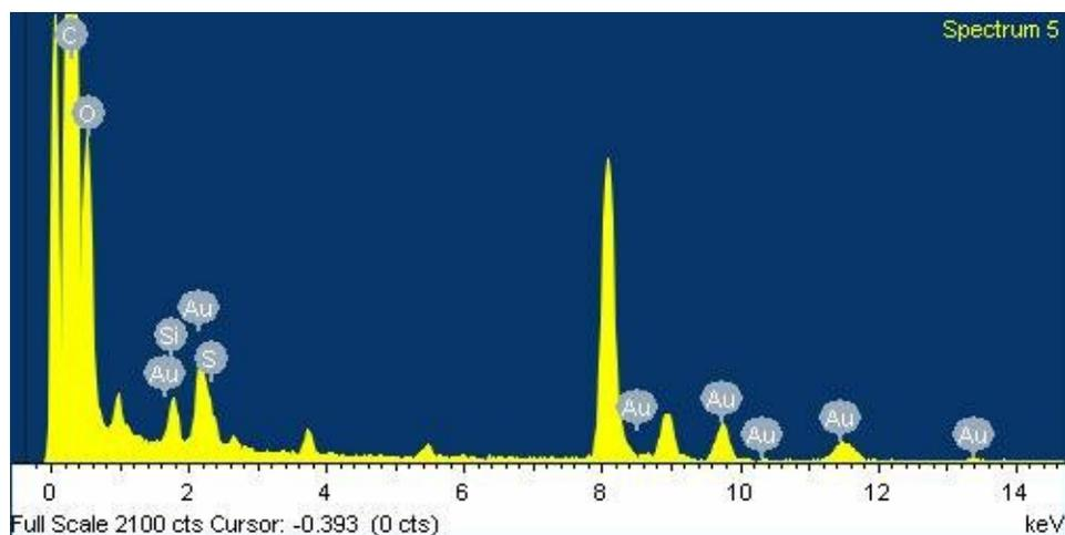
**Figure S2.** EDX of rGO/Au nanocomposite showing the presence of gold, silicon, sulphur and other elements.
