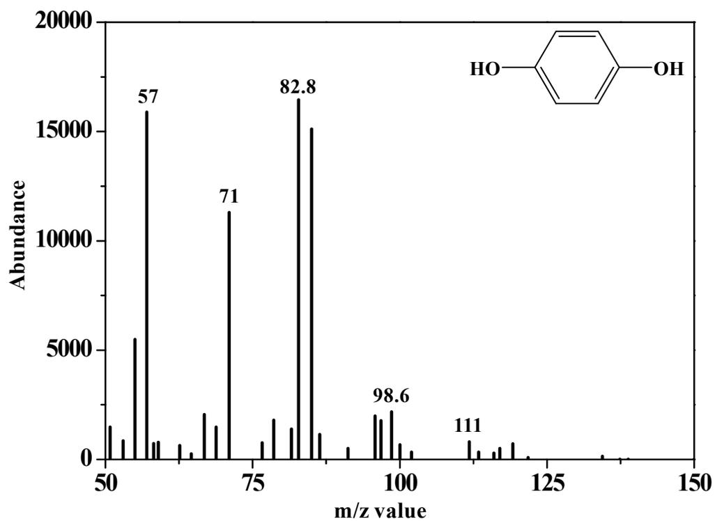
**Figure S10.** GC-MS spectrum showing m/z value 111 that corresponds to molecular ion peak of hydroquinone.
