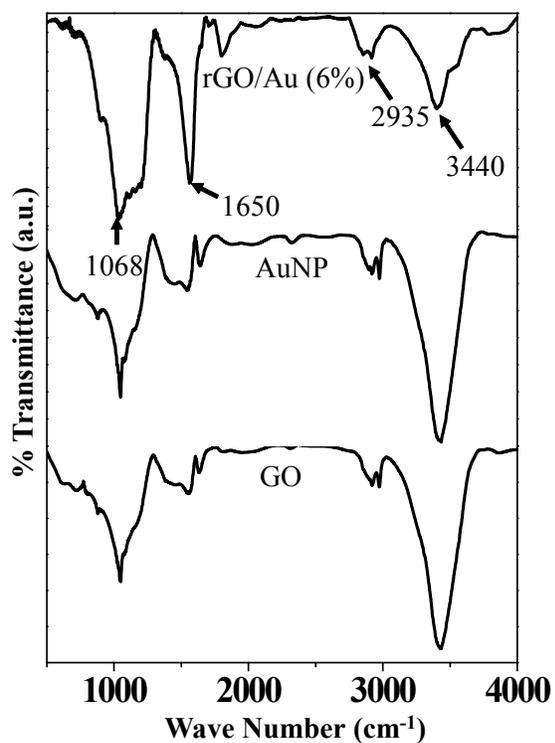
**Figure S3.** FTIR data of GO, silica coated Au and rGO/Au (6 %) nanocomposite. rGO/Au shows N-H vibration band at  $\sim 1650$  cm<sup>-1</sup> similar to silica coated Au nanoparticle and O-H vibration band at  $\sim 3440$  cm<sup>-1</sup> similar to GO.
