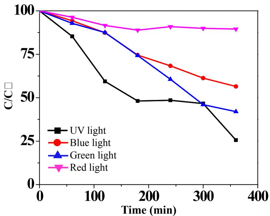
**Figure S12.** Light wavelength dependent photocatalytic degradation kinetics of bisphenol A by rGO/Au (6%) that is shown in Figure S11. Samples are collected at different times light irradiation and absorbance ratio of final to initial ( $C/C_0$ ) is measured at 278 nm.
