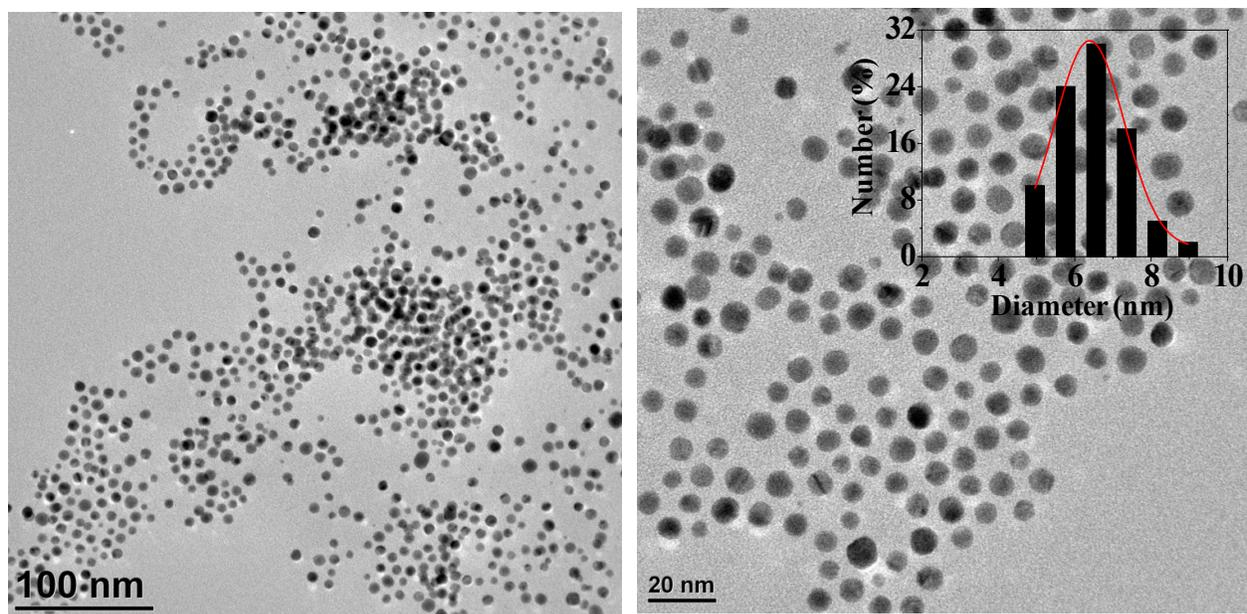
**Figure S1.** TEM image of silica coated Au nanoparticle at two different magnifications. Silica shell is too thin ( $< 5$  nm) to observe under TEM. Inset shows the particle size distribution with the average size on 7 nm.
