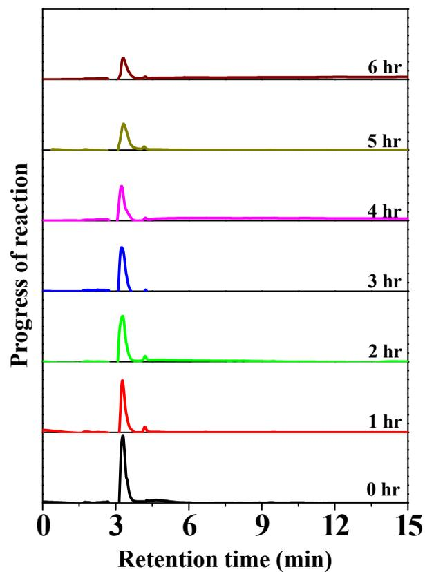
**Figure S4.** Monitoring of bisphenol A degradation by HPLC using UV-visible detector. Samples are collected at different times of visible light irradiation and detected at 280 nm. Here the photodegradation is studied in completely alcohol free condition.
