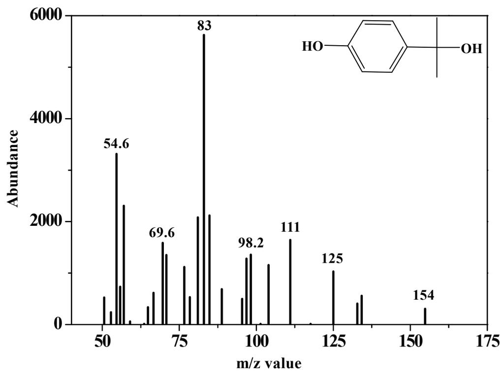
**Figure S6.** GC-MS spectrum showing m/z value 154 that corresponds to molecular ion peak of 4-(2-hydroxypropan-2-yl)phenol.
