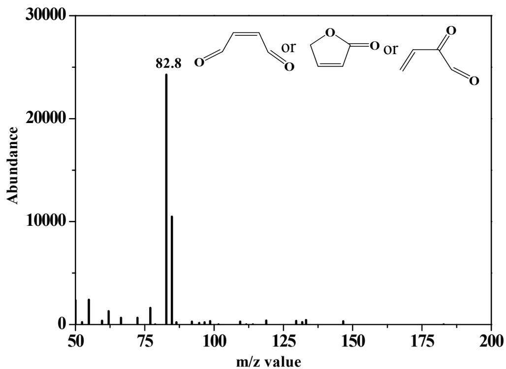
**Figure S8.** GC-MS spectrum showing m/z value 83 that corresponds to molecular ion peak of aliphatic ketone/aldehyde.
