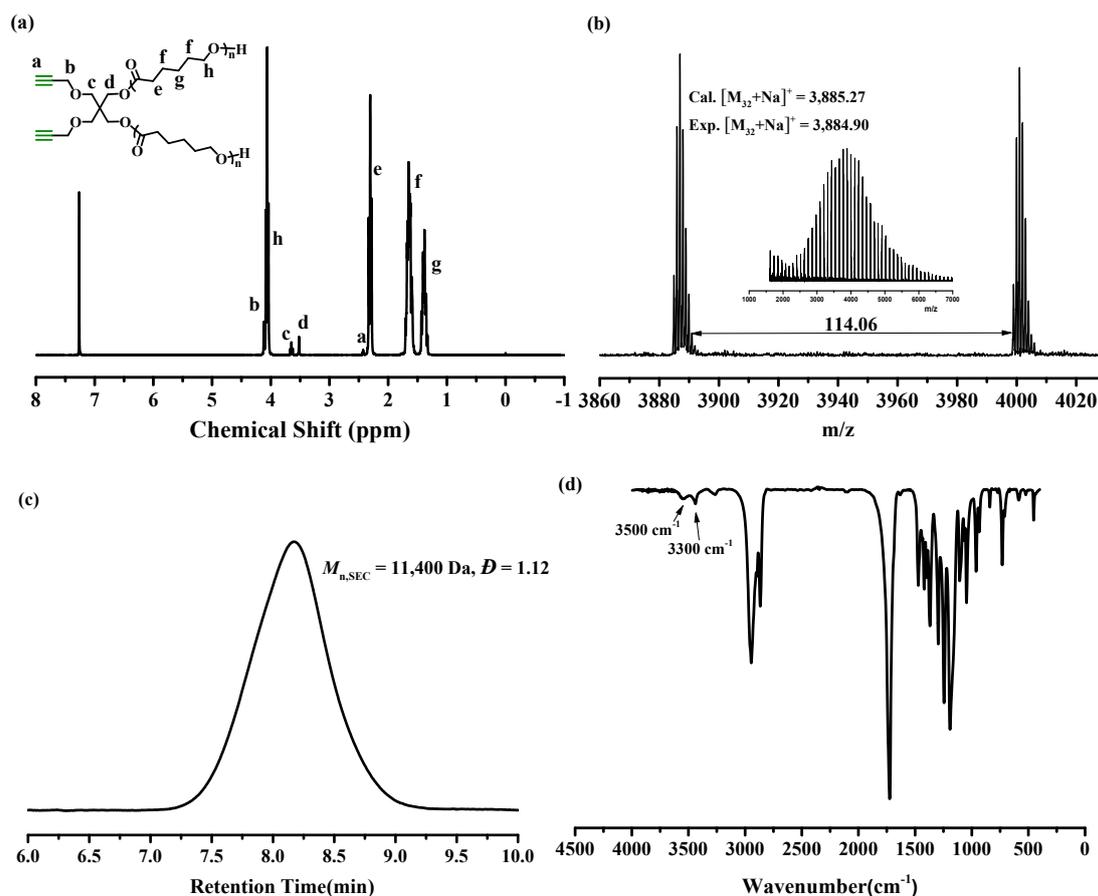
Figure S1. Structural characterizations of 2alkynyl-*l*-PCL-2OH: (a) <sup>1</sup>H NMR spectrum in CDCl<sub>3</sub>, (b) MALDI-TOF mass spectrum, (c) SEC trace, and (d) FT-IR spectrum.
