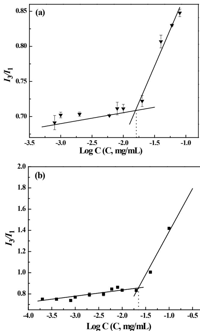
Figure S2. Intensity ratios ( $I_3/I_1$ ) in fluorescence emission spectra of pyrene as a function of the logarithm concentrations of (a) PEG-*b*-(*c*-PCL)-*b*-PEG and (b) PEG-*b*-(*l*-PCL)-*b*-PEG.
