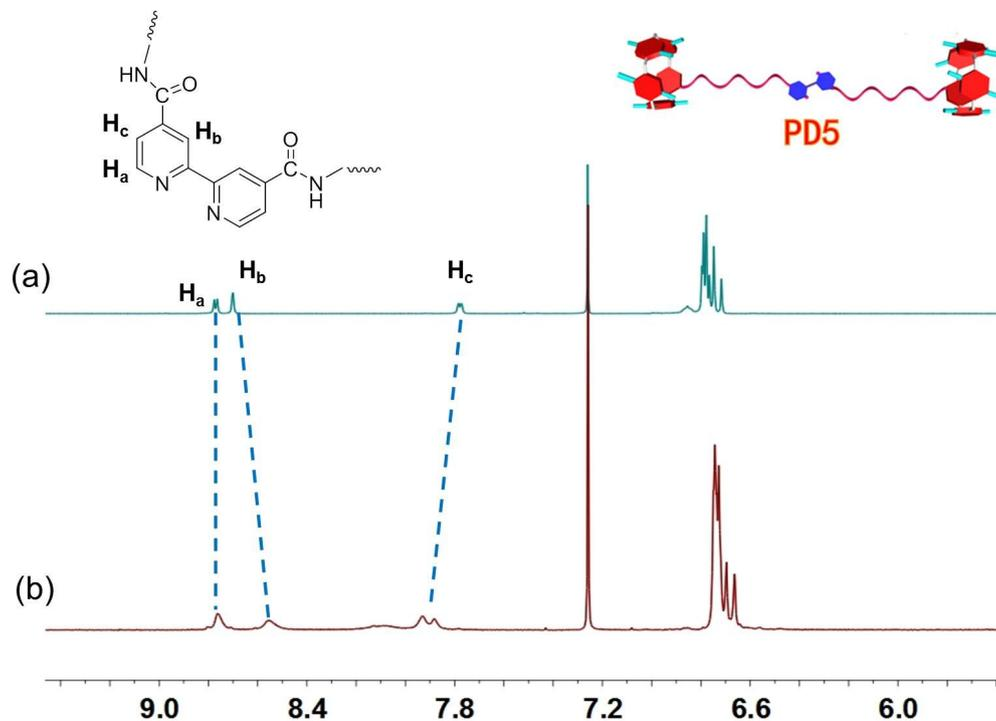
**Figure S17** Partial  $^1\text{H}$  NMR spectra (400 MHz,  $\text{CDCl}_3$ , 298 K) of 5.00 mM **PD5** in the absence (a) and presence (b) of 0.33 equiv. of  $\text{Zn}(\text{NTf}_2)_2$ .
