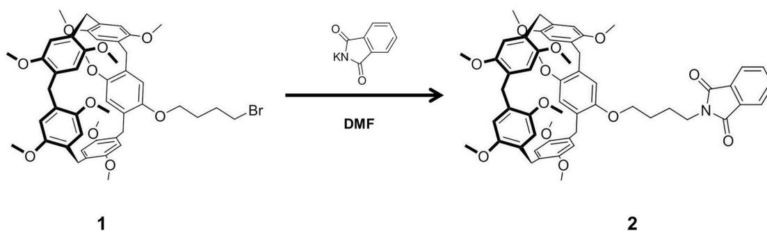
Compound **2**: A mixture of **1** (2.00 g, 2.20 mmol) and potassium phthalimide (1.00 g, 5.00 mmol) was stirred in N, N-dimethylformamide at 90 °C for 24 h. The solution
