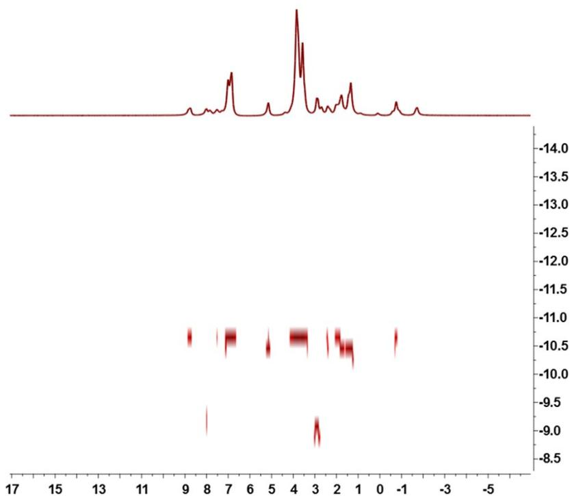
**Figure S15** DOSY NMR spectrum (500 MHz, CDCl<sub>3</sub>, 298 K) of **PD5** and **G** at 100 mM.
