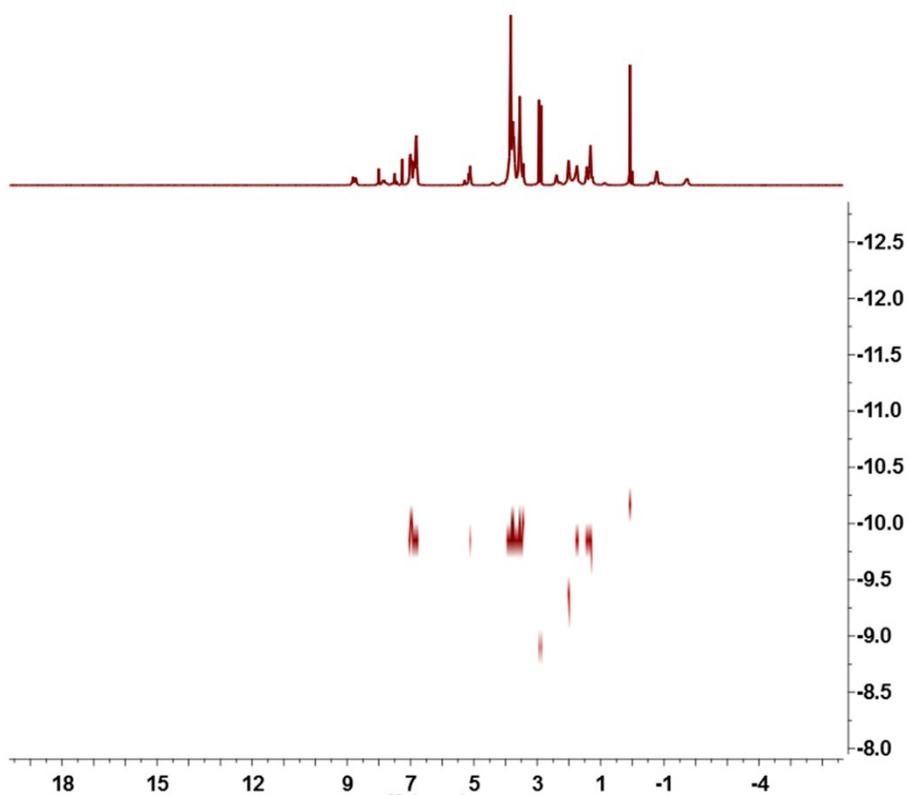
**Figure S12.** DOSY NMR spectrum (500 MHz, CDCl<sub>3</sub>, 298 K) of **PD5** and **G** at 30.0 mM.
