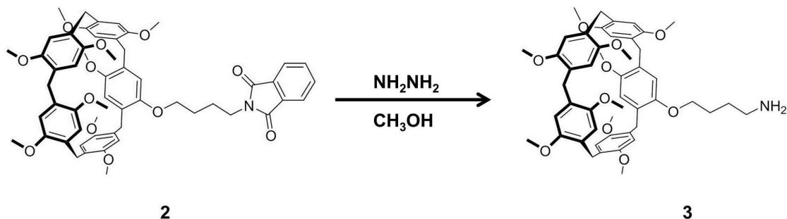
Compound **3**: A mixture of **2** (1.00 g, 1.06 mmol) and  $\text{NH}_2\text{NH}_2$  (10 mL) was heated at reflux in methanol (20 mL) for 12 h. Then the mixture was filtered and the residue was washed with methanol (10 mL  $\times$  2) to give **3** as a white solid (0.51 g, 60%), mp: 144.4–145.1  $^\circ\text{C}$ . The  $^1\text{H}$  NMR spectrum of compound **3** is shown in Figure S4.  $^1\text{H}$
