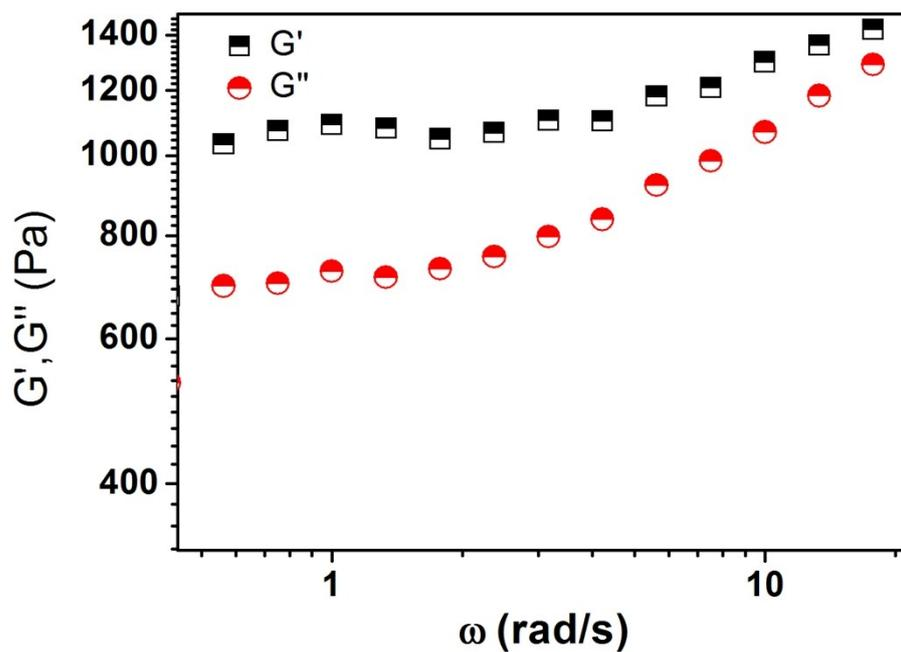
Figure S20 Frequency dependency of the storage modulus  $G'$  and loss modulus  $G''$  of the gel.
