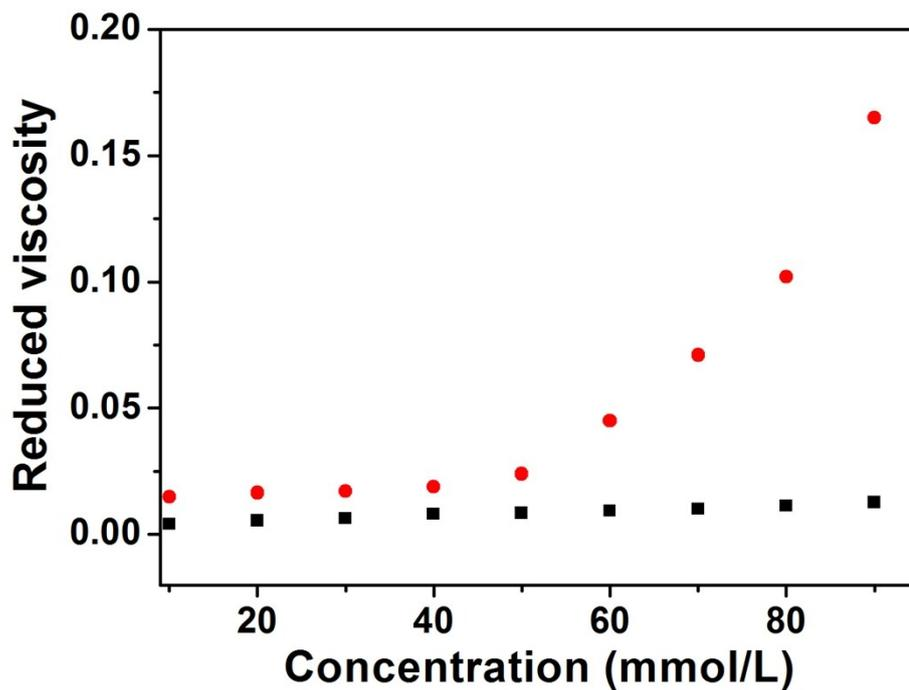
Figure S19 Reduced viscosity (chloroform 298 K) of a 1:1 molar mixture of PD5 and G (■) and 1:3:3 molar mixture of Zn<sup>2+</sup>, PD5 and G (●).
