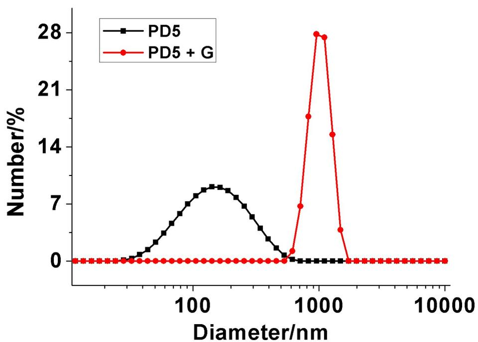
**Figure S16** Size distributions of **PD5** and **PD5 + G** ( $c = 55.0$  mM).
