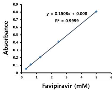
**Supplement Fig. 5.** Calibration curve of absorbance of Favipiravir at 360 nm.
