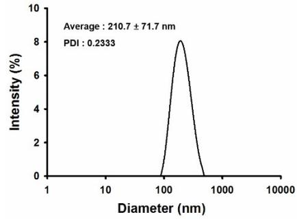
**Supplement Fig. 6.** DLS analysis of dual drug-loaded 80 w.t.% PBASomes..(Favipiravir and mir-323a)
