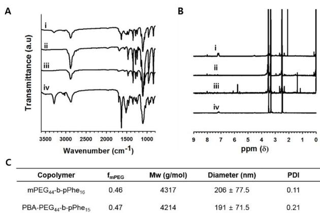
**Supplement Fig. 2.** Polymer characterization. A) FT-IR and B)  $^1H$  NMR spectrum of (i) PBA-PEG<sub>44</sub>-b-pPhe<sub>15</sub> ( $f_{mPEG} = 0.47$ ), (ii) NH<sub>2</sub>-PEG<sub>44</sub>-PBA, (iii) tBOC-PEG<sub>44</sub>-PBA and (iv) mPEG<sub>44</sub>-b-pPhe<sub>16</sub> ( $f_{mPEG} = 0.46$ ). C) characterization table of mPEG<sub>44</sub>-b-pPhe<sub>16</sub> and PBA-PEG<sub>44</sub>-b-pPhe<sub>15</sub>.
