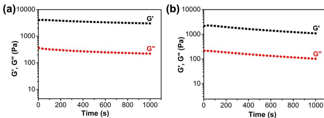
**Figure S7.** The rheological measurement of fluorescent hydrogels obtained from HA-ALD biopolymers, prepared from 4 hours reaction time (a) and 5 hours reaction time (b).
