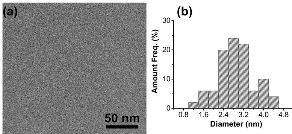
**Figure S1.** (a) The typical TEM image for the CDs. (b) The corresponding size of the CDs.
