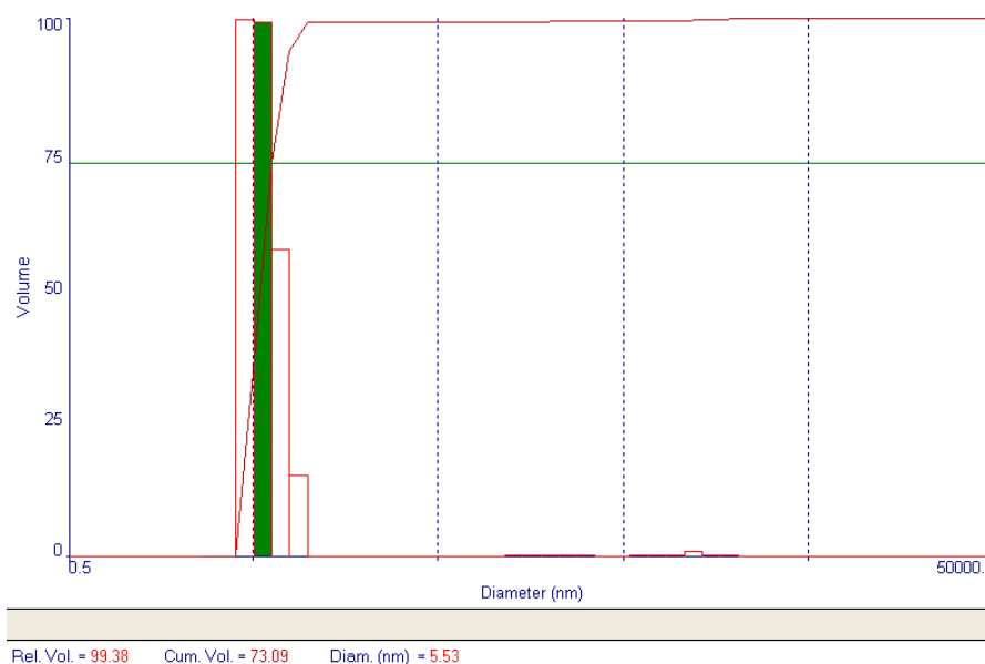
Figure S7. DLS analysis of LDP- G_{3Gly}F measured with a DLS laser of \lambda_{DLS} = 633 \text{ nm} in 0.1 M PB (pH 7.4) revealed a hydrodynamic molecular diameter of 5.53 nm. In case of the LDPs of BODIPY, PBI, and rhodamine the wavelength of the DLS laser interfered with the fluorescence of the conjugated fluorophore. Therefore, representative LDP- G_{3Gly}F serves as an example for the entire LDP series.
