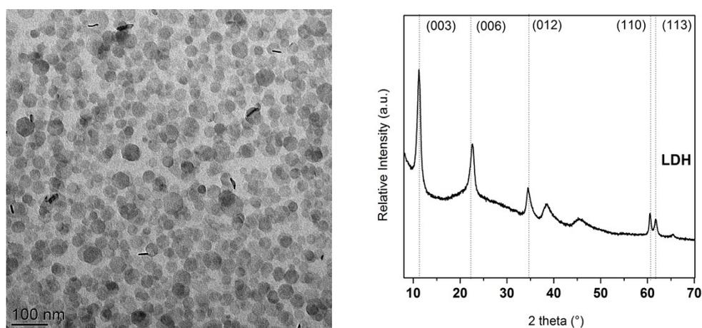
**Figure S1:** TEM image (left) and PXRD pattern (right) of Mg<sub>3</sub>Al-CO<sub>3</sub> nanoparticles.
