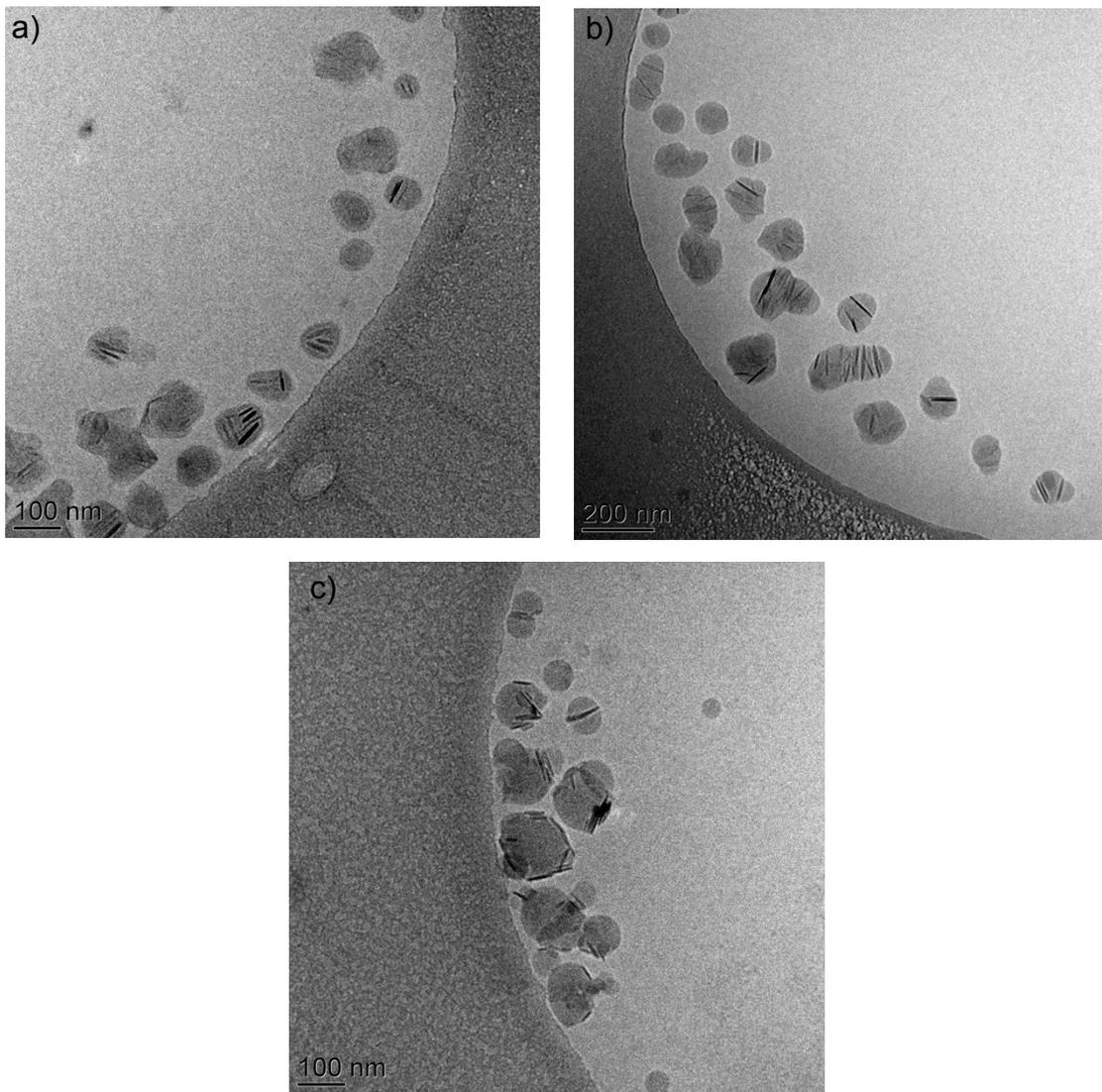
**Figure S2:** Cryo-TEM images of the latexes obtained using a)  $P(AA-BA)_{15}$ -R to give encapsulated, b)  $P(AA-BA)_{35}$ -R to give dumbbell, and c)  $P(AA-BA)_{35}$  to give armoured particles.
