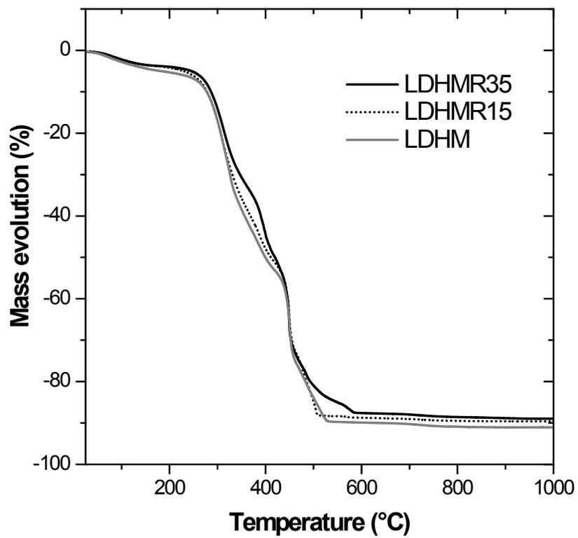
**Figure S3:** TGA curves of the different LDH nanocomposite films studied.
