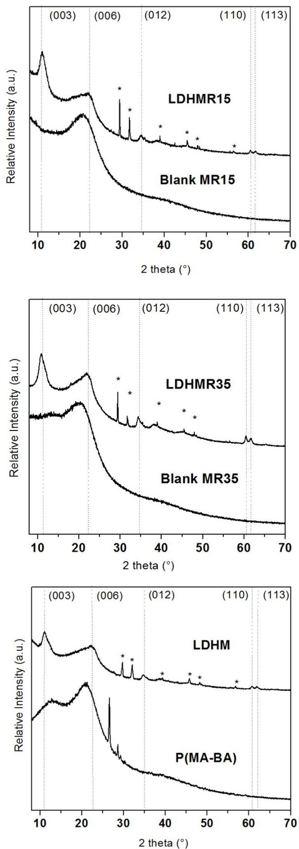
**Figure S4:** PXRD patterns of the different LDH nanocomposite films studied and of the corresponding blank matrices
