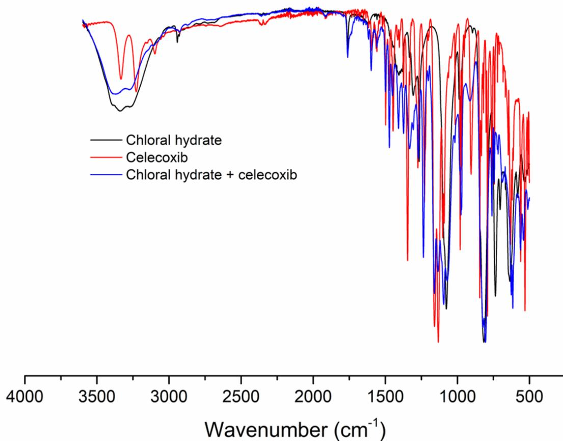
Figure S49. Comparison of FT-IR spectra of chloral hydrate, celecoxib and the corresponding mixture. Note that the carbonyl peak at 1762 cm<sup>-1</sup> is broadened in the mixture compared to chloral, which indicates some degree of interaction between the chloral and celecoxib.
