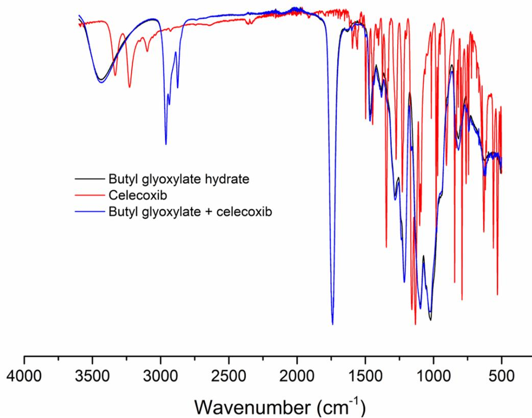
Figure S48. Comparison of FT-IR spectra of butyl glyoxylate hydrate, celecoxib and the corresponding mixture.
