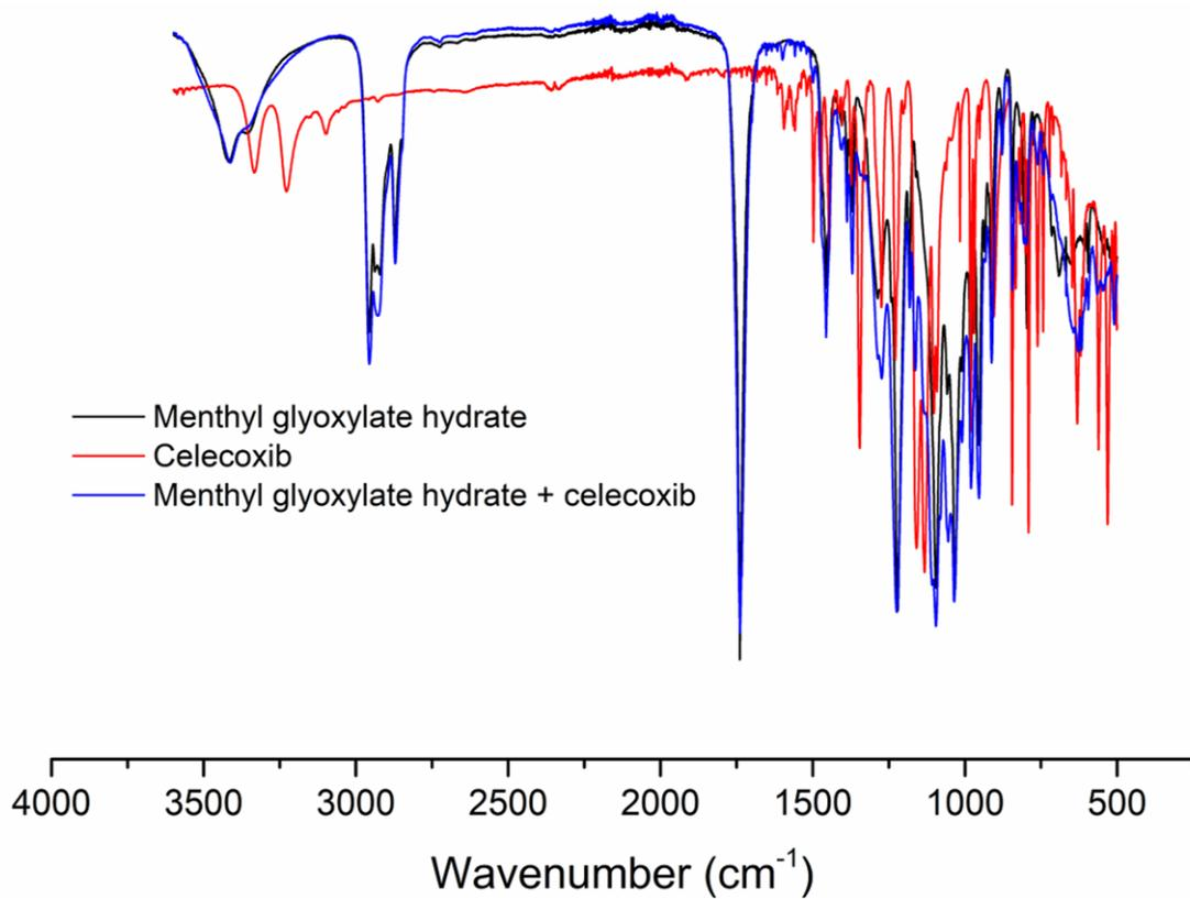
Figure S51. Comparison of FT-IR spectra of menthol glyoxylate hydrate, celecoxib and the corresponding mixture.
