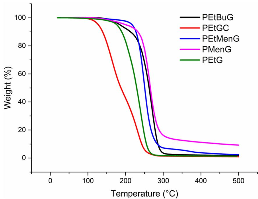
Figure S17. TGA curves of the polymers.
