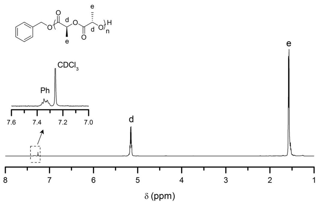
Figure S8. Representative <sup>1</sup>H NMR spectrum of PLLA. Deuterated chloroform was used as solvent.
