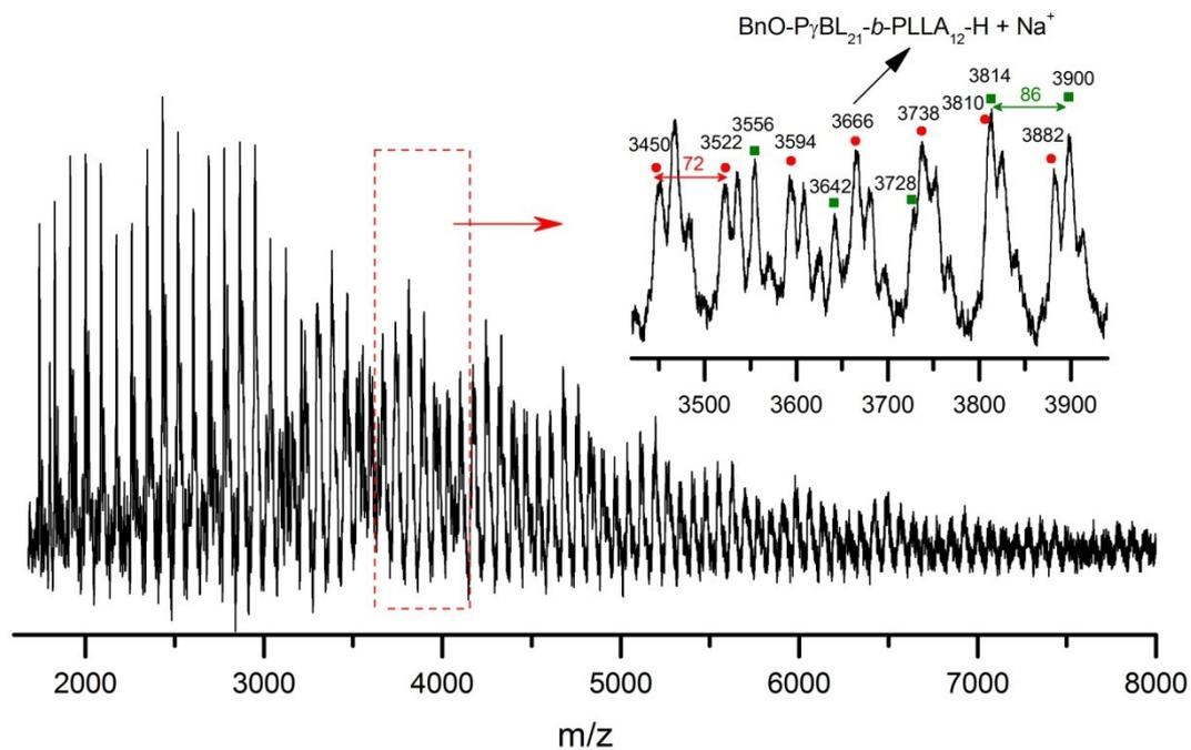
Figure S12. MALDI-TOF spectrum of PyBL-*b*-PLLA (Table 1, run 15). One possible structure for peak 3666 is  $BnO-PyBL_{21}-b-PLLA_{12}-H + Na^+$ .
