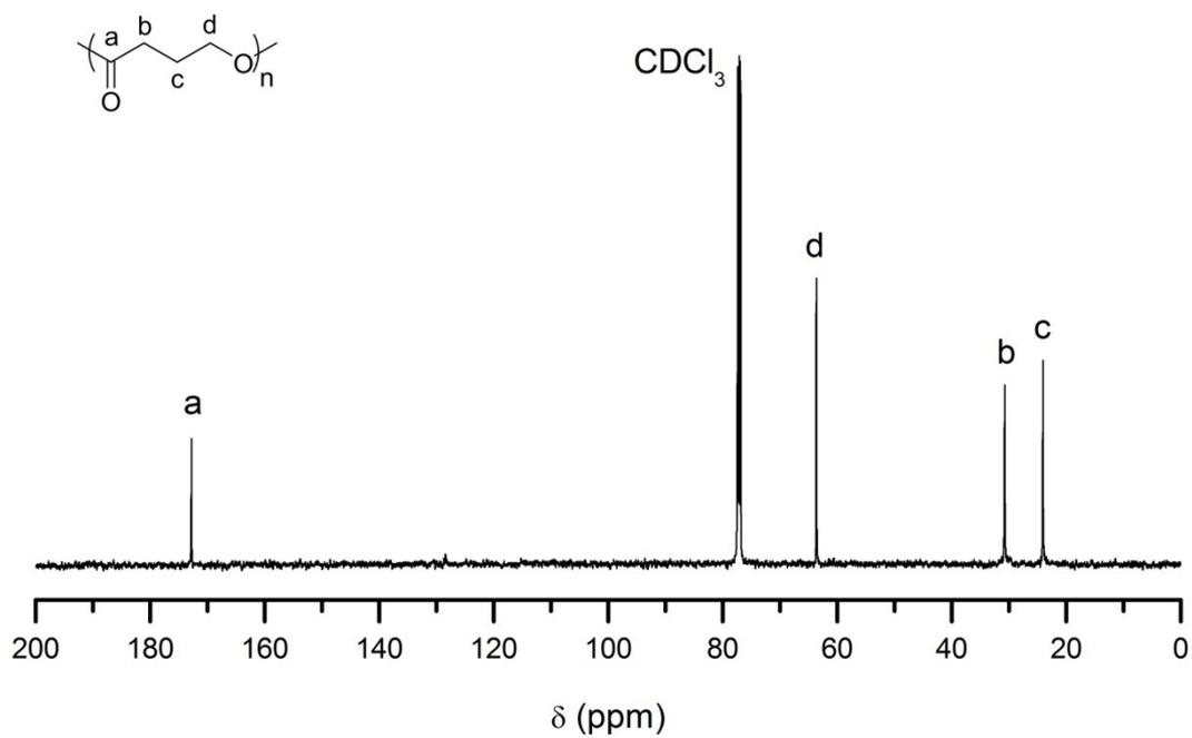
Figure S10. Representative  $^{13}\text{C}$  NMR spectrum of PyBL. Deuterated chloroform was used as solvent.
