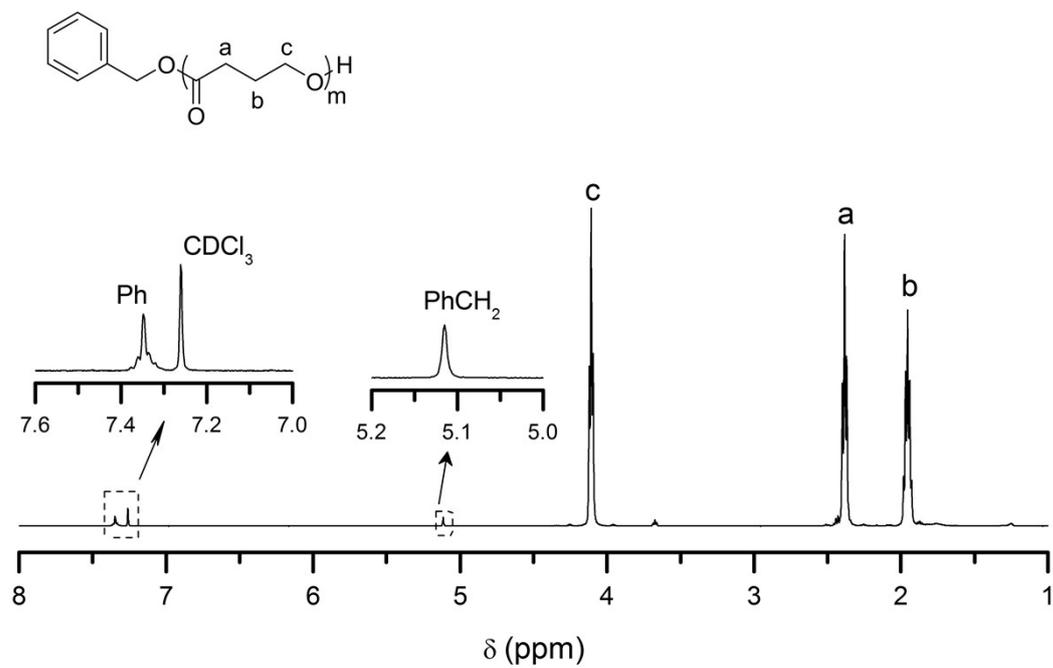
Figure S7. Representative <sup>1</sup>H NMR spectrum of PyBL. Deuterated chloroform was used as solvent.
