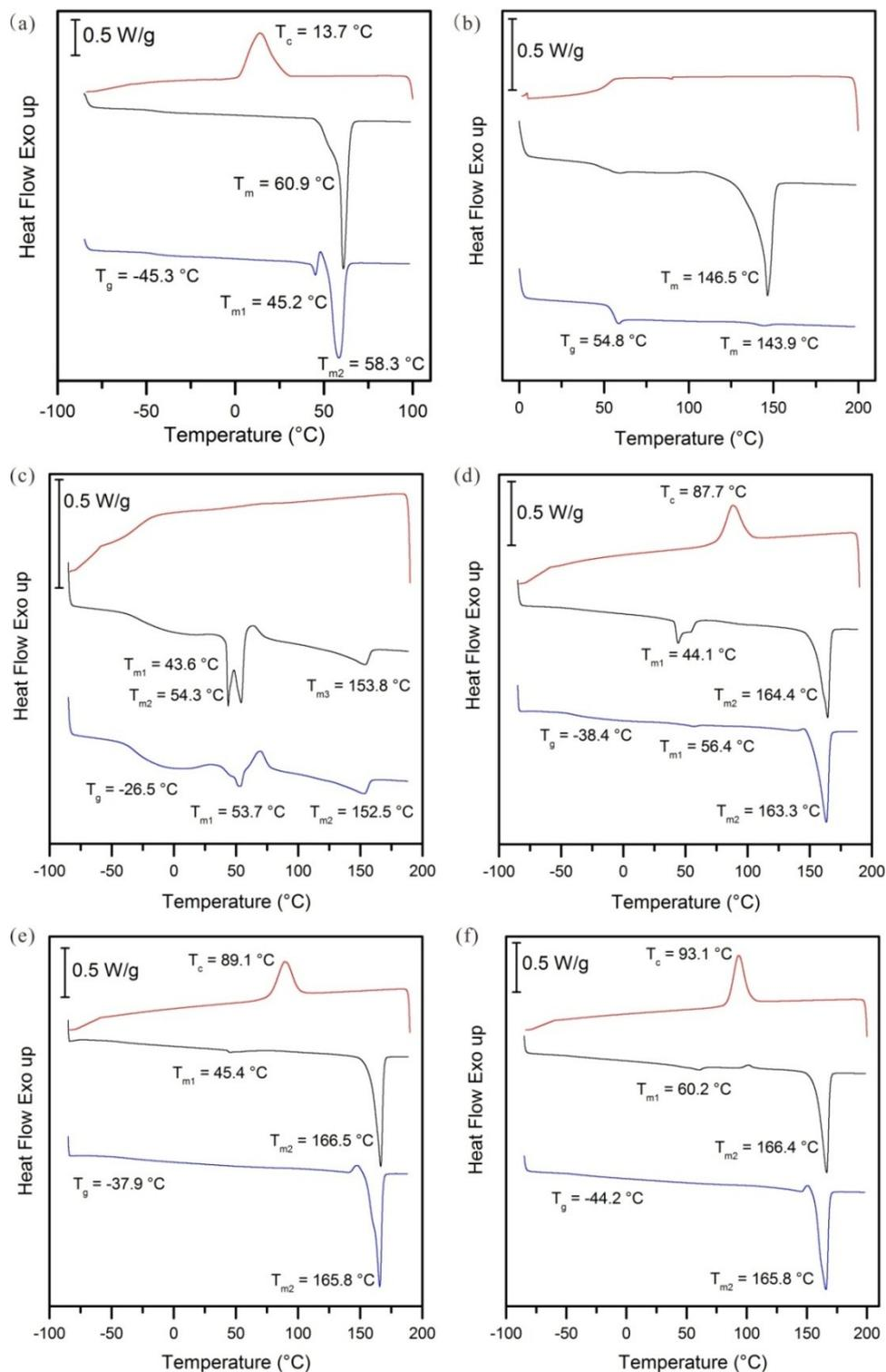
Figure S14. DSC curves (black lines: first heating scans; red lines: cooling scans; blue lines: second heating scans) of (a) PyBL (Table 1, run 7), (b) PLLA (Table S1, run 2), (c) PyBL<sub>50</sub>-b-PLLA<sub>29</sub> (Table 1, run 10), (d) PyBL<sub>44</sub>-b-PLLA<sub>49</sub> (Table 1, run 11), (e) PyBL<sub>50</sub>-b-PLLA<sub>77</sub> (Table 1, run 12) and (f) PyBL<sub>53</sub>-b-PLLA<sub>97</sub> (Table 1, run 9).
