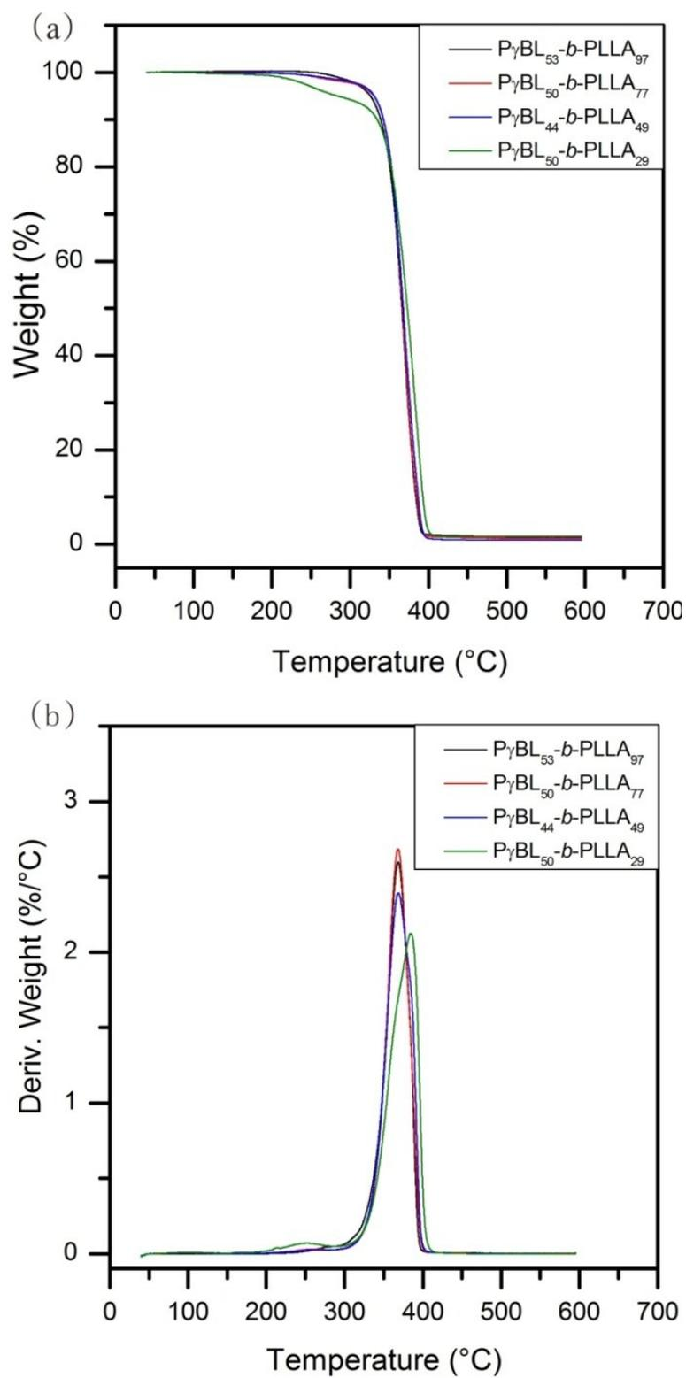
Figure S13. Representative (a) TGA and (b) DTG curves of  $P\gamma BL_x-b-PLLA_y$ . The samples used were the same with Table S4.
