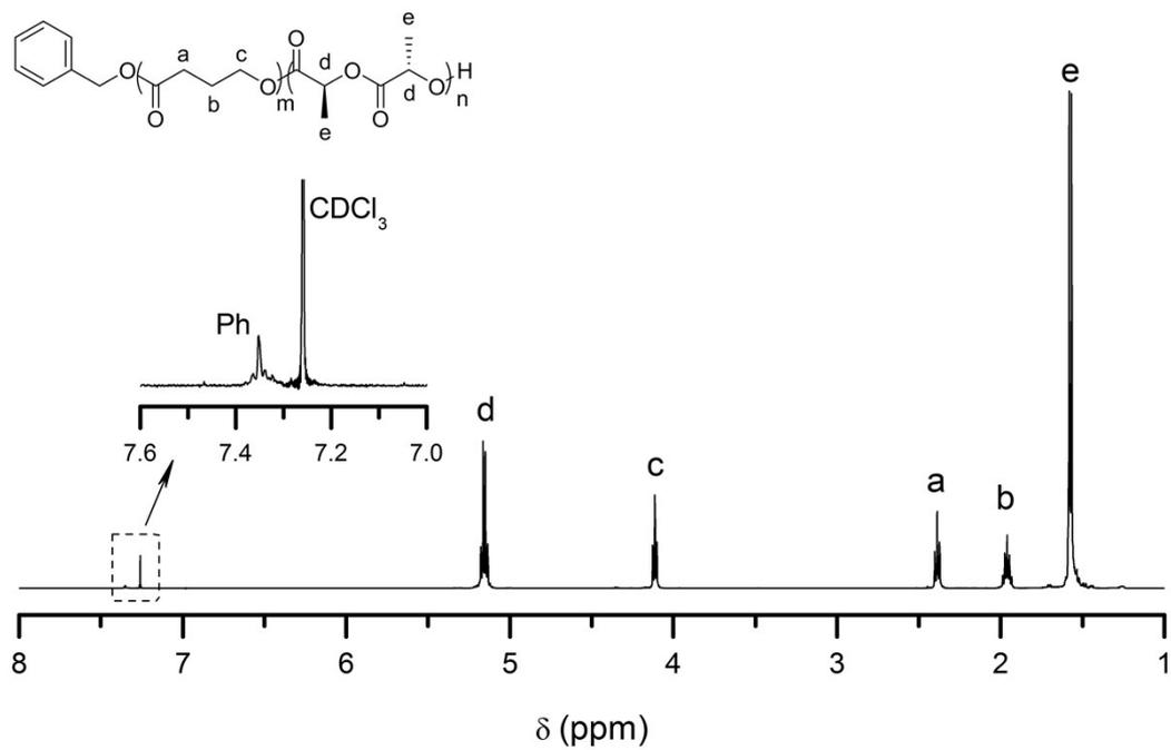
Figure S9. Representative  $^1\text{H}$  NMR spectrum of PyBL-*b*-PLLA. Deuterated chloroform was used as solvent.
