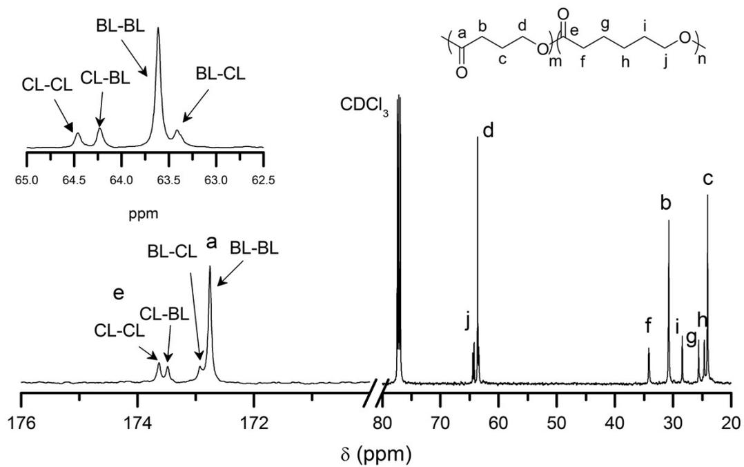
Figure S5.  $^{13}\text{C}$  NMR spectrum of PyBL-co-PCL (Table S3, run 1). Deuterated chloroform was used as solvent.
