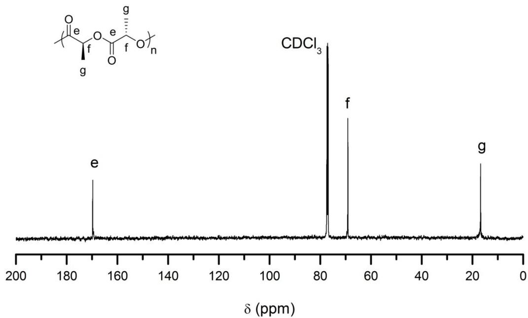
Figure S11. Representative  $^{13}C$  NMR spectrum of PLLA. Deuterated chloroform was used as solvent.
