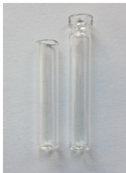
Figure S1. Left: vial after removal of the top part; right: crimped photo glass vial.
