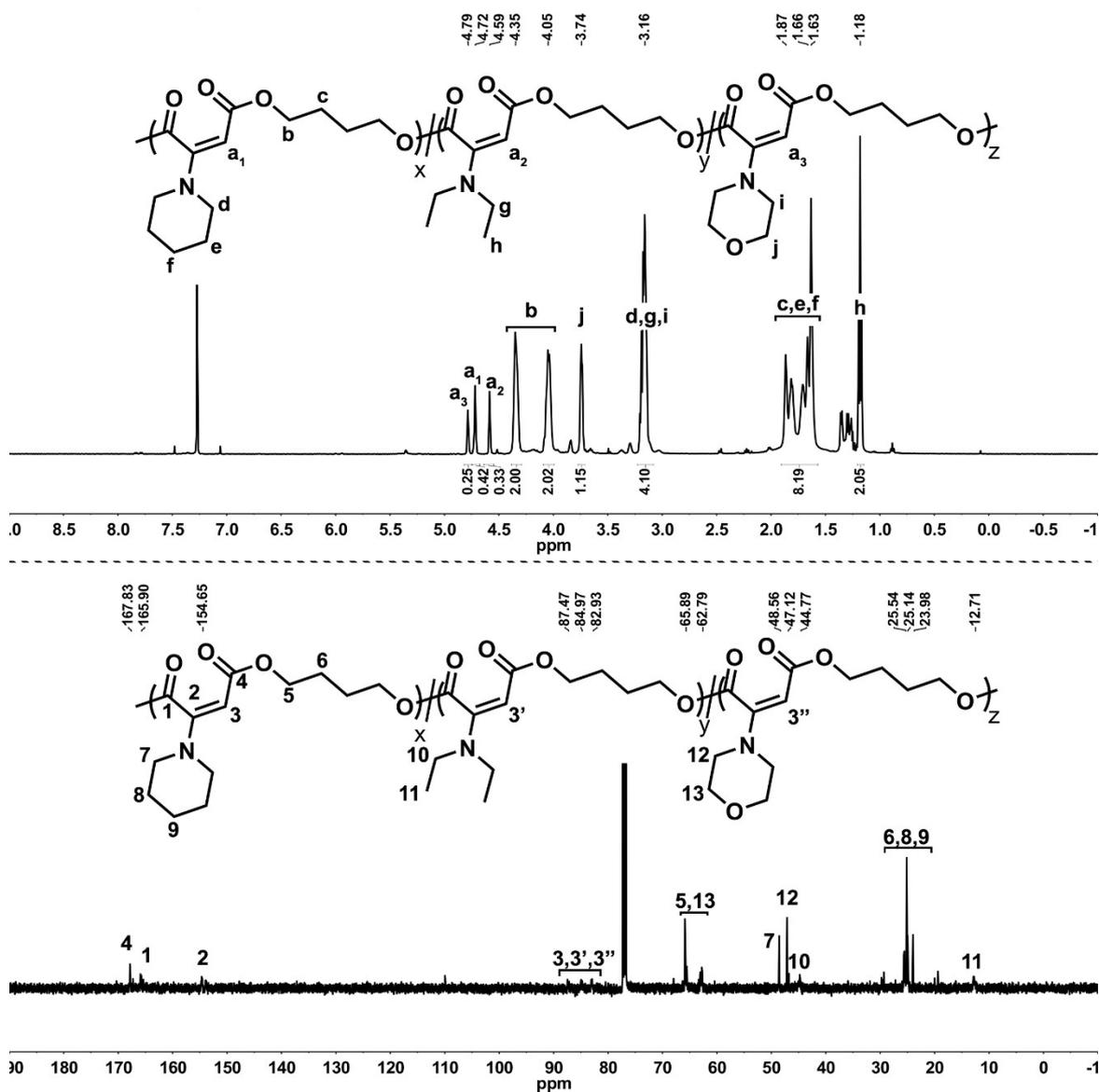
**Figure S9.**  $^1\text{H}$  (up) and  $^{13}\text{C}$  NMR (down) spectra of **P7** in  $\text{CDCl}_3$  (500 and 125 MHz, respectively).
