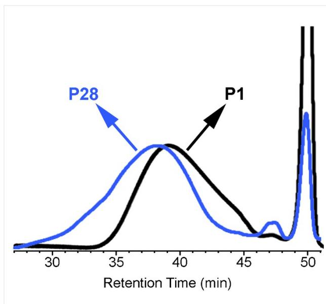
**Figure S45.** Overlaid GPC traces of **P1** and **P28** (at 30 °C in THF).
