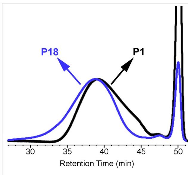
Figure S28. Overlaid GPC traces of P1 and P18 (at 30 °C in THF).
