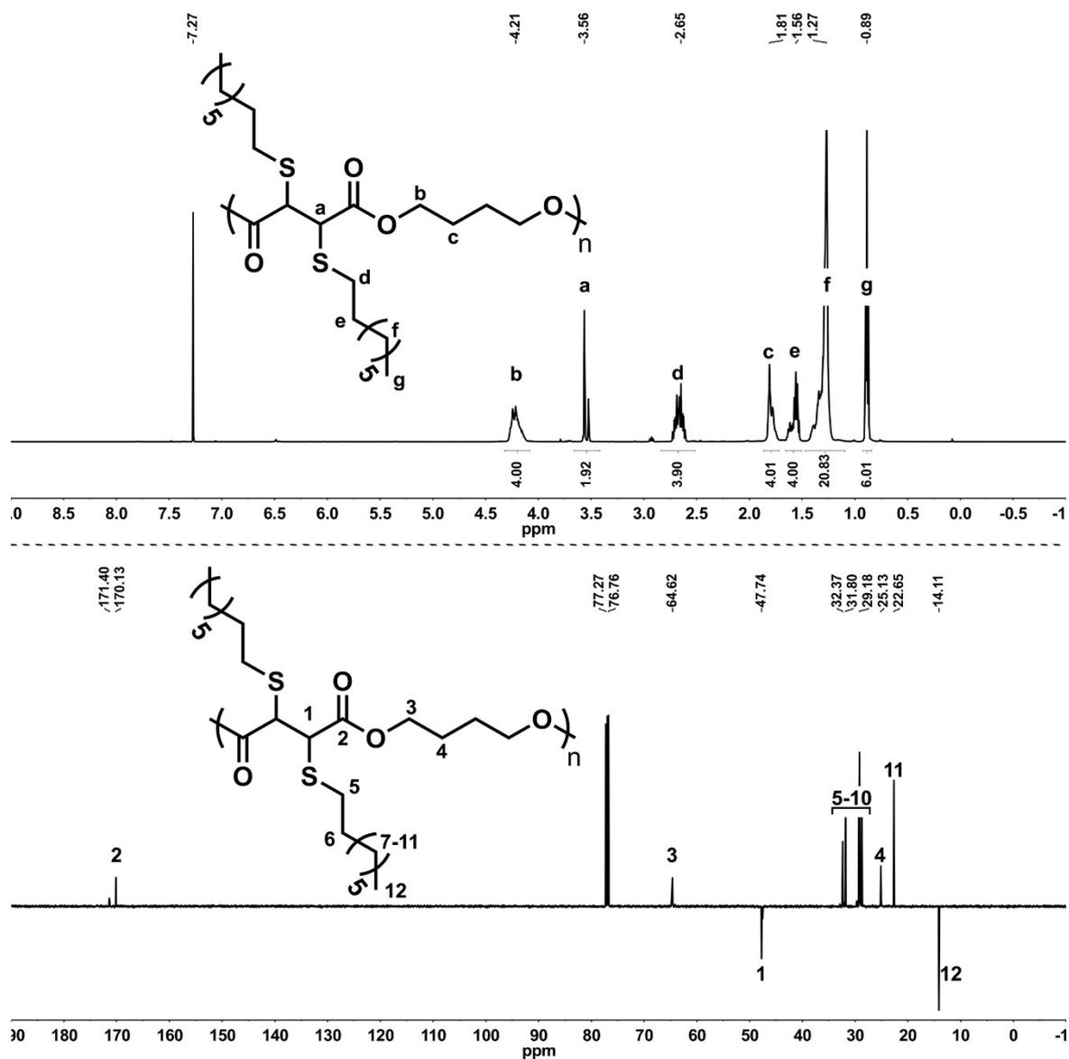
**Figure S34.** <sup>1</sup>H (up) and <sup>13</sup>C APT (down) spectra of P22 in CDCl<sub>3</sub> (500 and 125 MHz, respectively).
