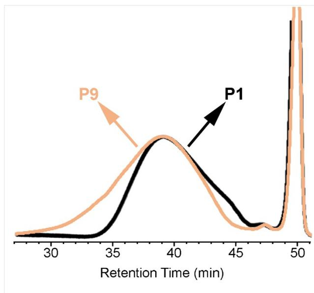
**Figure S12.** Overlaid GPC traces of **P1** and **P9** (at 30 °C in THF).
