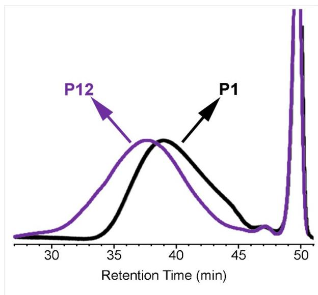
**Figure S18.** Overlaid GPC traces of **P1** and **P12** (at 30 °C in THF).
