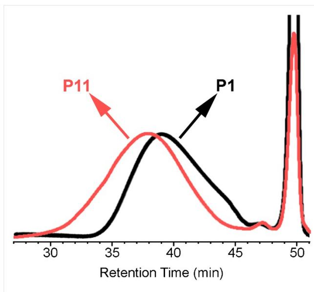
**Figure S16.** Overlaid GPC traces of **P1** and **P11** (at 30 °C in THF).
