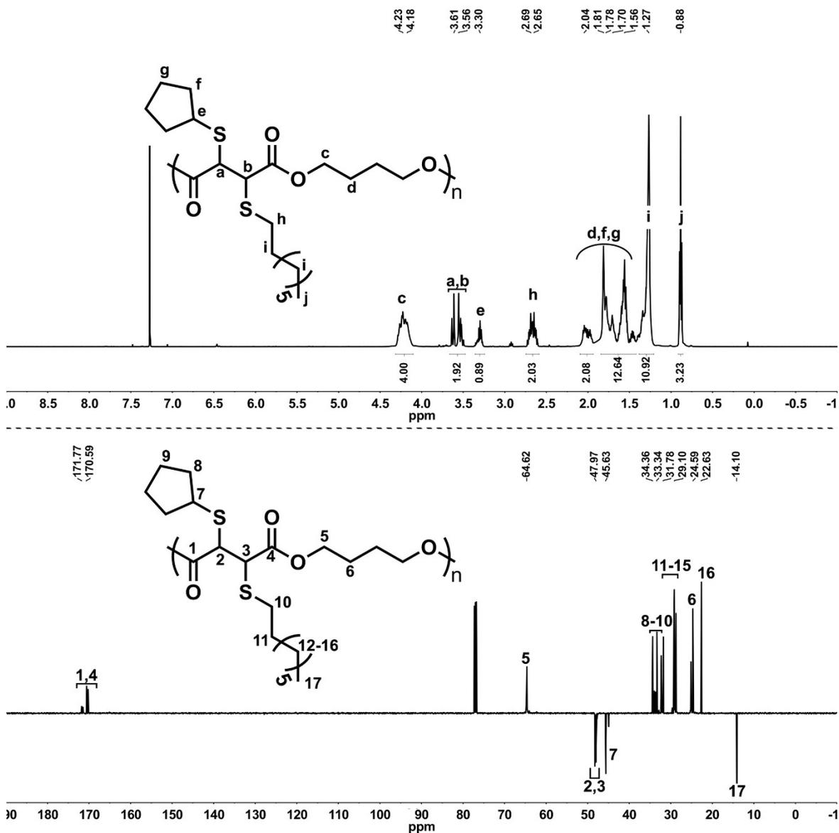
**Figure S42.** <sup>1</sup>H (up) and <sup>13</sup>C APT (down) spectra of **P27** in CDCl<sub>3</sub> (500 and 125 MHz, respectively).
