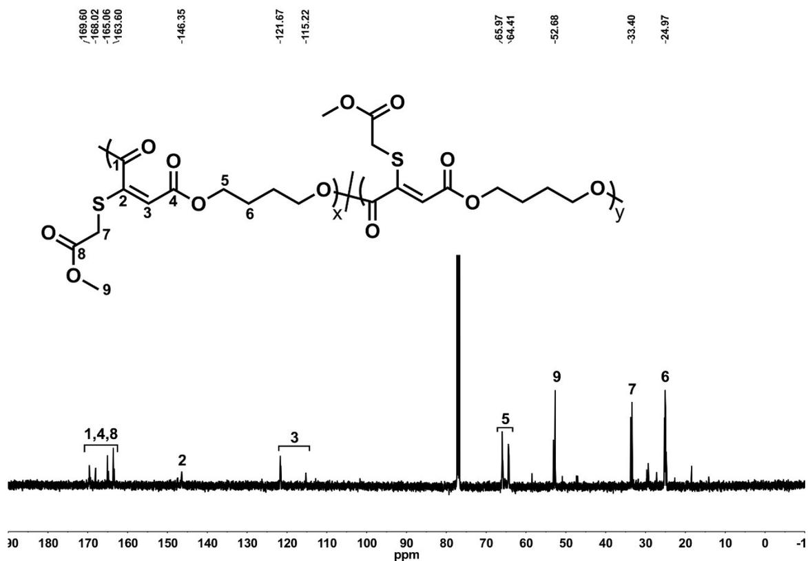
Figure S27.  $^{13}\text{C}$  NMR spectrum of P18 in  $\text{CDCl}_3$  (125 MHz).
