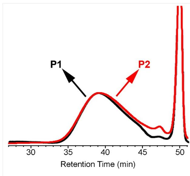
**Figure S1.** Overlaid GPC traces of **P1** and **P2** (at 30 °C in THF).
