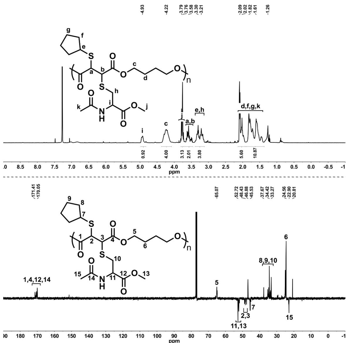
**Figure S48.**  $^1\text{H}$  (up) and  $^{13}\text{C}$  APT (down) spectra of P30 in  $\text{CDCl}_3$  (500 and 125 MHz, respectively).
