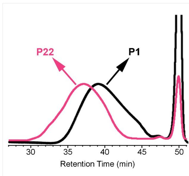
**Figure S35.** Overlaid GPC traces of **P1** and **P22** (at 30 °C in THF).
