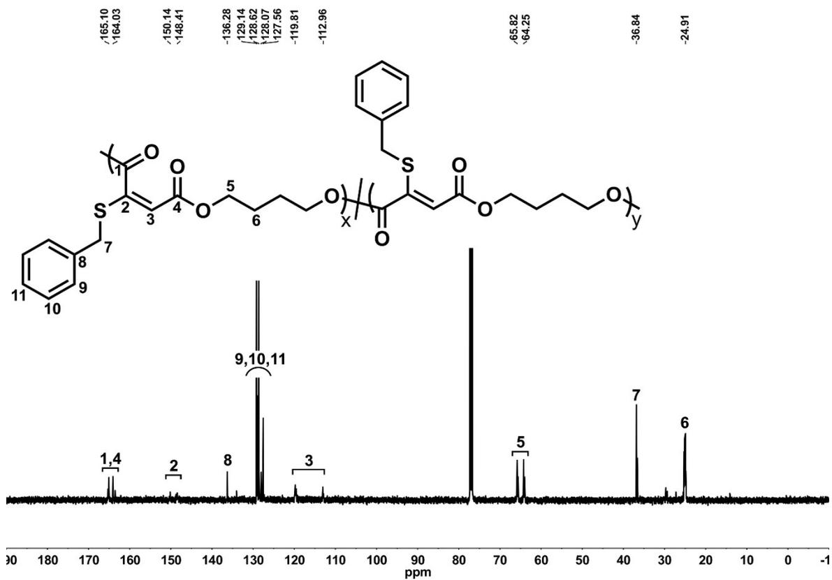
Figure S25. <sup>13</sup>C NMR spectrum of P17 in CDCl<sub>3</sub> (125 MHz).
