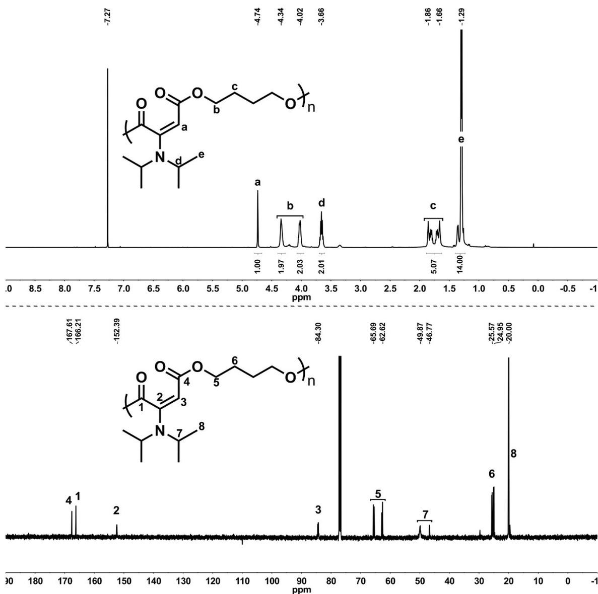
**Figure S2.** <sup>1</sup>H (up) and <sup>13</sup>C NMR (down) spectra of **P3** in CDCl<sub>3</sub> (500 and 125 MHz, respectively).
