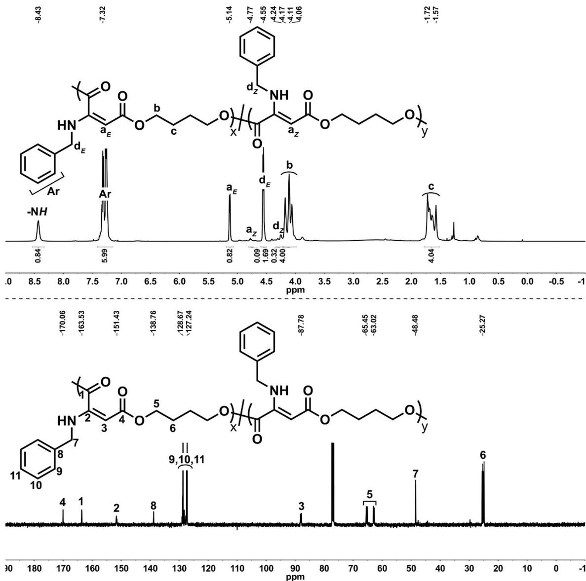
**Figure S17.** <sup>1</sup>H (up) and <sup>13</sup>C NMR (down) spectra of **P12** in CDCl<sub>3</sub> (500 and 125 MHz, respectively).
