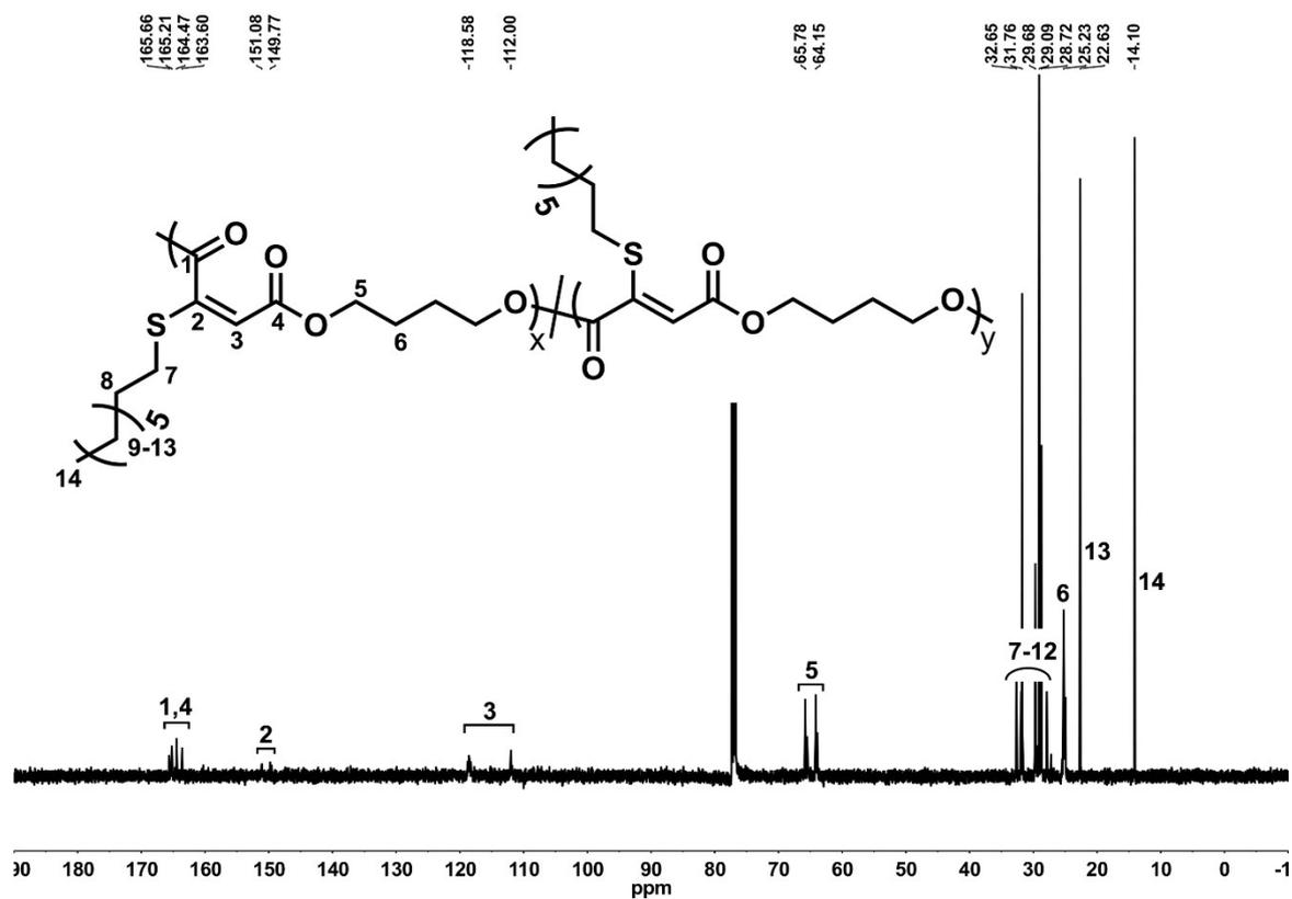
Figure S23.  $^{13}\text{C}$  NMR spectrum of P16 in  $\text{CDCl}_3$  (125 MHz).
