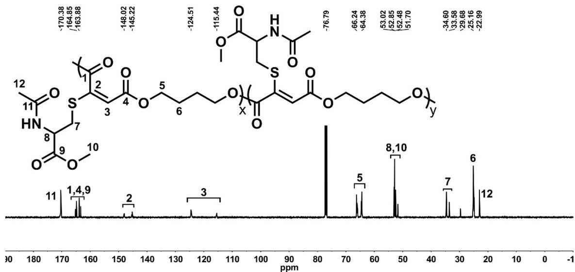
Figure S29.  $^{13}\text{C}$  NMR spectrum of P19 in  $\text{CDCl}_3$  (125 MHz).
