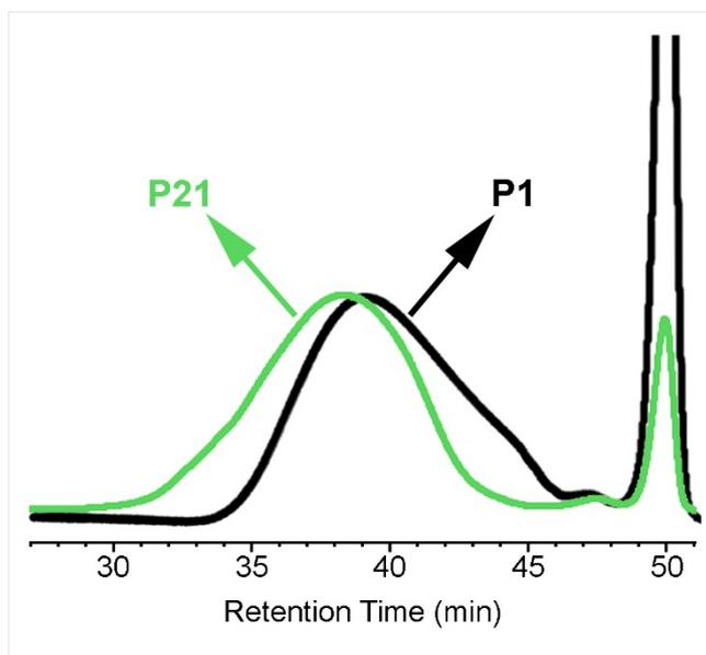
**Figure S33.** Overlaid GPC traces of **P1** and **P21** (at 30 °C in THF).
