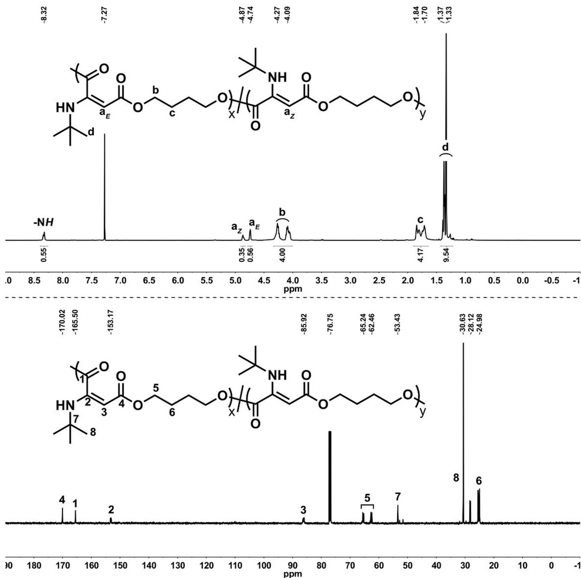
**Figure S15.** <sup>1</sup>H (up) and <sup>13</sup>C NMR (down) spectra of **P11** in CDCl<sub>3</sub> (500 and 125 MHz, respectively).
