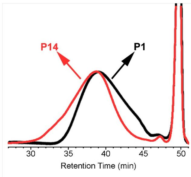
**Figure S21.** Overlaid GPC traces of **P1** and **P14** (at 30 °C in THF).
