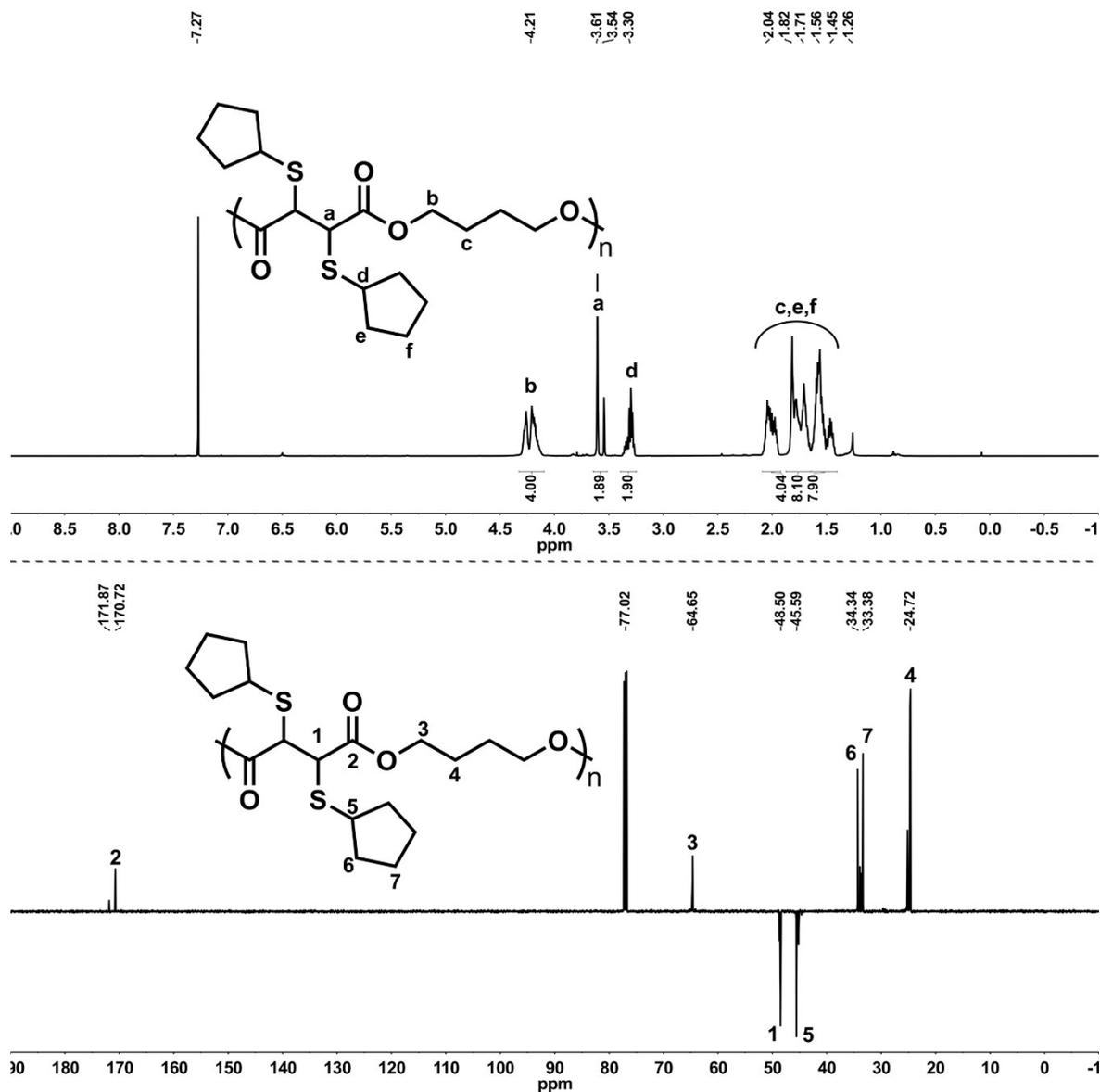
**Figure S32.** <sup>1</sup>H (up) and <sup>13</sup>C APT (down) spectra of **P21** in CDCl<sub>3</sub> (500 and 125 MHz, respectively).
