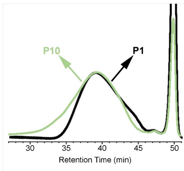
**Figure S14.** Overlaid GPC traces of **P1** and **P10** (at 30 °C in THF).
