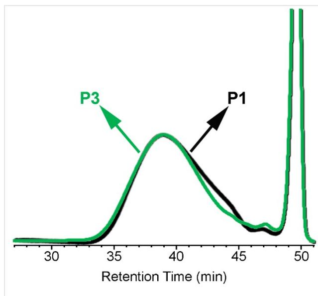
**Figure S3.** Overlaid GPC traces of **P1** and **P3** (at 30 °C in THF).
