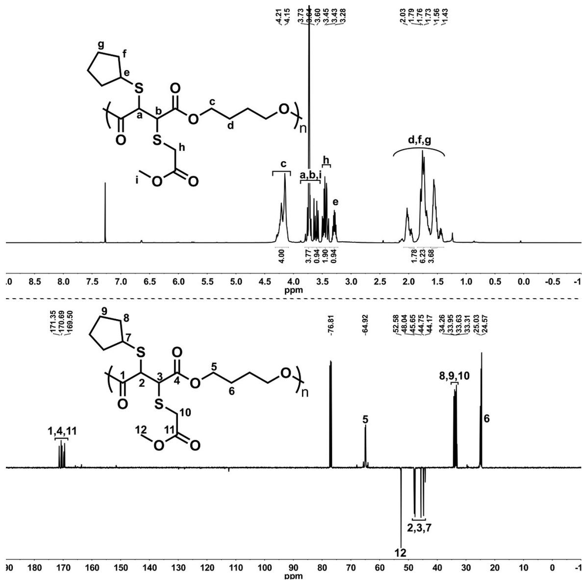
**Figure S46.** <sup>1</sup>H (up) and <sup>13</sup>C APT (down) spectra of **P29** in CDCl<sub>3</sub> (500 and 125 MHz, respectively).
