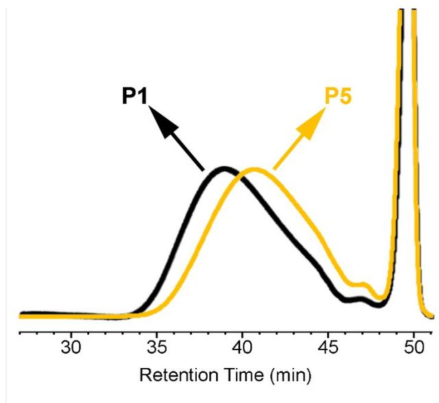
Figure S7. Overlaid GPC traces of **P1** and **P5** (at 30 °C in THF).
