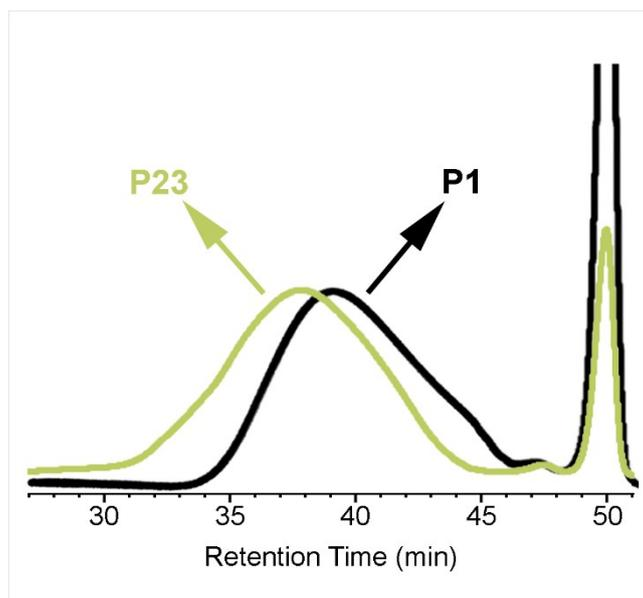
**Figure S37.** Overlaid GPC traces of **P1** and **P23** (at 30 °C in THF).
