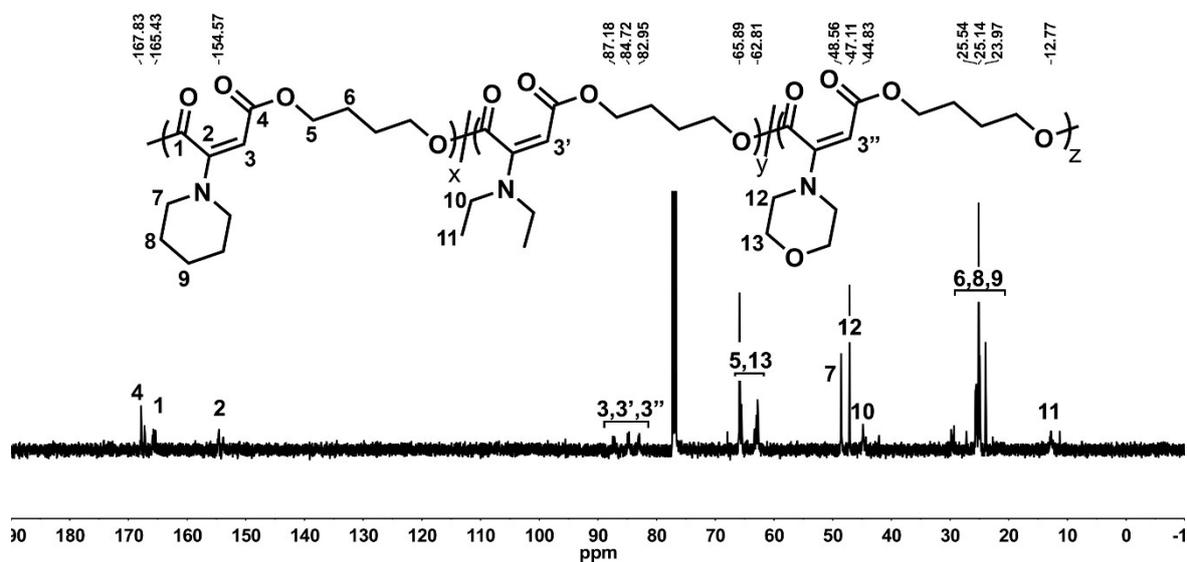
Figure S8.  $^{13}\text{C}$  NMR spectrum of **P6** in  $\text{CDCl}_3$  (125 MHz).
