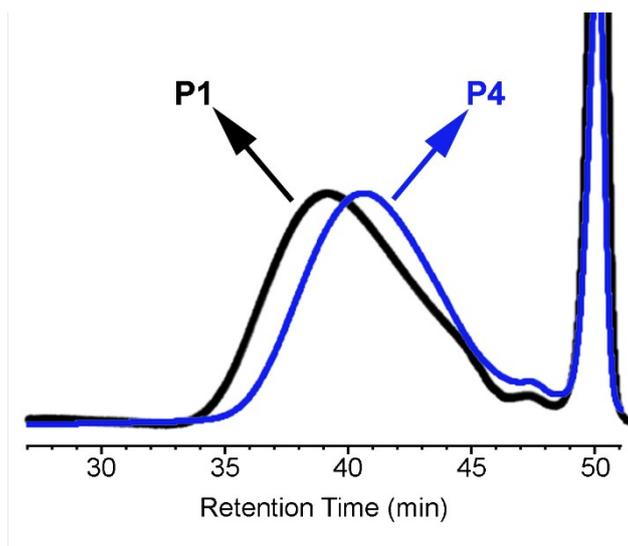
**Figure S5.** Overlaid GPC traces of **P1** and **P4** (at 30 °C in THF).
