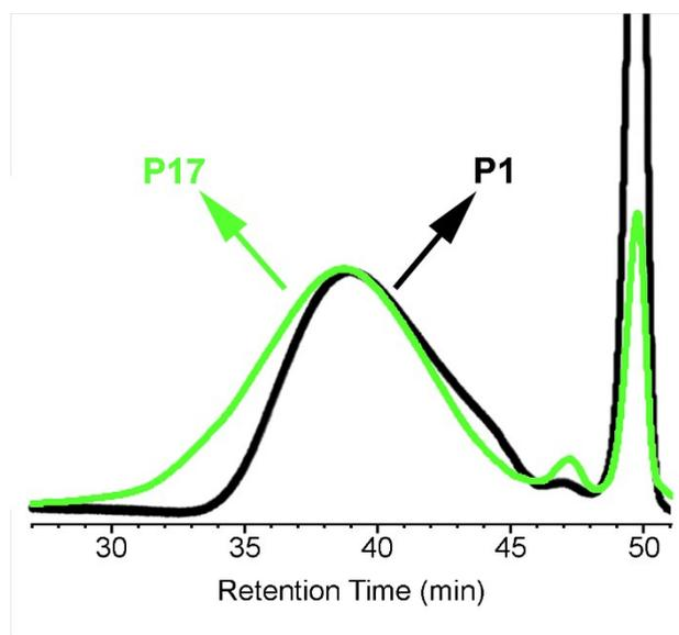
Figure S26. Overlaid GPC traces of P1 and P17 (at 30 °C in THF).
