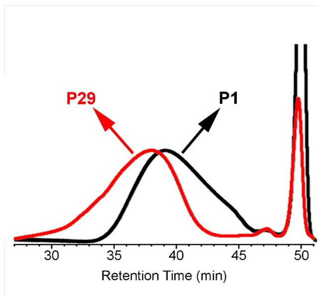
**Figure S47.** Overlaid GPC traces of **P1** and **P29** (at 30 °C in THF).
