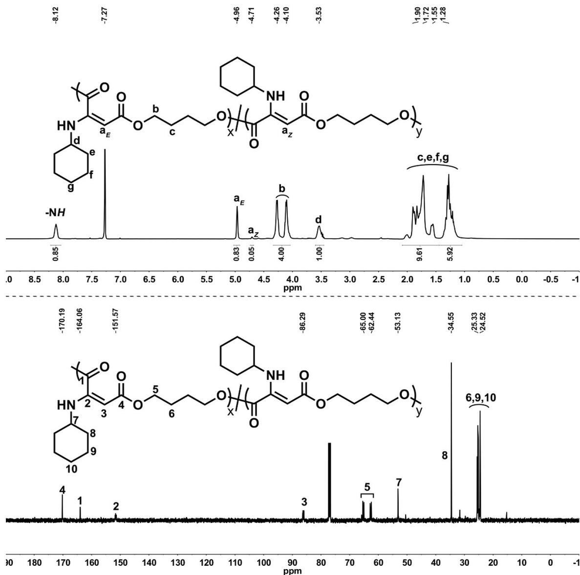
**Figure S11.** <sup>1</sup>H (up) and <sup>13</sup>C NMR (down) spectra of **P9** in CDCl<sub>3</sub> (500 and 125 MHz, respectively).
