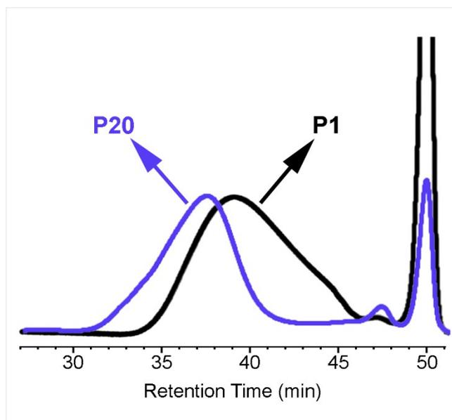
**Figure S31.** Overlaid GPC traces of **P1** and **P20** (at 30 °C in THF).
