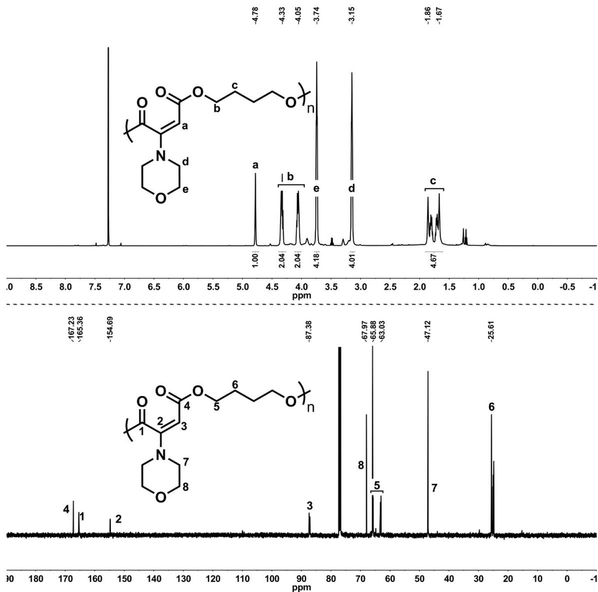
**Figure S6.** <sup>1</sup>H (up) and <sup>13</sup>C NMR (down) spectra of **P5** in CDCl<sub>3</sub> (500 and 125 MHz, respectively).
