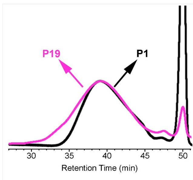
Figure S30. Overlaid GPC traces of P1 and P19 (at 30 °C in THF).
