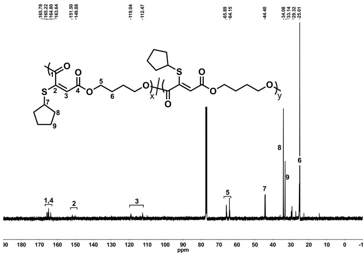
Figure S22. <sup>13</sup>C NMR spectrum of P15 in CDCl<sub>3</sub> (125 MHz).
