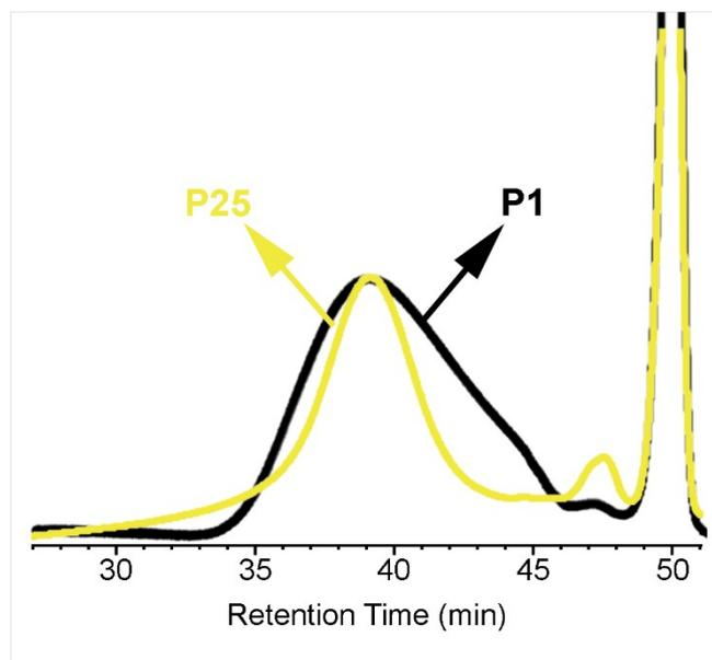
**Figure S41.** Overlaid GPC traces of **P1** and **P25** (at 30 °C in THF).
