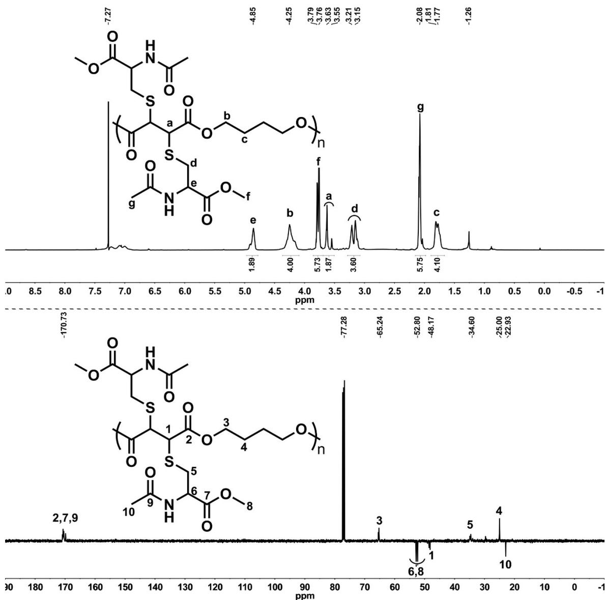
**Figure S40.**  $^1\text{H}$  (up) and  $^{13}\text{C}$  APT (down) spectra of **P25** in  $\text{CDCl}_3$  (500 and 125 MHz, respectively).
