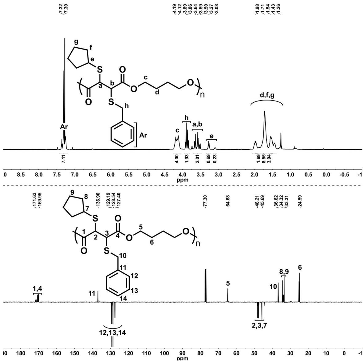
**Figure S44.** <sup>1</sup>H (up) and <sup>13</sup>C APT (down) spectra of **P28** in CDCl<sub>3</sub> (500 and 125 MHz, respectively).
