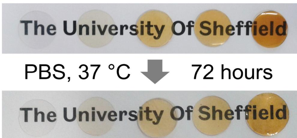
**Fig. S4** Photographs of PGSG copolymers before and after swelling in phosphate buffered saline (PBS) for 72 h at 37 °C (from left to right PGSG0, PGSG5, PGSG10, PGSG15, and PGSG20), showing volume expansions.
