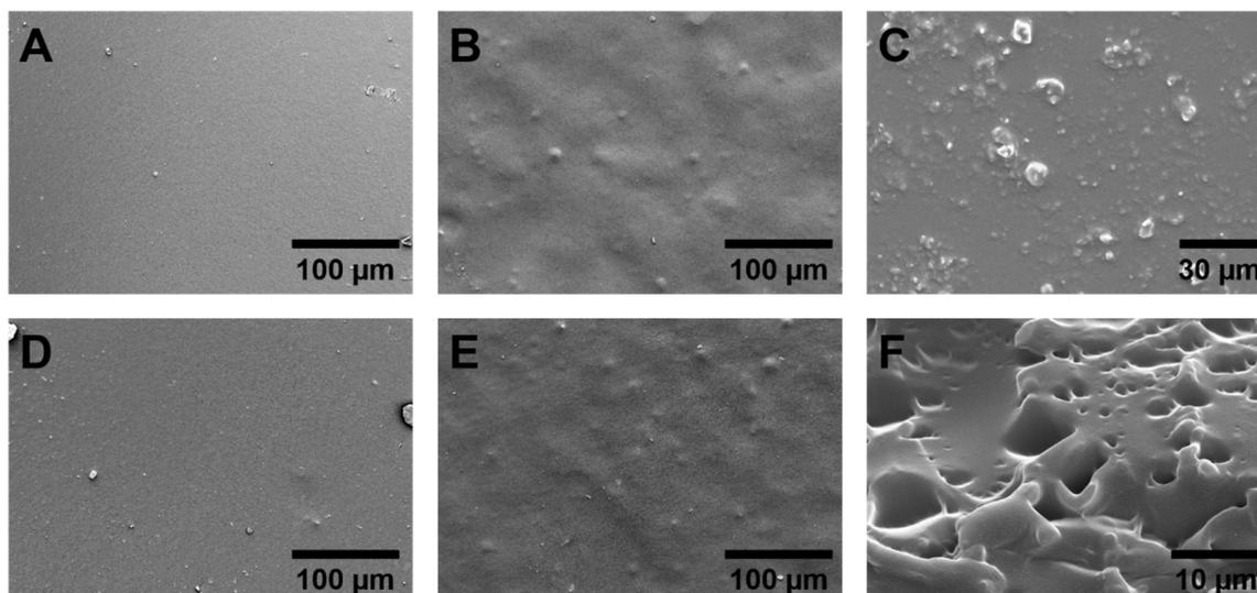
**Fig. S6** Scanning electron microscopy (SEM) images showing the surface of PGSG specimens after degradation. (A-C) PGSG10 incubated for 28 days at 37 °C in (A) PBS only, (B) lipase + PBS, and (C) collagenase + PBS. (D-F) PGSG20 incubated for 28 days at 37 °C in (D) PBS only, (E) lipase + PBS, and (F) collagenase + PBS.
