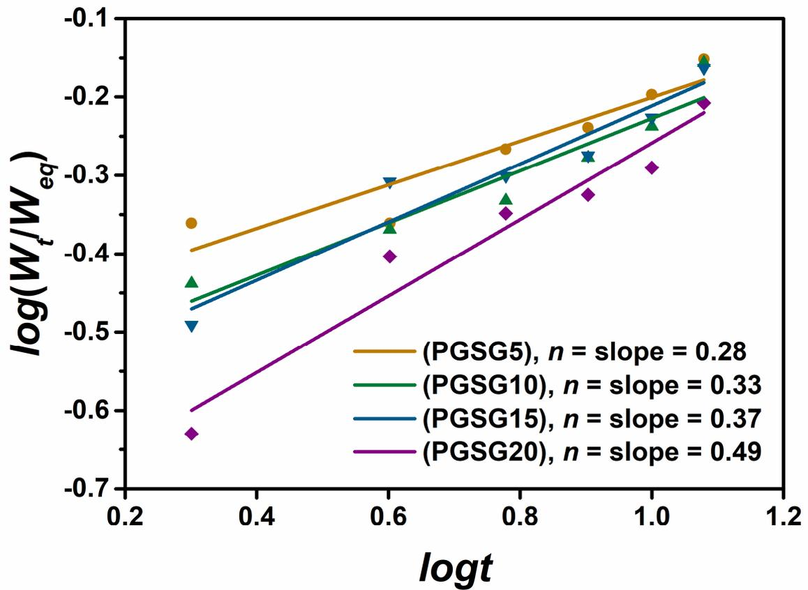
**Fig. S5** The swelling ratio of PGSGs fit to Ritger-Peppas equation, with the  $n$  values shown by the slope of the fitting lines.
