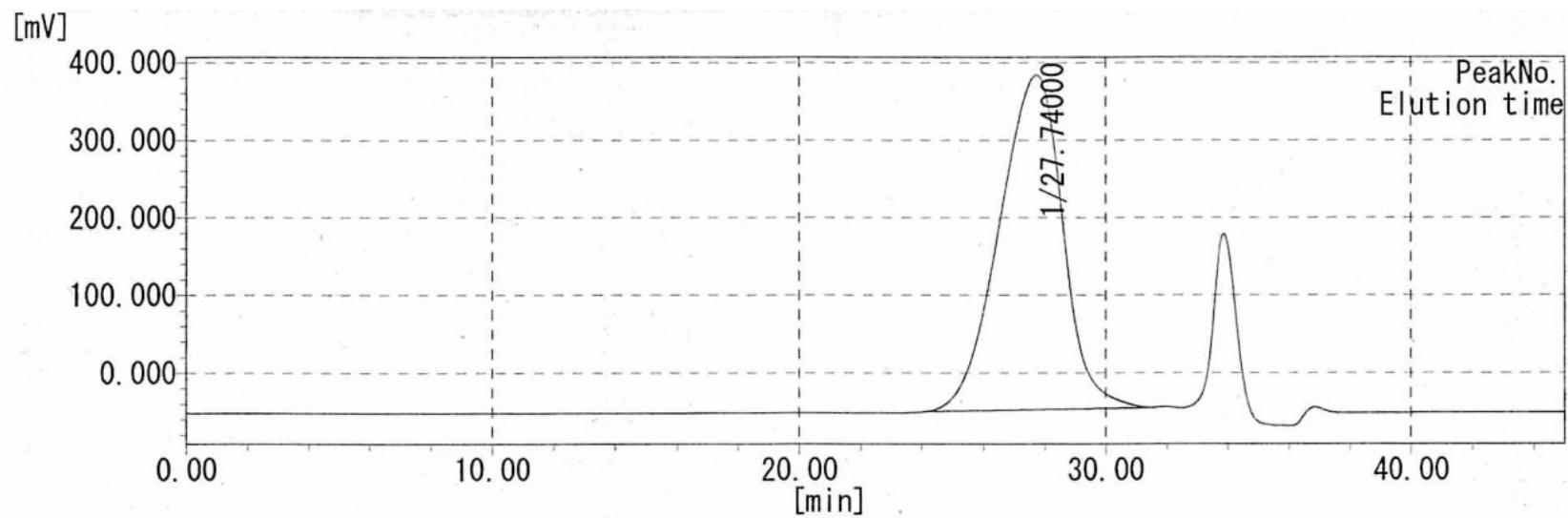
**Fig. S7** SEC curve of poly(**1b**) (Sample: Table 1, run 5).
