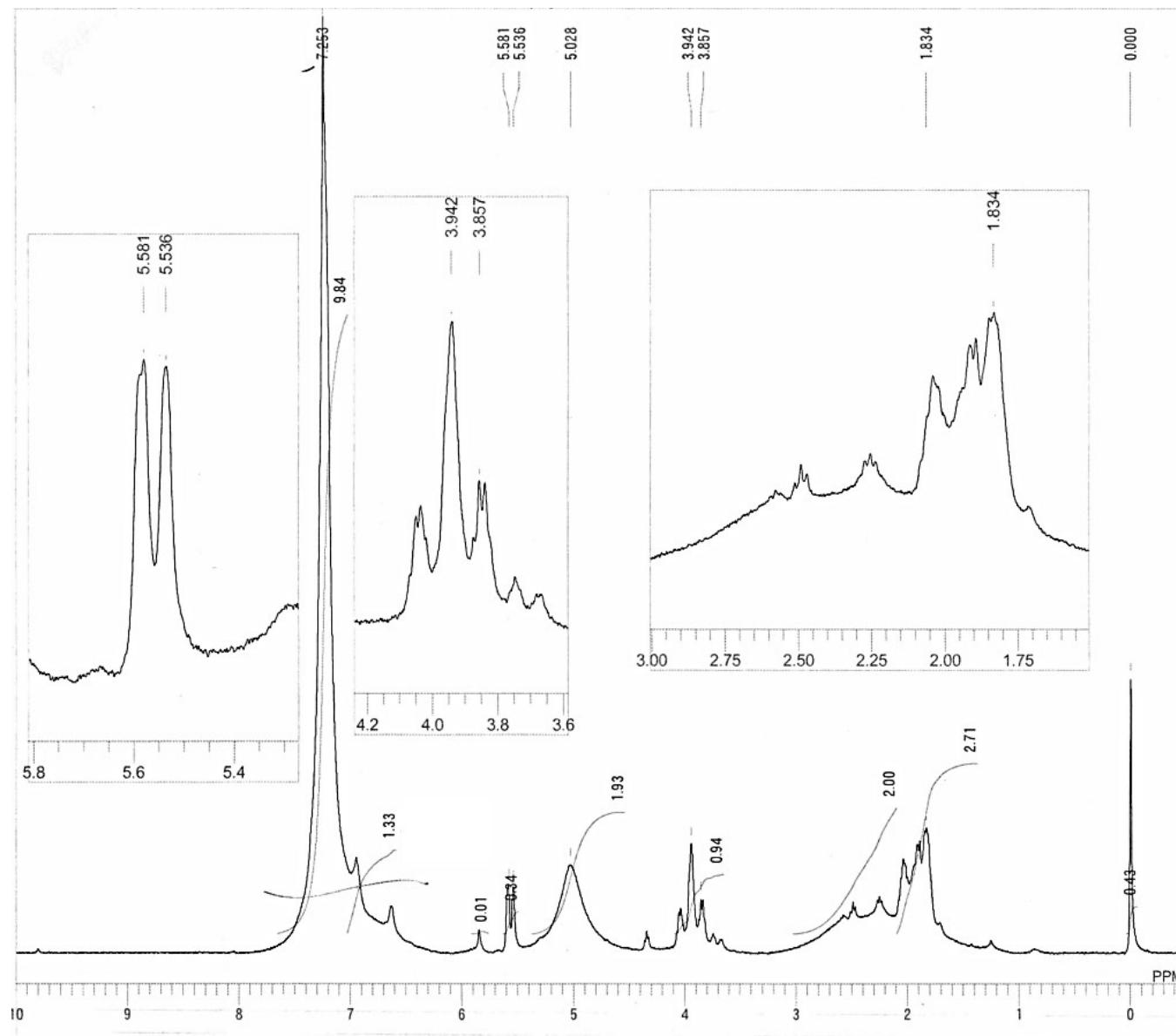
**Fig. S17**  $^1\text{H}$  NMR (400 MHz) spectrum of poly(**1a**)-*block*-poly(**2b**) measured in  $\text{CDCl}_3$ .
