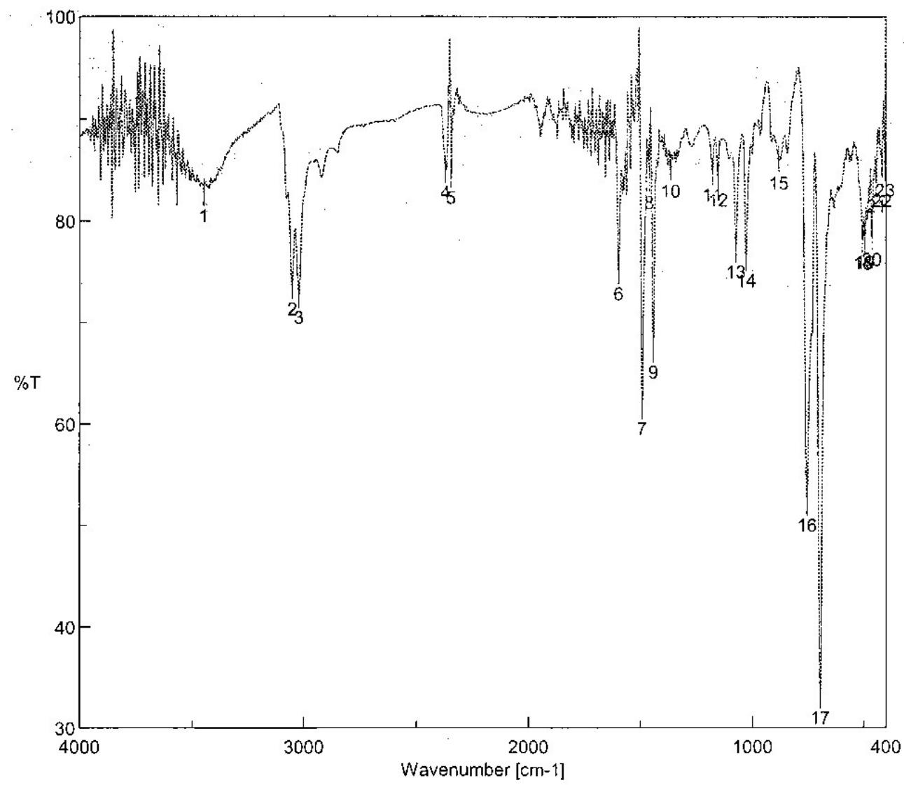
**Fig. S2** IR spectrum of poly(1a).
