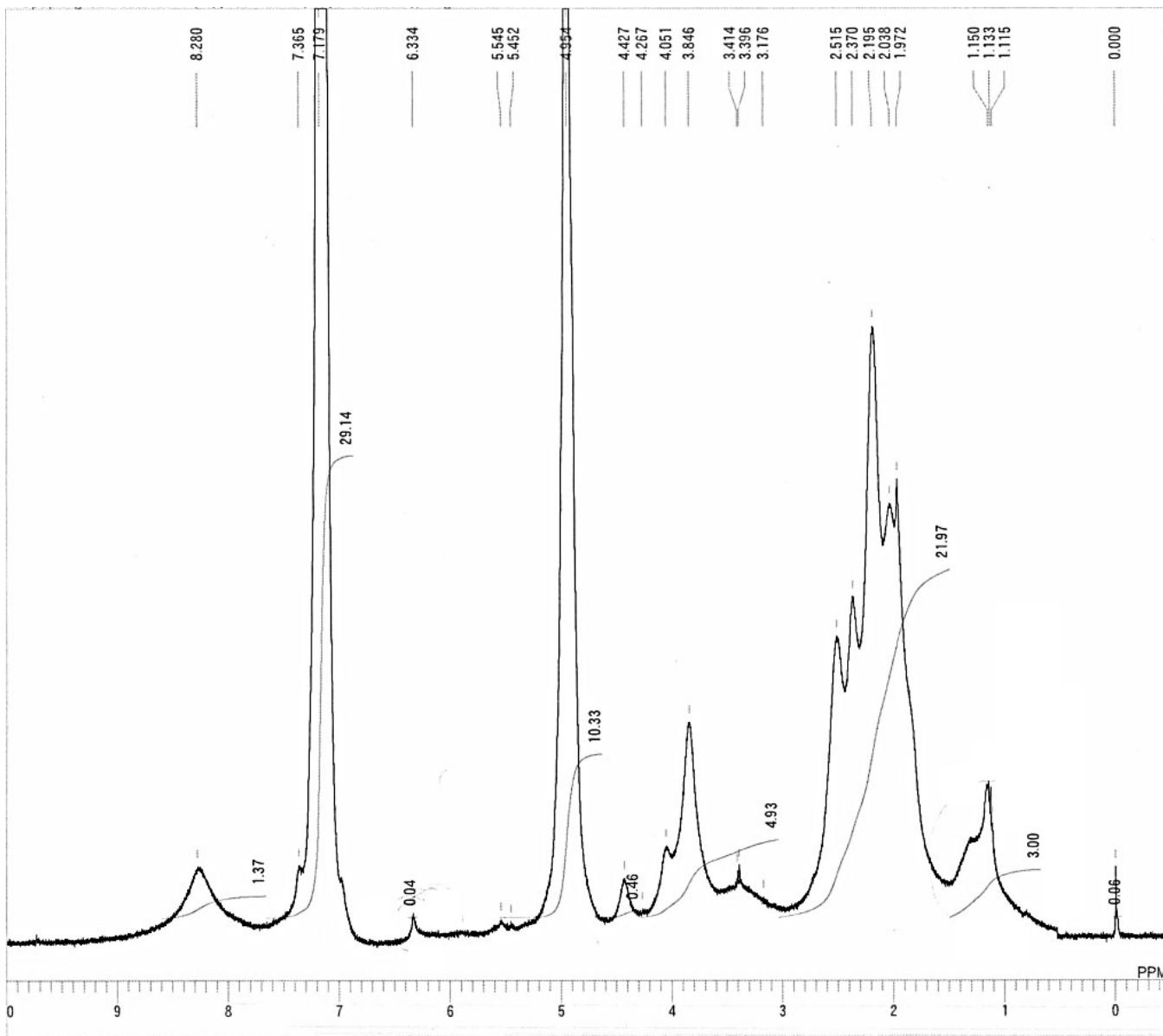
**Fig. S23** <sup>1</sup>H NMR (400 MHz) spectrum of poly(**1c**)-block-poly(**2b**) measured in  $\text{CDCl}_3$ .
