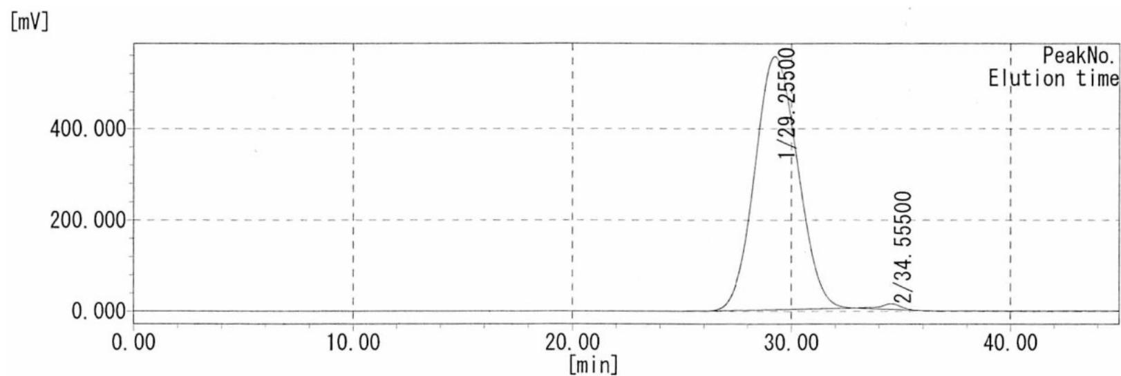
**Fig. S13** SEC curve of poly(**1a**) after Si coupling.
