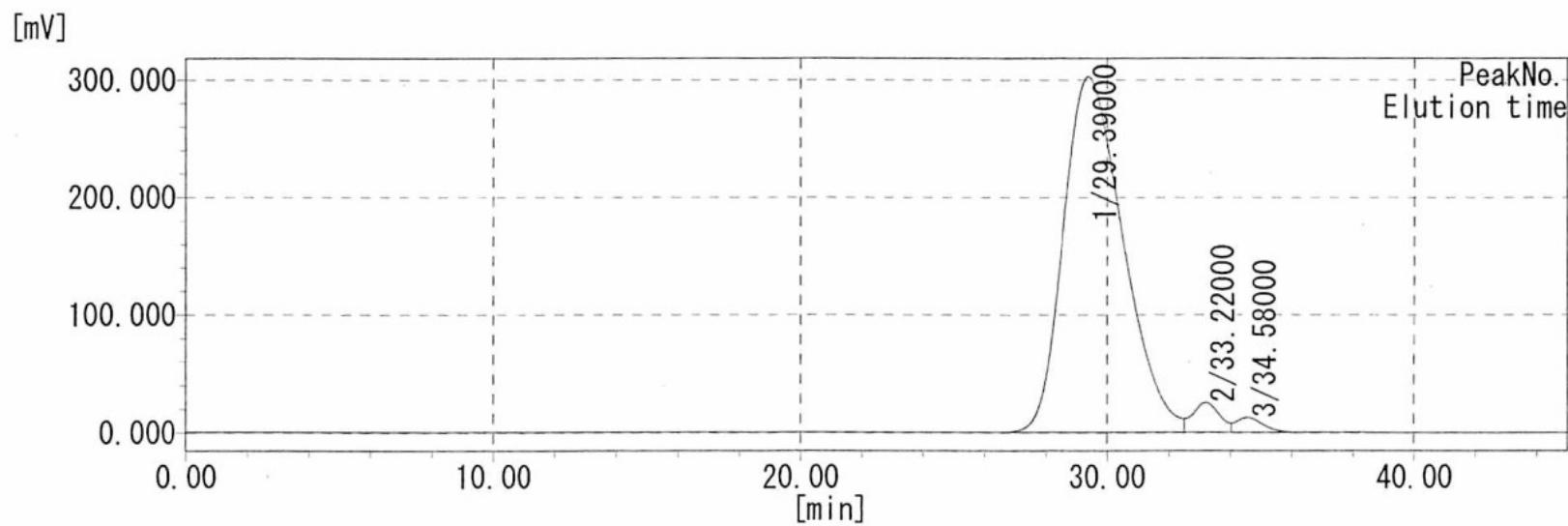
**Fig. S12** SEC curve of poly(**1a**) before Si coupling.
