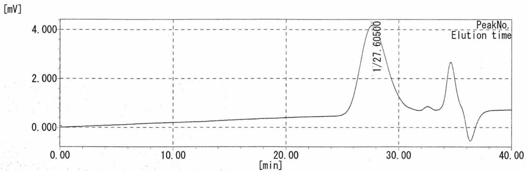
**Fig. S4** SEC curve of poly(**1a**) (Sample: Table 1, run 2).
