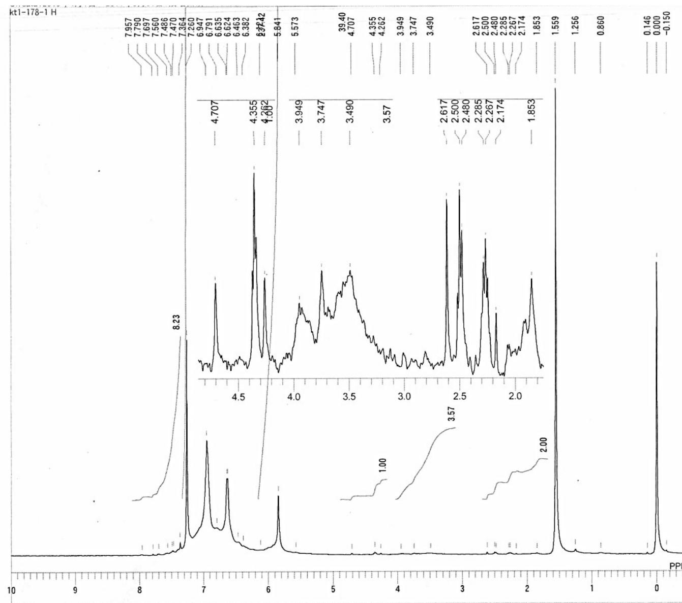
**Fig. S1**  $^1\text{H}$  NMR (400 MHz) spectrum of poly(**1a**) measured in  $\text{CDCl}_3$ .
