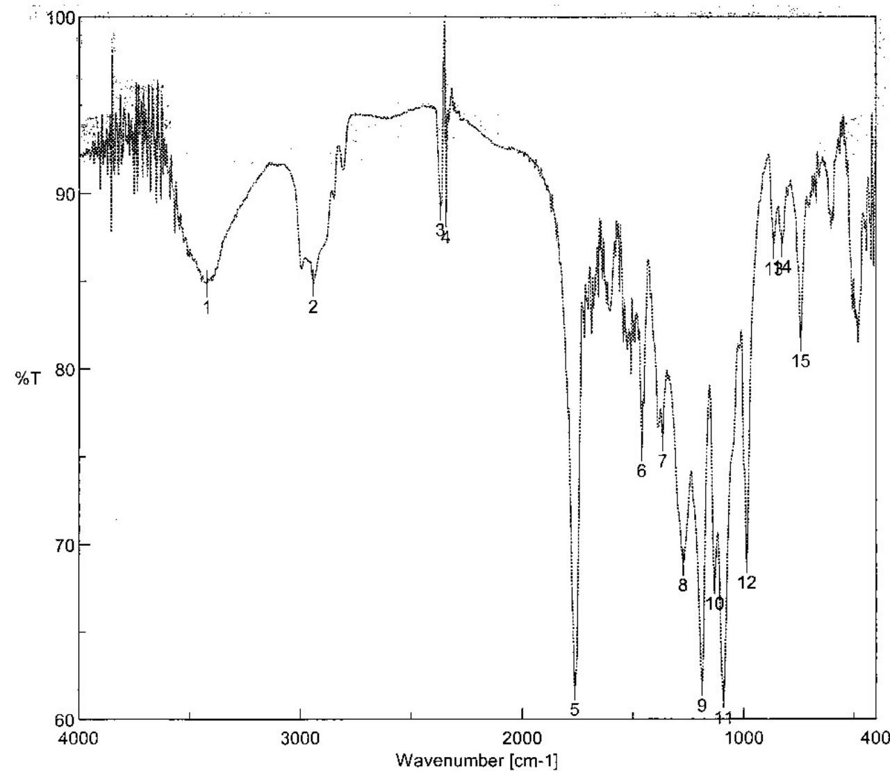
**Fig. S21** IR spectrum of poly(**1b**)-block-poly(**2a**).
