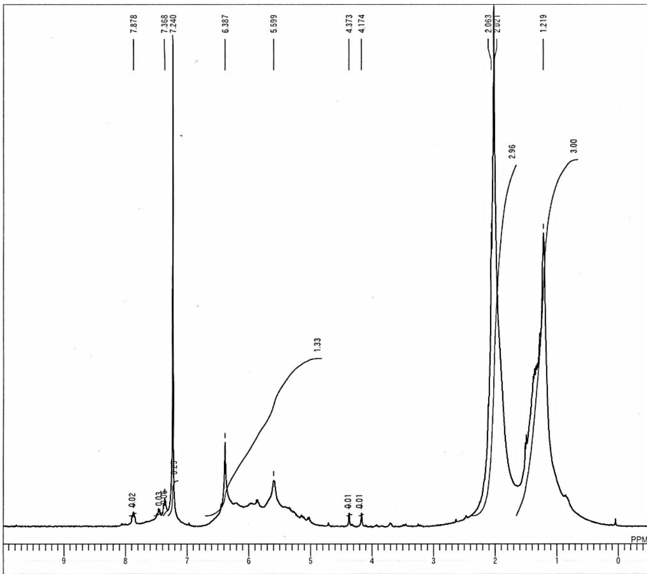
**Fig. S8** <sup>1</sup>H NMR (400 MHz) spectrum of poly(**1c**) measured in CDCl<sub>3</sub>.
