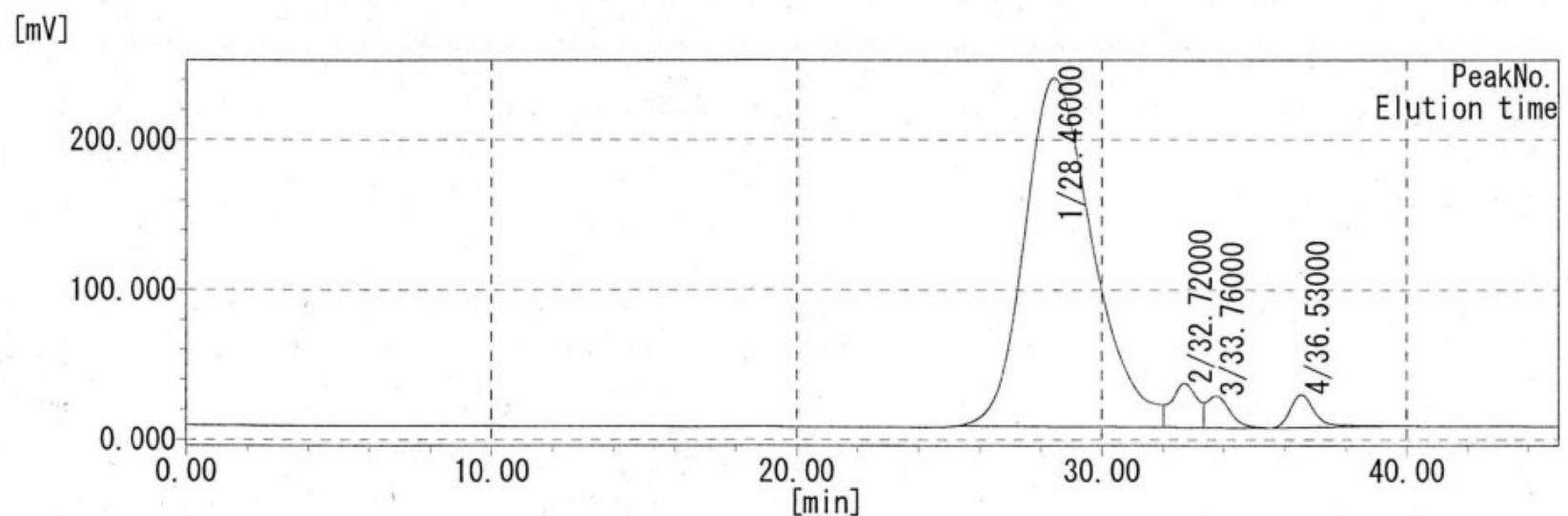
**Fig. S3** SEC curve of poly(**1a**) (Sample: Table 1, run 1).
