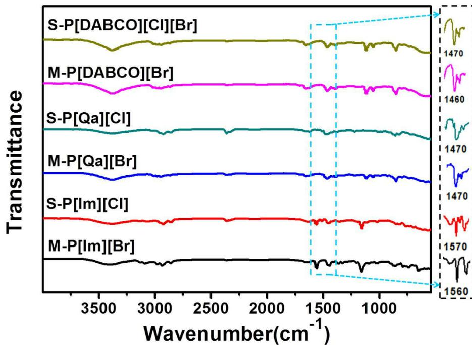
**Figure S2.** FTIR spectra of the side-chain/main-chain cationic polymers.
