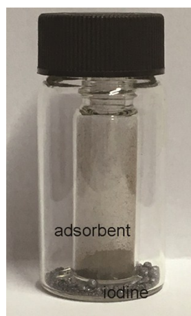
Fig. S6 Iodine vapor adsorption apparatus set-up.
