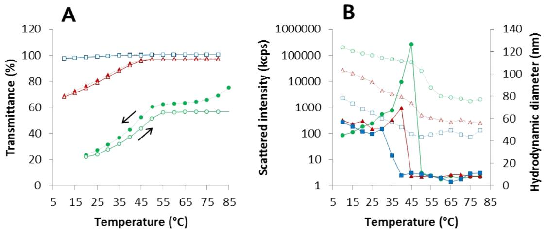
**Figure S6.** Variation of (a) transmittance, (b) hydrodynamic diameter and scattered intensity with temperature for UCST-2 at 0.01 wt% (circles), 0.1 wt% (square) and 1 wt% (triangle) in water. On Figure S6b, the solid lines correspond to diameter and dash lines correspond to scattered intensity.
