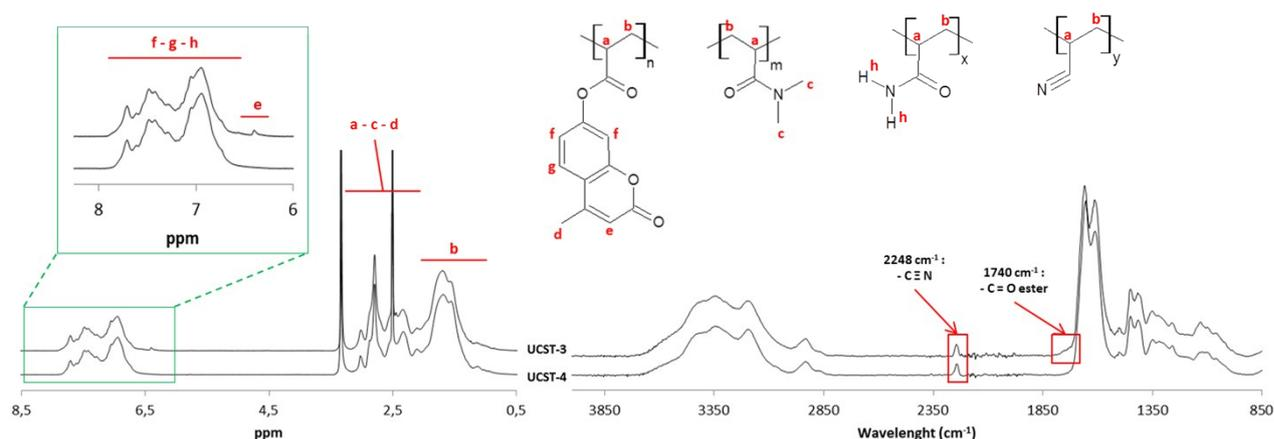
**Figure S2.**  $^1\text{H-NMR}$  and FTIR spectrums of UCST-3 and UCST-4 copolymers.
