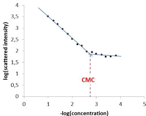
**Figure S3.** Determination of CMC value for UCST-3 copolymer using dynamic light scattering method.
