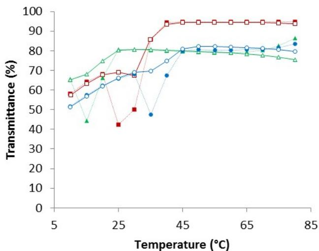
**Figure S8.:** Variation of transmittance with temperature during cooling (dash lines)-heating (solid lines) process for UCST-2 at 1 wt% in 0.05 M (blue circle), 0.1 M (red square) and 0.2 M (green triangle) NaSCN aqueous solutions.
