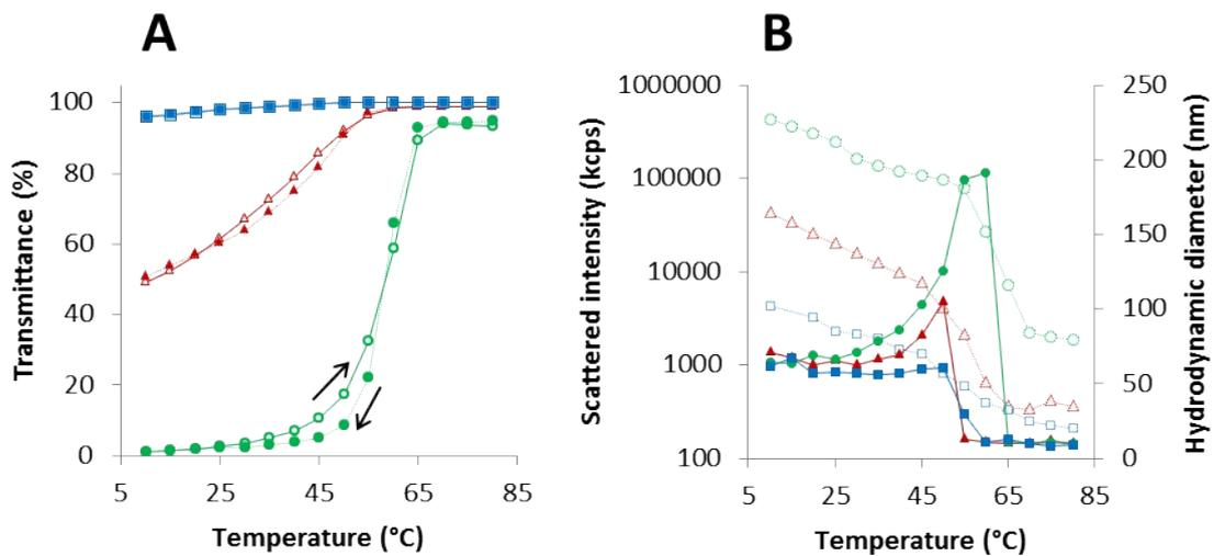
**Figure S7.** Variation of (a) transmittance, (b) hydrodynamic diameter and scattered intensity with temperature for UCST-2 at 0.01 wt% (circles), 0.1 wt% (square) and 1 wt% (triangle) in deuterated water. On Figure S7b, the solid lines correspond to diameter and dash lines correspond to scattered intensity.
