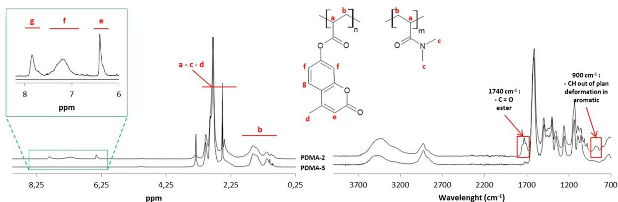
**Figure S1.**  $^1\text{H-NMR}$  and FTIR spectrums of PDMA-2 and PDMA-3 copolymers.
