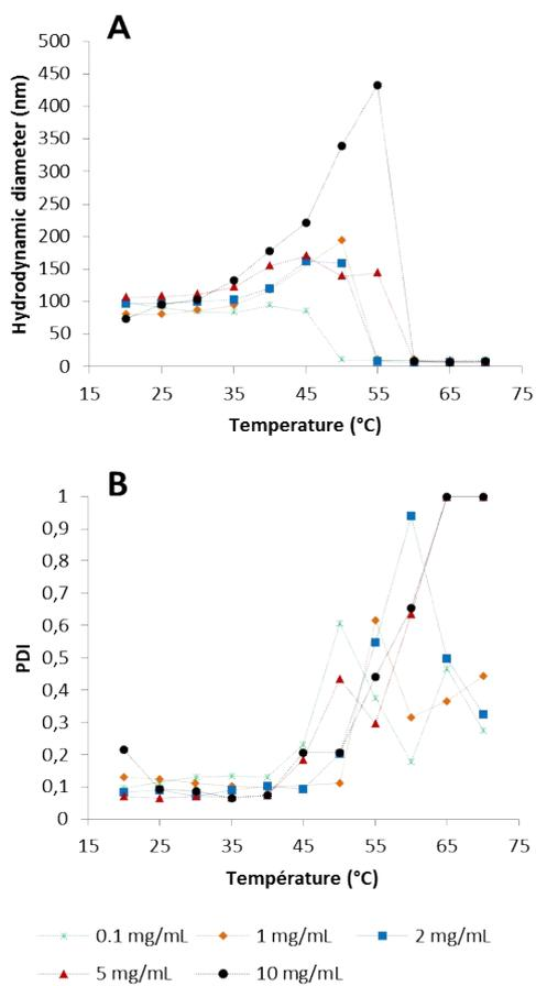
**Figure S4.** Variation of (a) hydrodynamic diameter and (b) polydispersity index with temperature for various concentrations of UCST-3 copolymer in water.
