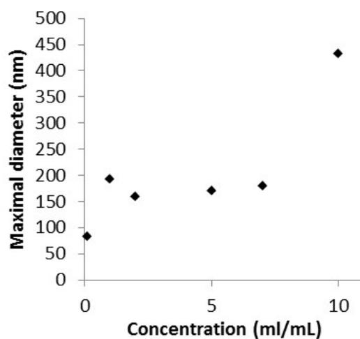
**Figure S5.** Variation of maximal diameter reached just before micelles dissociation as function of copolymer concentration.
