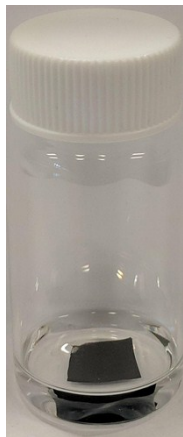
Figure S1. Photograph of the PF-N 3 -SWNT functionalization process. A 1 cm 2 PF-N 3 -SWNT thin film is soaked in a solution of strained cyclooctyne.
