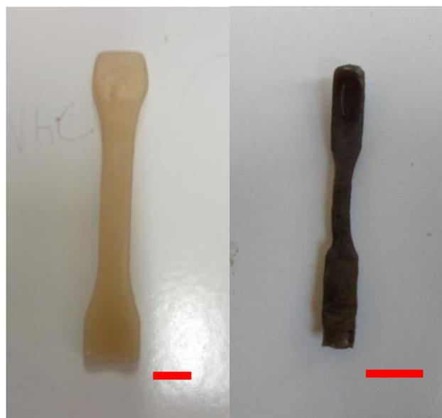
**Figure S6:** Pictures of the shaped PBUuMA composite at (a) 160°C, and (b) 180°C. Scale bar is 1 cm.
