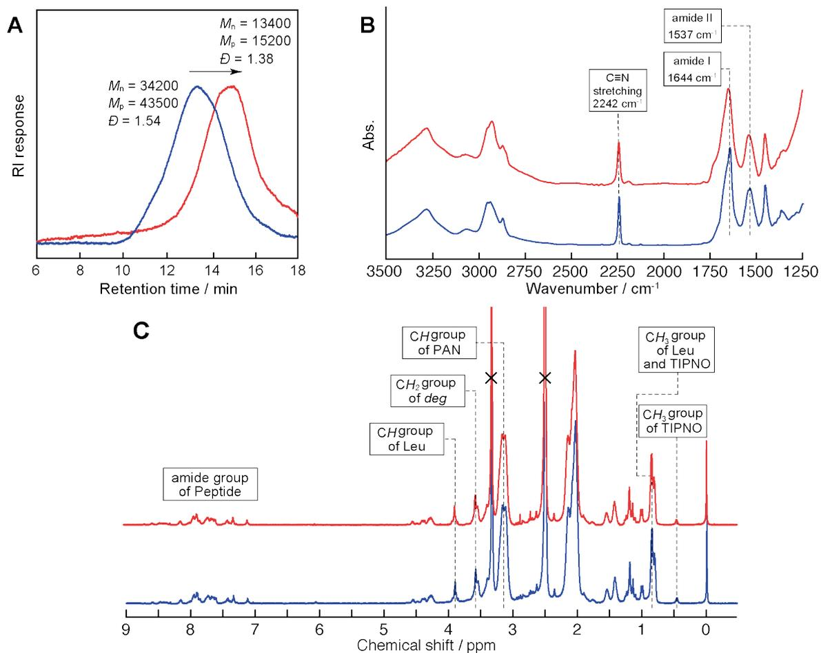
**Figure S19. Characterization of the multiblock P9.** **A.** SEC traces (DMF, 40 °C) of the multiblock **P9** obtained before (blue) and after (red) fragmentation showing a clear shift towards a lower molecular weight. **B.** Transmission-FTIR spectra of **P9** (blue) and fragmented **P9** (red) casted from the DMSO solution onto a  $\text{CaF}_2$  plate. **C.**  $^1\text{H}$  NMR spectra of **P9** (blue) and fragmented **P9** (red) in  $\text{DMSO-}d_6$  at 25°C.
