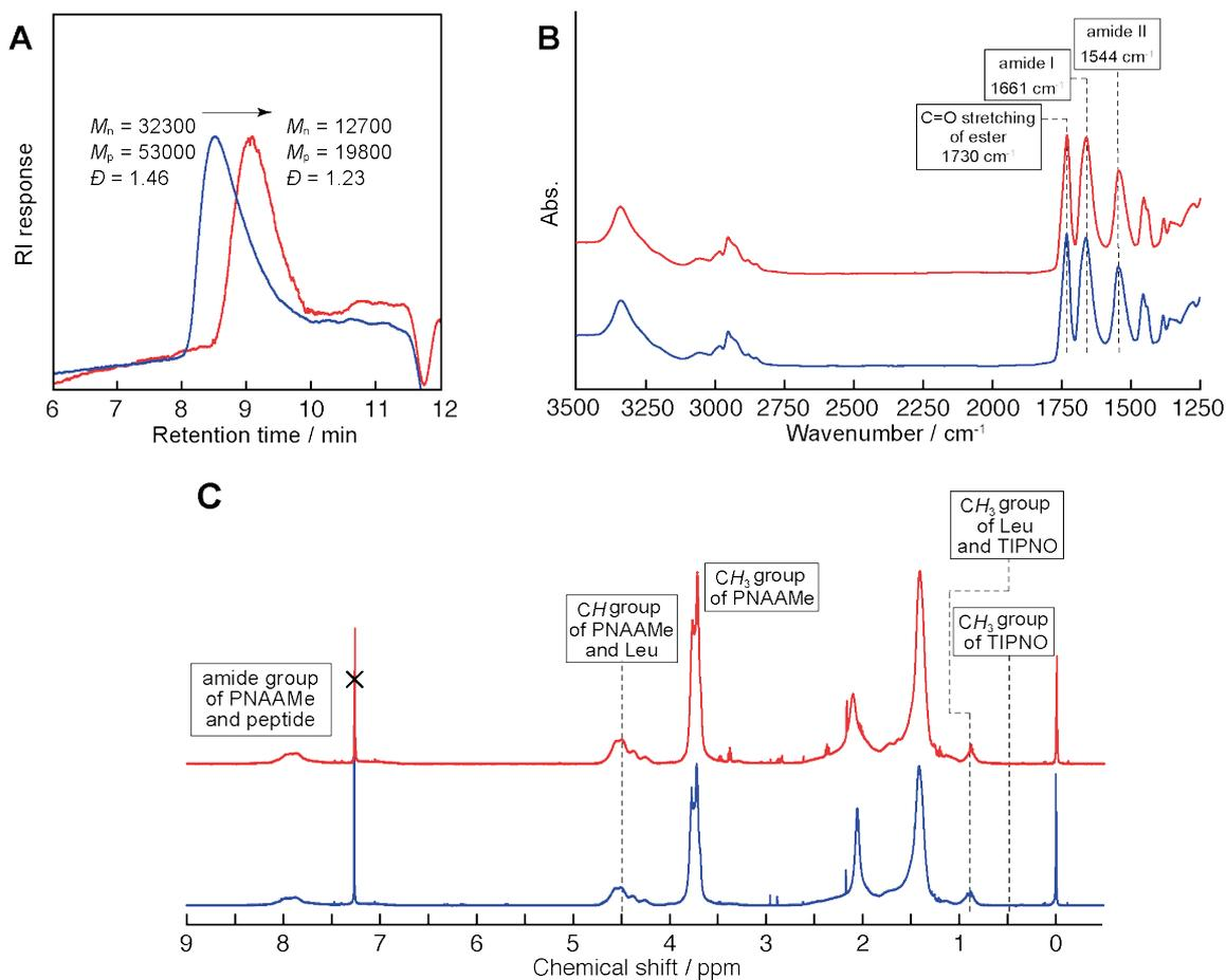
**Figure S15. Characterization of the multiblock P6.** **A.** SEC traces (THF, 40 °C) of the multiblock **P6** obtained before (blue) and after (red) fragmentation showing a clear shift towards a lower molecular weight. **B.** Transmission-FTIR spectra of **P6** (blue) and fragmented **P6** (red) casted from the  $\text{CHCl}_3$  solution onto a  $\text{CaF}_2$  plate. **C.**  $^1\text{H}$  NMR spectra of **P6** (blue) and fragmented **P6** (red) in  $\text{CDCl}_3$  at 25°C.
