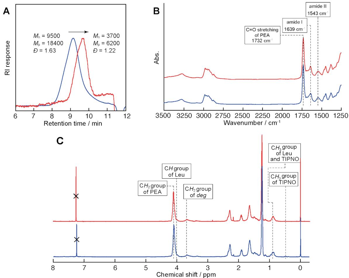
**Figure S18. Characterization of the multiblock P8.** **A.** SEC traces (THF, 40 °C) of the multiblock **P8** obtained before (blue) and after (red) fragmentation showing a clear shift towards a lower molecular weight. **B.** Transmission-FTIR spectra of **P8** (blue) and fragmented **P8** (red) casted from the  $\text{CHCl}_3$  solution onto a  $\text{CaF}_2$  plate. **C.**  $^1\text{H}$  NMR spectra of **P8** (blue) and fragmented **P8** (red) in  $\text{CDCl}_3$  at 25°C.
