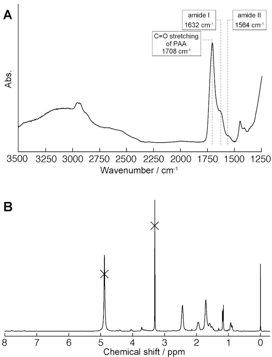
**Figure S17.** **A.** Transmission-FTIR spectrum of **P7** obtained after treatment with TFA casted from the MeOH solution onto a  $\text{CaF}_2$  plate. **B.**  $^1\text{H}$  NMR spectra of **P7** obtained after treatment TFA in  $\text{CD}_3\text{OD}$  at  $25^\circ\text{C}$ .
