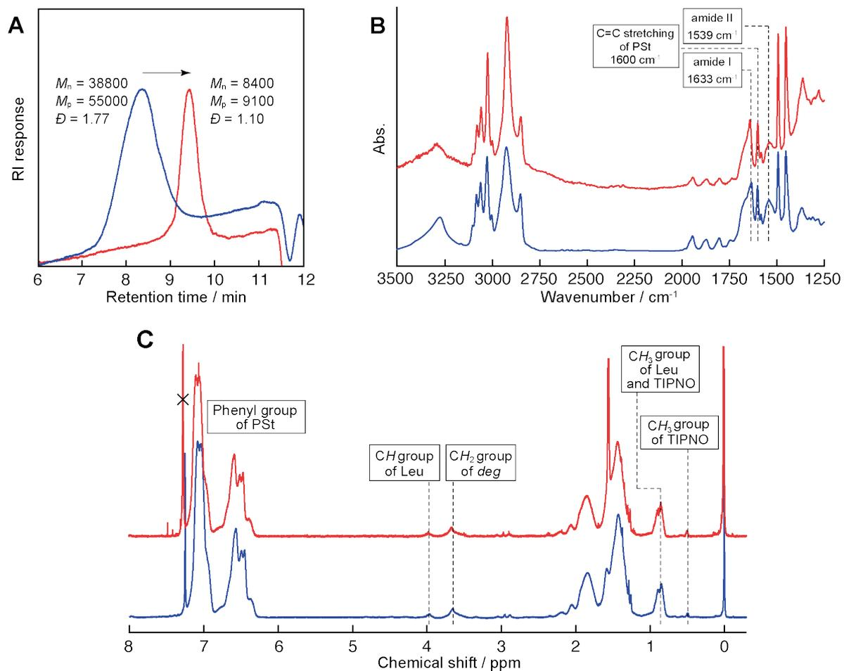
**Figure S20. Characterization of the multiblock P10.** **A.** SEC traces (THF, 40 °C) of the multiblock **P10** obtained before (blue) and after (red) fragmentation showing a clear shift towards a lower molecular weight. **B.** Transmission-FTIR spectra of **P10** (blue) and fragmented **P10** (red) casted from the  $\text{CHCl}_3$  solution onto a  $\text{CaF}_2$  plate. **C.**  $^1\text{H}$  NMR spectra of **P10** (blue) and fragmented **P10** (red) in  $\text{CDCl}_3$  at 25°C.
