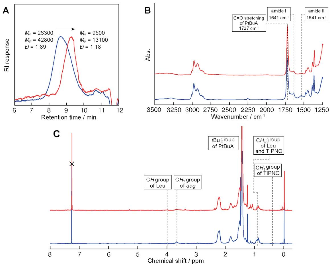
**Figure S16. Characterization of the multiblock P7.** **A.** SEC traces (THF, 40 °C) of the multiblock **P7** obtained before (blue) and after (red) fragmentation showing a clear shift towards a lower molecular weight. **B.** Transmission-FTIR spectra of **P7** (blue) and fragmented **P7** (red) casted from the  $\text{CHCl}_3$  solution onto a  $\text{CaF}_2$  plate. **C.**  $^1\text{H}$  NMR spectra of **P7** (blue) and fragmented **P7** (red) in  $\text{CDCl}_3$  at 25°C.
