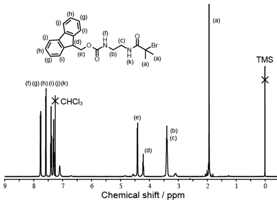
**Figure S3.**  $^1\text{H}$  NMR spectrum of Fmoc-EDA-Br (**2**) in  $\text{CDCl}_3$  at  $25^\circ\text{C}$ .
