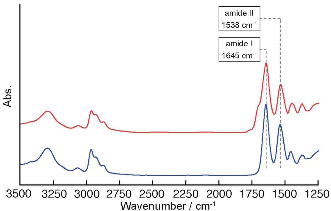
**Figure S10.** Transmission-FTIR spectra of **P2** (blue) and fragmented **P2** (red) casted from the  $\text{CHCl}_3$  solution onto a  $\text{CaF}_2$  plate.
