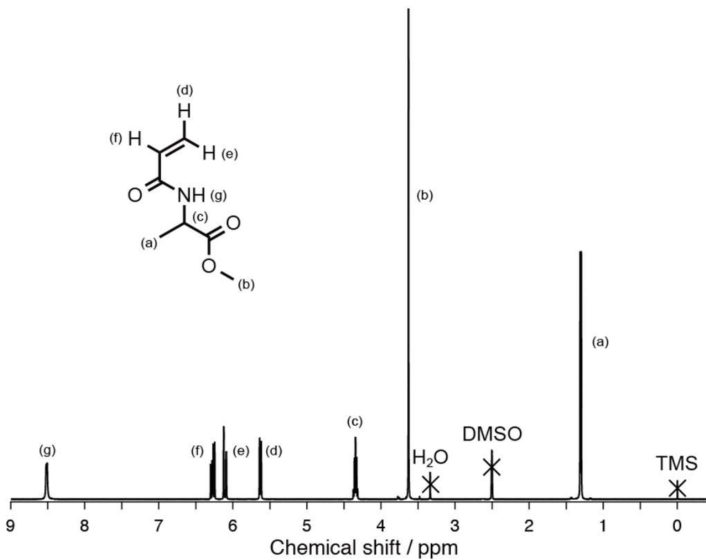
**Figure S21.**  $^1\text{H}$  NMR spectrum of NAAME in  $\text{DMSO-}d_6$  at  $25^\circ\text{C}$ .
