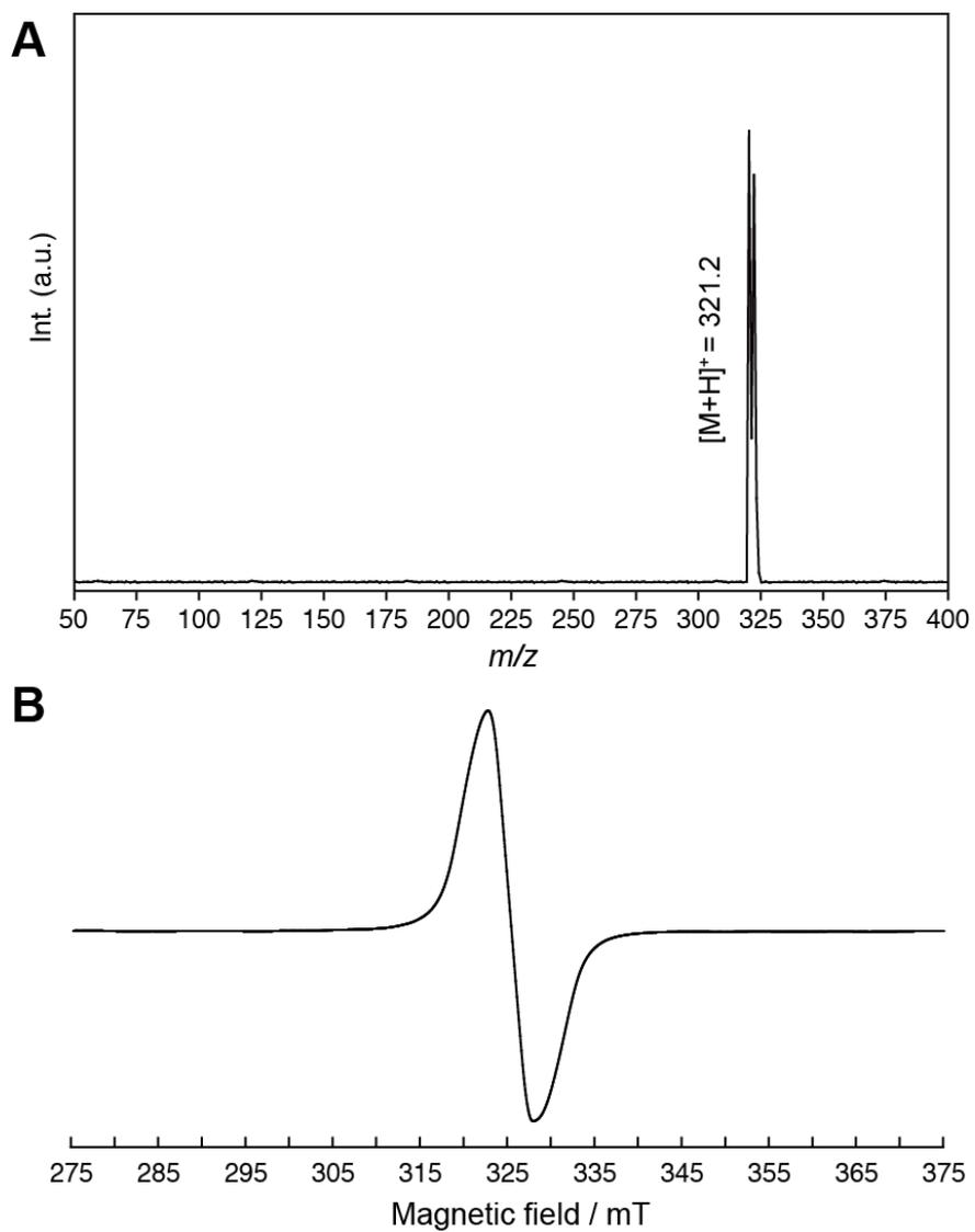
**Figure S6.** **A.** DART MS spectrum of TIPNO-COOtBu, free radical (**5**). Ionization temperature: 300°C. **B.** ESR spectrum of **5** in CHCl<sub>3</sub> at -196°C.
