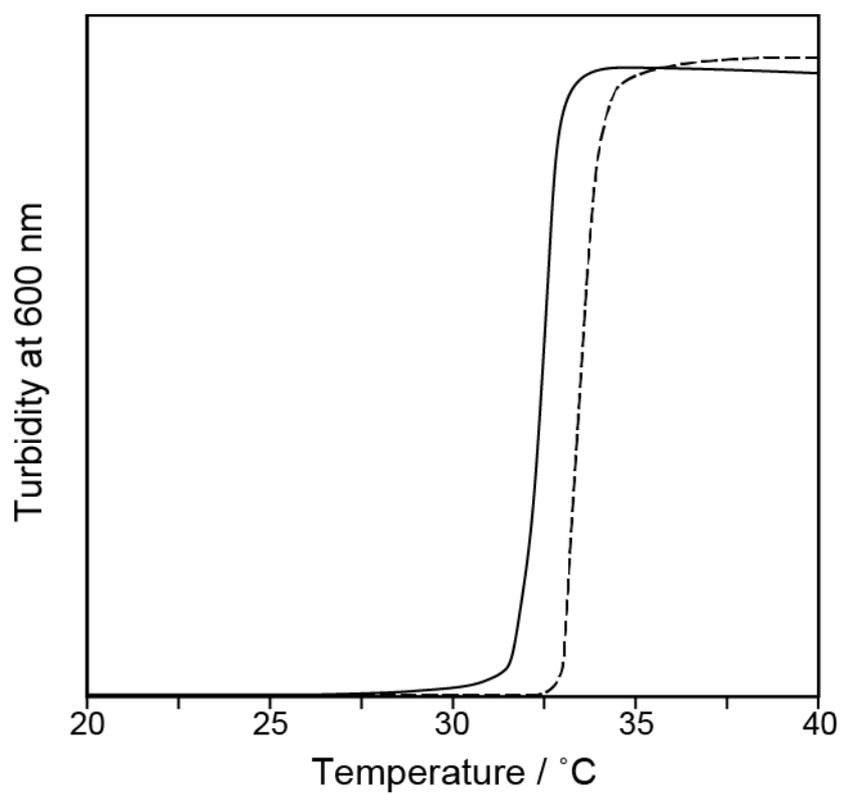
**Figure S9.** Turbidity measurements of **P5** (solid line) and PNIPAM homopolymer ( $M_n=74000 \text{ g mol}^{-1}$ ) (dashed line) in water at 600 nm. [Polymer]=1 wt%.
