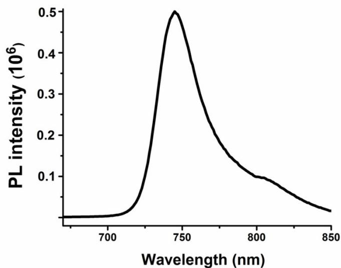
**Figure S14.** The emission spectra of fluorophore BOD-alky in DMSO, concentration =  $5 \mu\text{g/mL}$ ,  $\lambda_{\text{ex}}=695 \text{ nm}$ ,  $\lambda_{\text{em}}=745 \text{ nm}$ .
