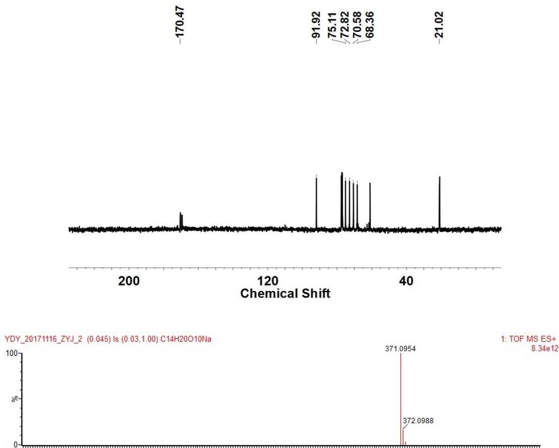
**Figure S3.**  $^1\text{H}$  NMR and  $^{13}\text{C}$  NMR spectra of the GTA in  $\text{CDCl}_3$  and HRMS.
