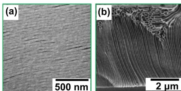
Fig. S5 SEM micrographs of BBCPs self-assembled in bulk (a:  $(g\text{PDMS})_{122}\text{-}b\text{-(gPS)}_{93}$ ; b:  $(g\text{PDMS})_{97}\text{-}b\text{-(gPS)}_{82}$ )
