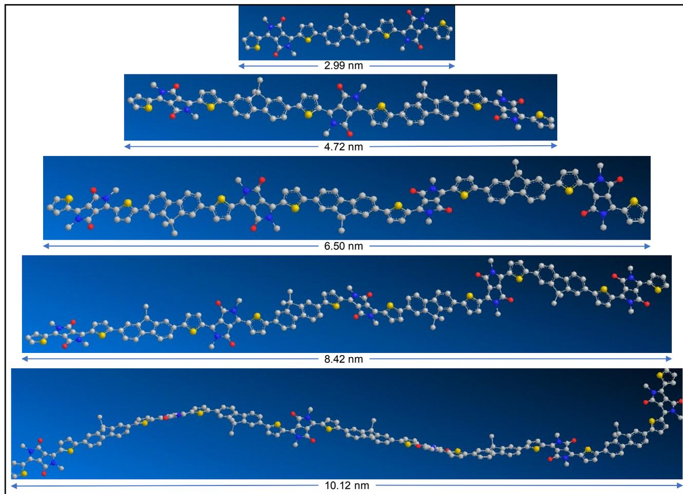
**Fig. S5** DFT-optimized geometries of oligomers **Os1~5** (the alkyl chains replaced by methyl groups).
