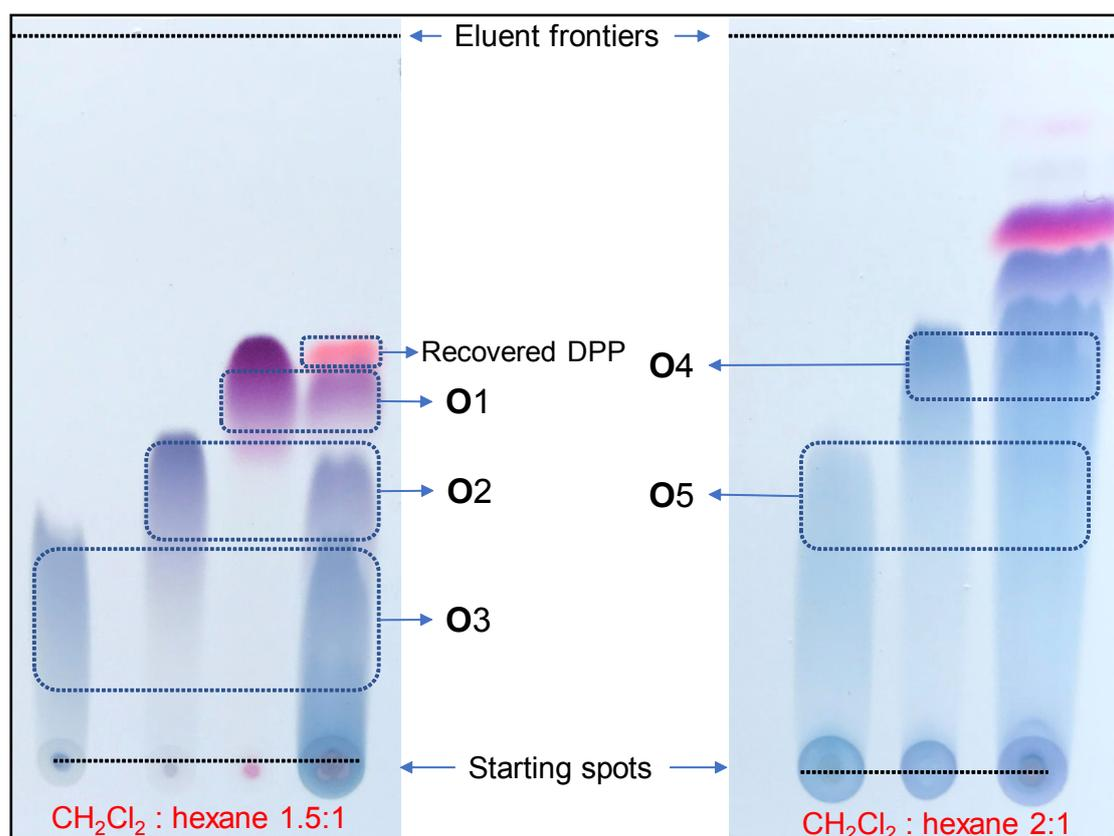
**Fig. S1** TLC analysis of the direct arylated coupling between DPP and 2,7-dibromo-9,9-dioctylfluorene in molar ratio of 1.4/1 using  $\text{CH}_2\text{Cl}_2$  : hexane (1.5:1 and 2:1 respectively, v/v) as eluent. The starting spots on each TLC plate involved the reaction mixture and the corresponding purified oligomers.
