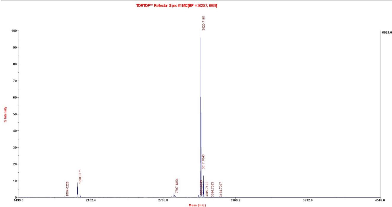
Fig. S16 MALDI-TOF MS of O<sub>2</sub>, calcd. 3020.88, found 3020.72.
