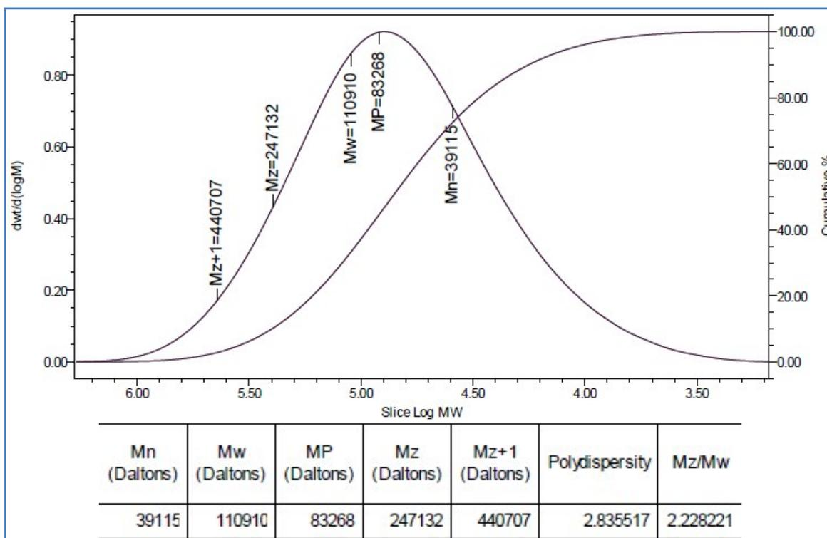
**Fig. S3** GPC profile of **P1** and the corresponding list of the obtained data.
