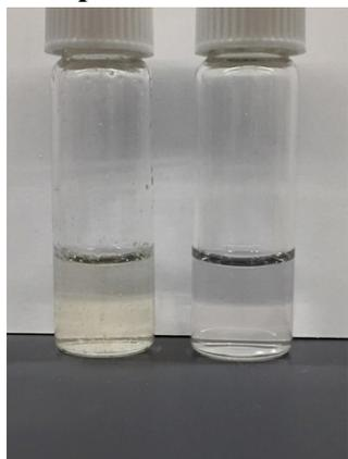
Figure S2. Picture of left) Solvent switch of **20-20** from DMF to water at 5 wt% solids, right) ROMPISA formulation of **20-20** at 5 wt% solids. Note the polymer precipitates in the left vial.
