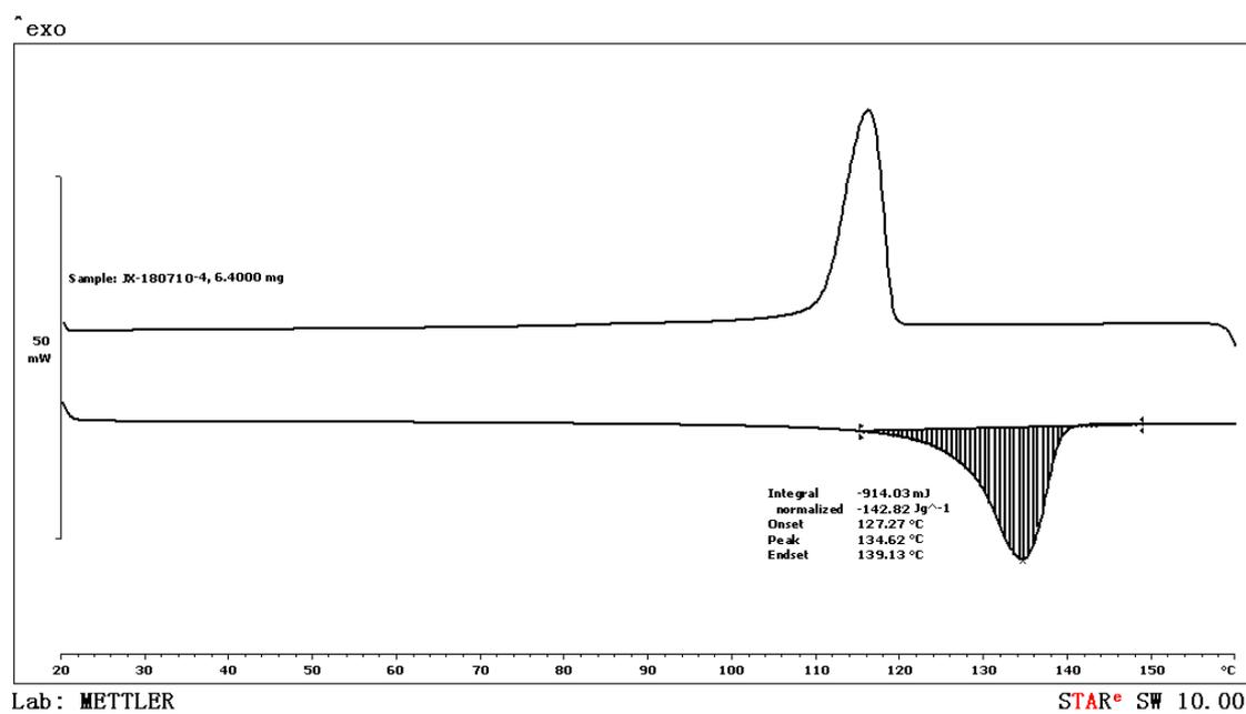
**Figure S79.** DSC data of the polymer from table 1, entry 10.
