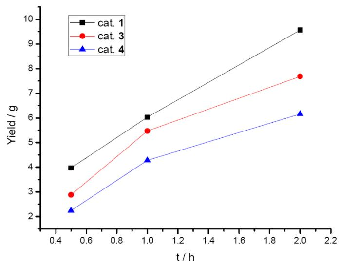
**Figure S90.** Time-dependence studies of catalysts towards ethylene polymerization.
