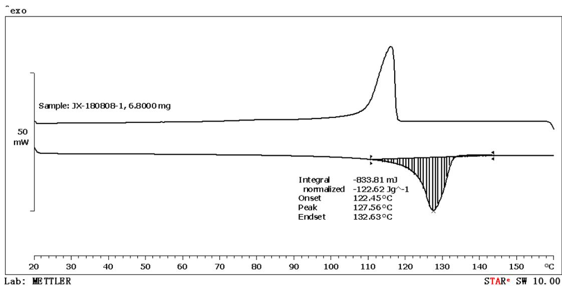
**Figure S81.** DSC data of the polymer from table 2, entry 3.
