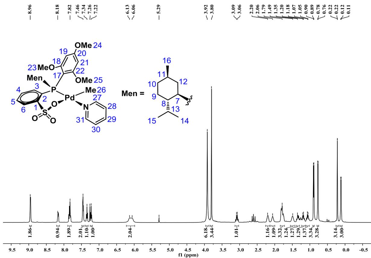
**Figure S24.**  $^1\text{H}$  NMR spectrum (500 MHz, 298 K,  $\text{CDCl}_3$ ) of complex **4**.
