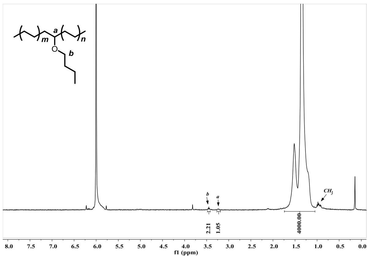
**Figure S49.**  $^1\text{H NMR}$  spectrum (400 MHz,  $\text{C}_2\text{D}_2\text{Cl}_4$ , 100 °C) of the E-BVE copolymer from table 2, entry 16.
