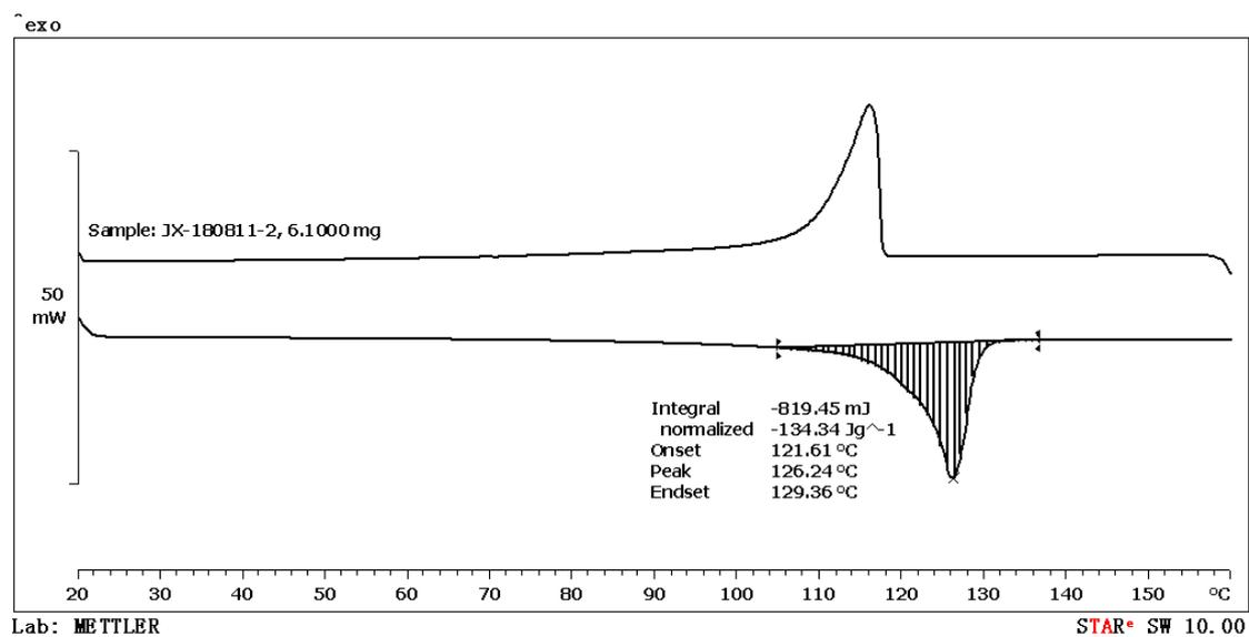
**Figure S86.** DSC data of the polymer from table 2, entry 13.
