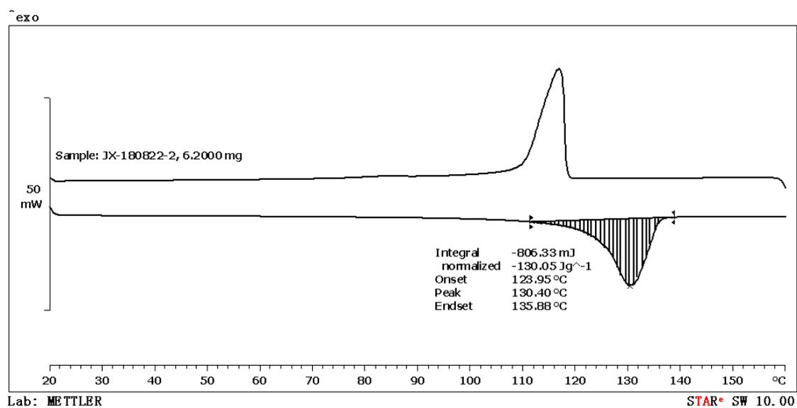
**Figure S87.** DSC data of the polymer from table 2, entry 16.
