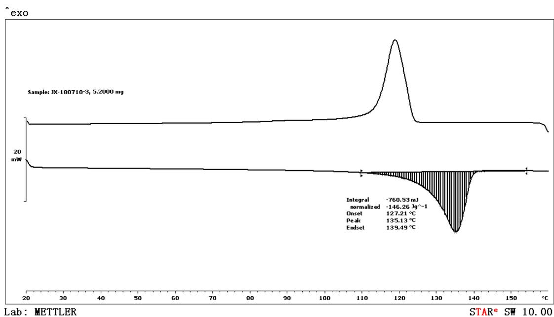
**Figure S77.** DSC data of the polymer from table 1, entry 8.
