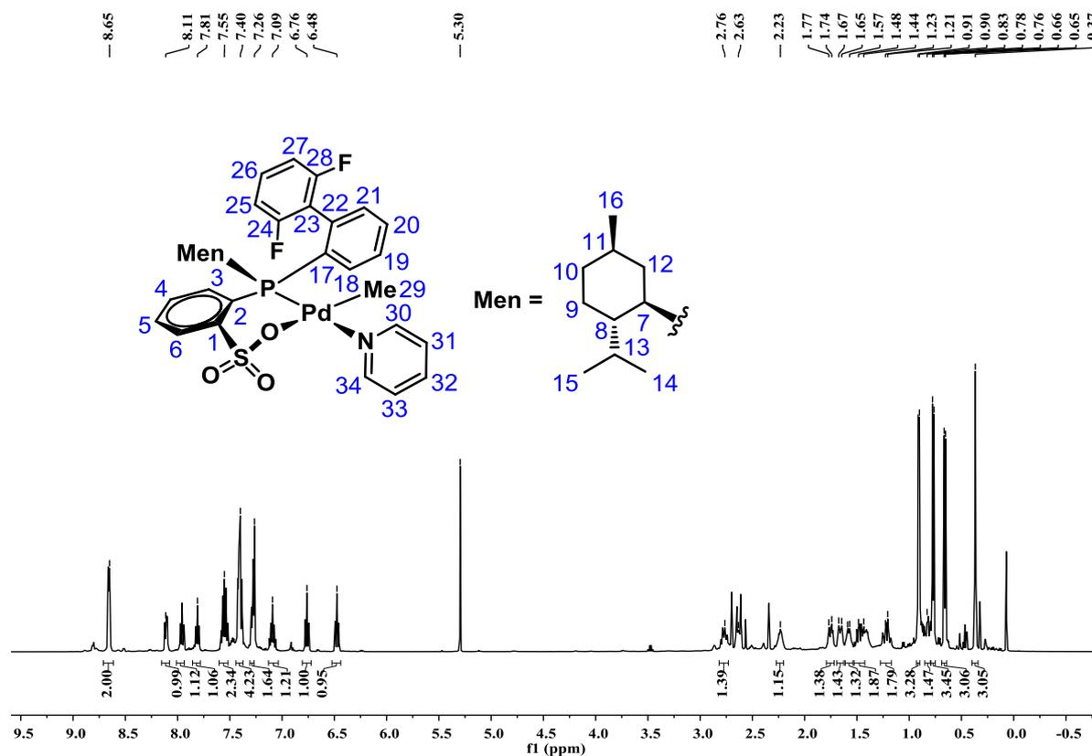
Figure S20.  $^1\text{H}$  NMR spectrum (500 MHz, 298 K,  $\text{CDCl}_3$ ) of complex **3**.
