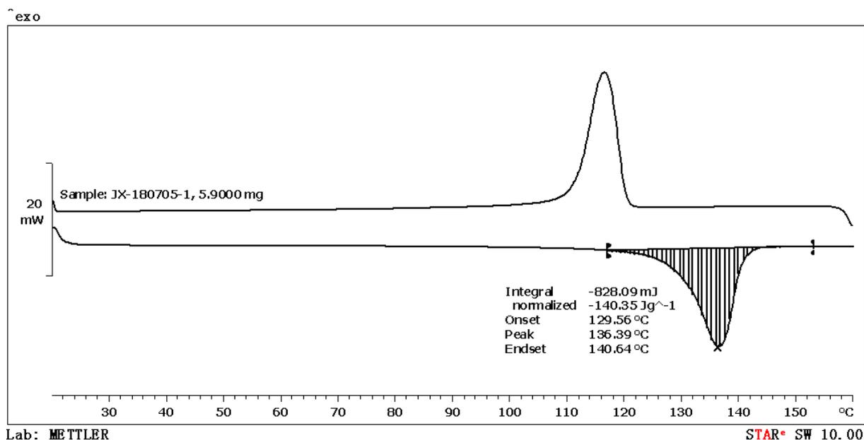
**Figure S72.** DSC data of the polymer from table 1, entry 1.
