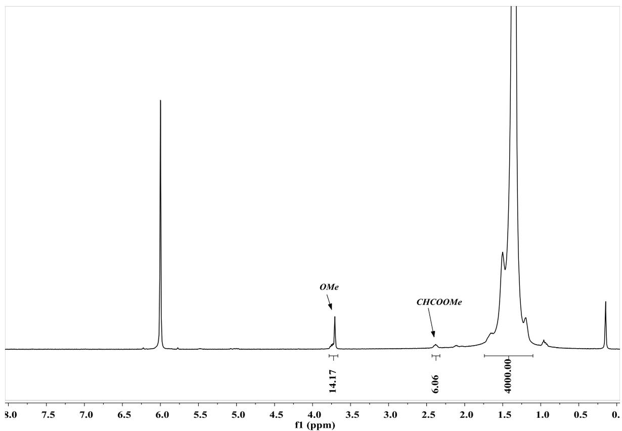
**Figure S36.** <sup>1</sup>H NMR spectrum (400 MHz, C<sub>2</sub>D<sub>2</sub>Cl<sub>4</sub>, 100 °C) of the E-MA copolymer from table 2, entry 2.
