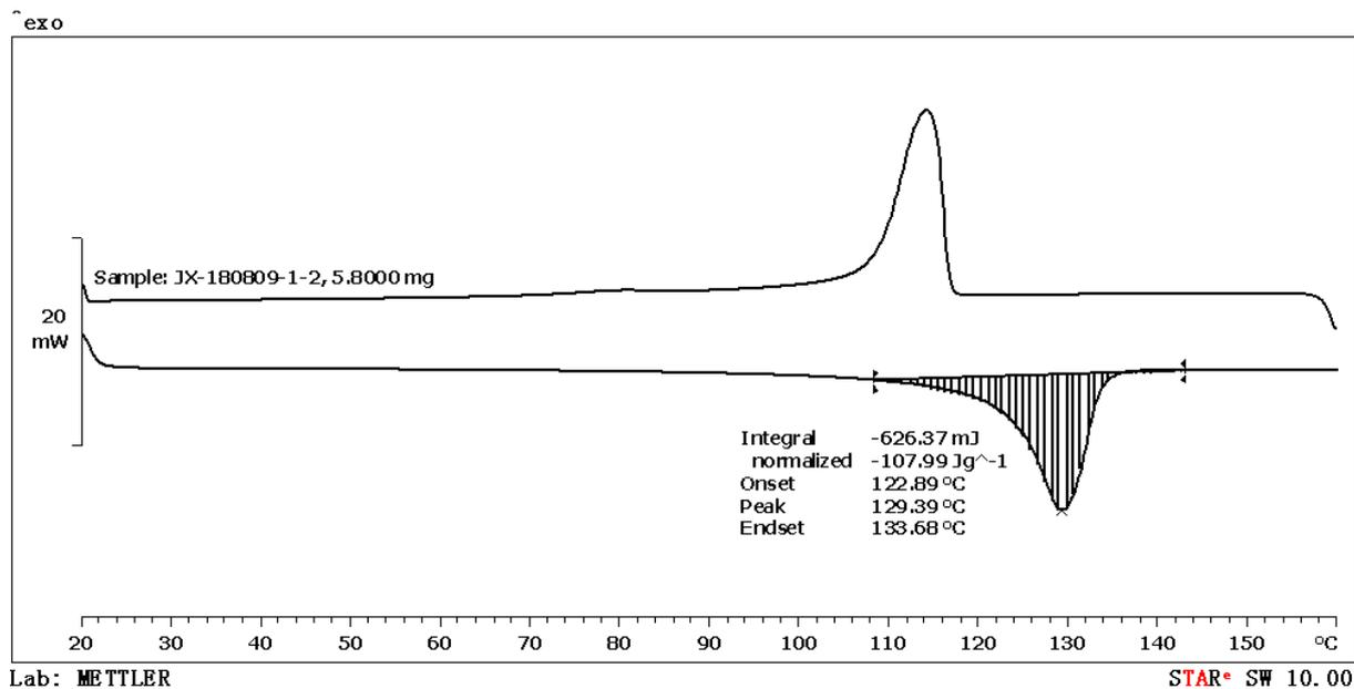
**Figure S80.** DSC data of the polymer from table 2, entry 2.
