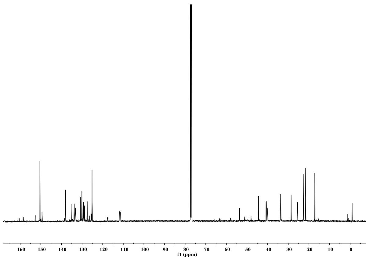
**Figure S21.**  $^{13}\text{C}\{^1\text{H}\}$  NMR spectrum (125 MHz, 298 K,  $\text{CDCl}_3$ ) of complex **3**.
