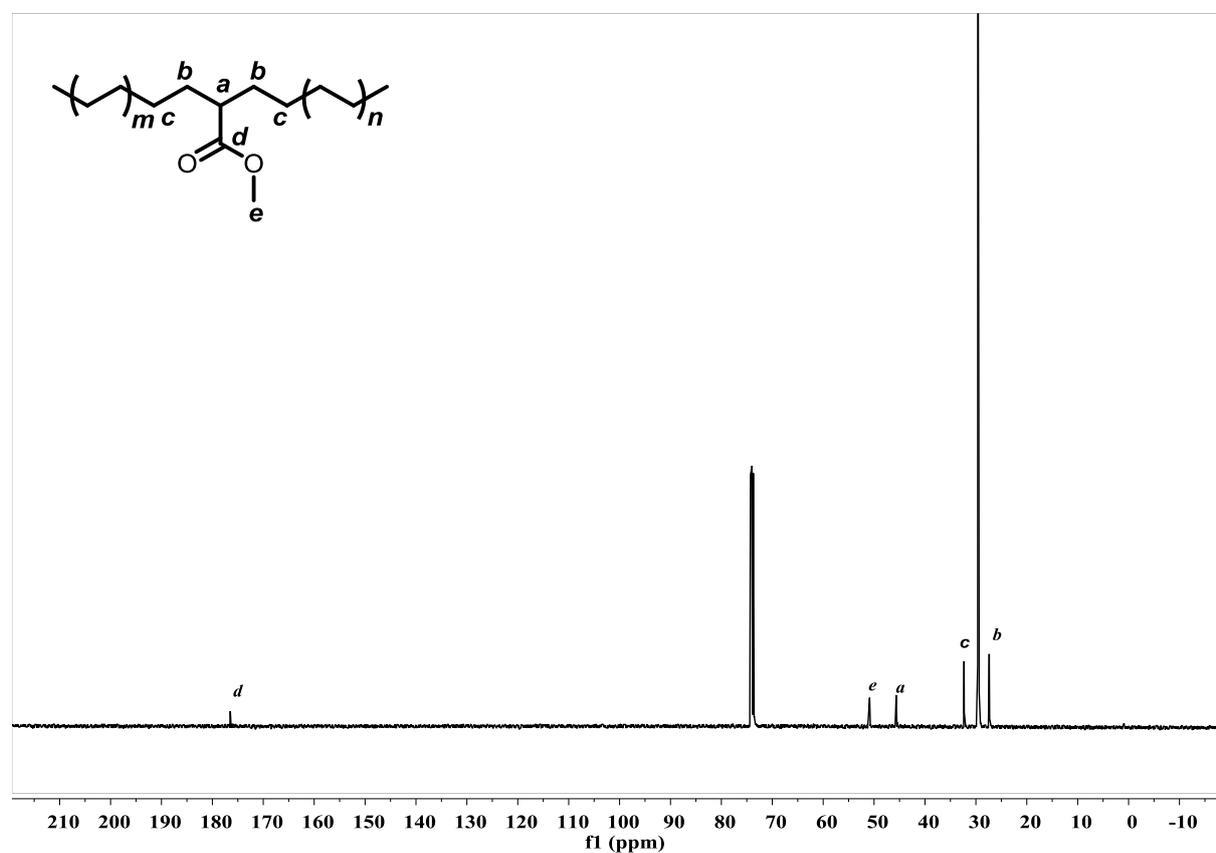
**Figure S52.**  $^{13}\text{C}$  NMR spectrum (400 MHz,  $\text{C}_2\text{D}_2\text{Cl}_4$ , 100  $^\circ\text{C}$ ) of the E-MA polymer from table 2, entry 7.
