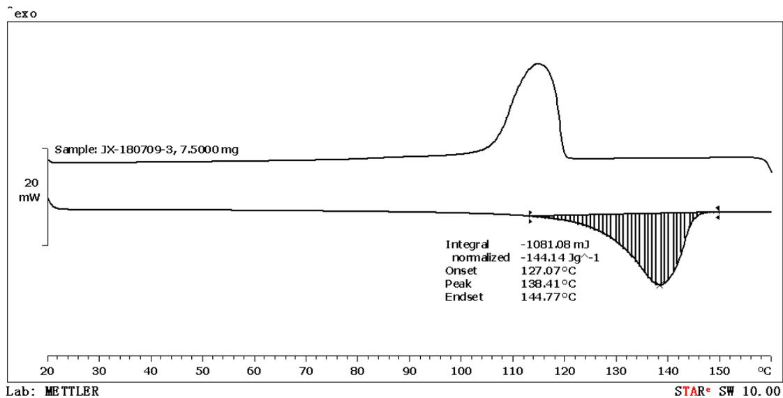
**Figure S76.** DSC data of the polymer from table 1, entry 7.
