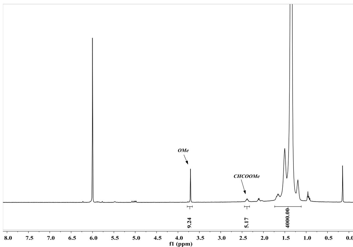
**Figure S35.** <sup>1</sup>H NMR spectrum (400 MHz, C<sub>2</sub>D<sub>2</sub>Cl<sub>4</sub>, 100 °C) of the E-MA copolymer from table 2, entry 1.
