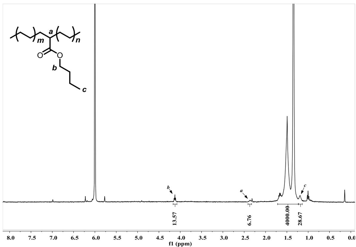
**Figure S43.**  $^1\text{H}$  NMR spectrum (400 MHz,  $\text{C}_2\text{D}_2\text{Cl}_4$ , 100  $^\circ\text{C}$ ) of the E-*n*BuA copolymer from table 2, entry 9.
