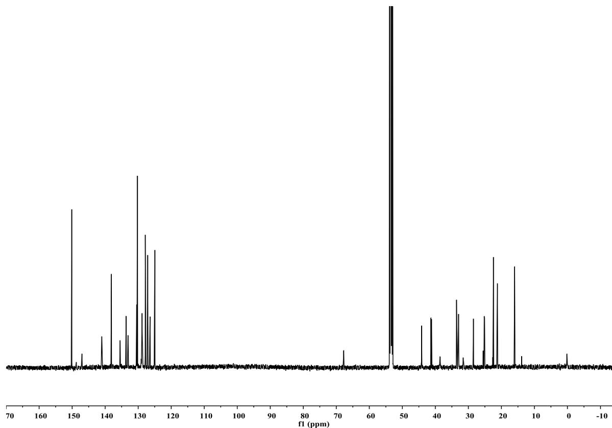
**Figure S18.**  $^{13}\text{C}\{^1\text{H}\}$  NMR spectrum (125 MHz, 298 K,  $\text{CD}_2\text{Cl}_2$ ) of complex 2.
