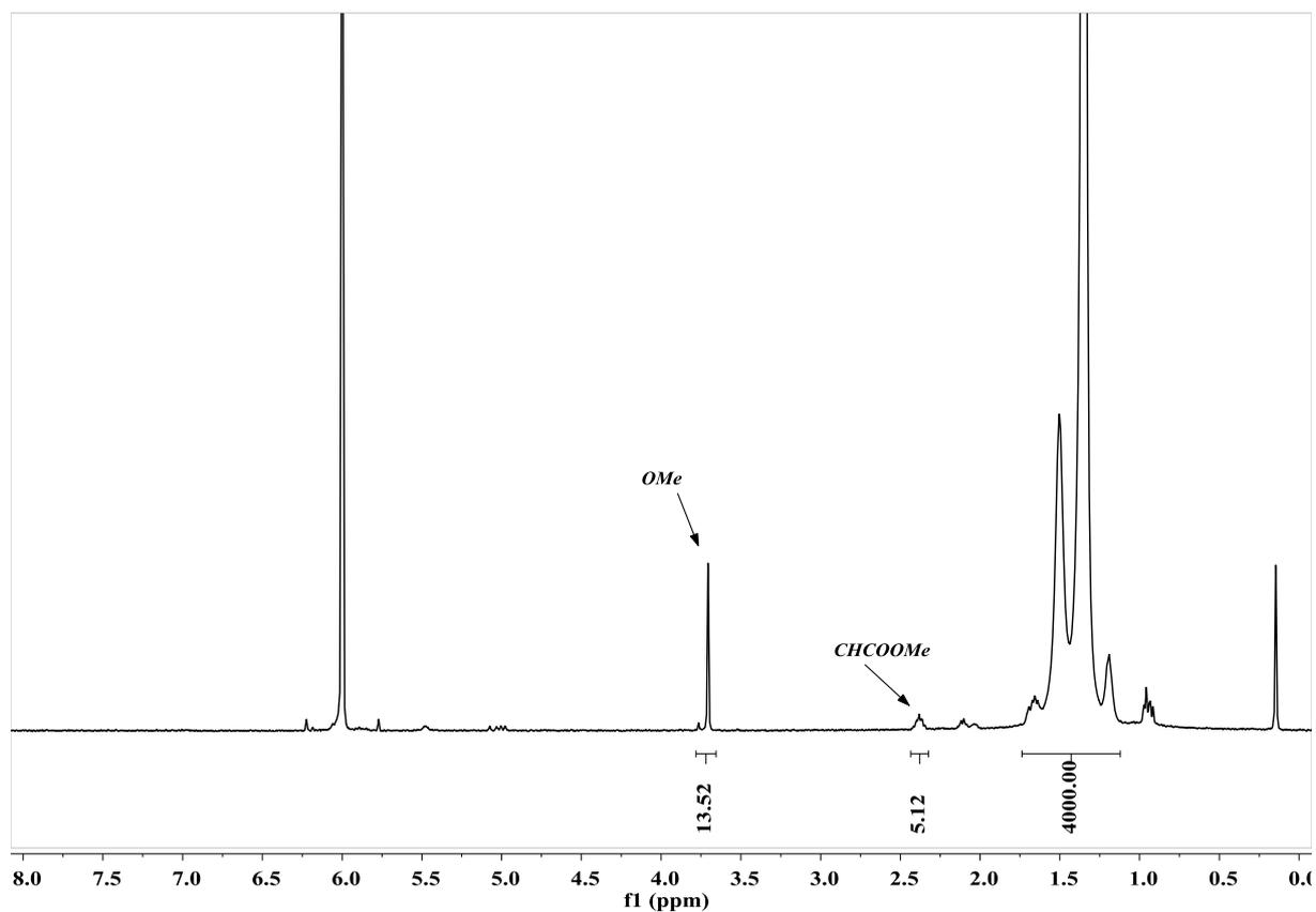
**Figure S37.** <sup>1</sup>H NMR spectrum (400 MHz, C<sub>2</sub>D<sub>2</sub>Cl<sub>4</sub>, 100 °C) of the E-MA copolymer from table 2, entry 3.
