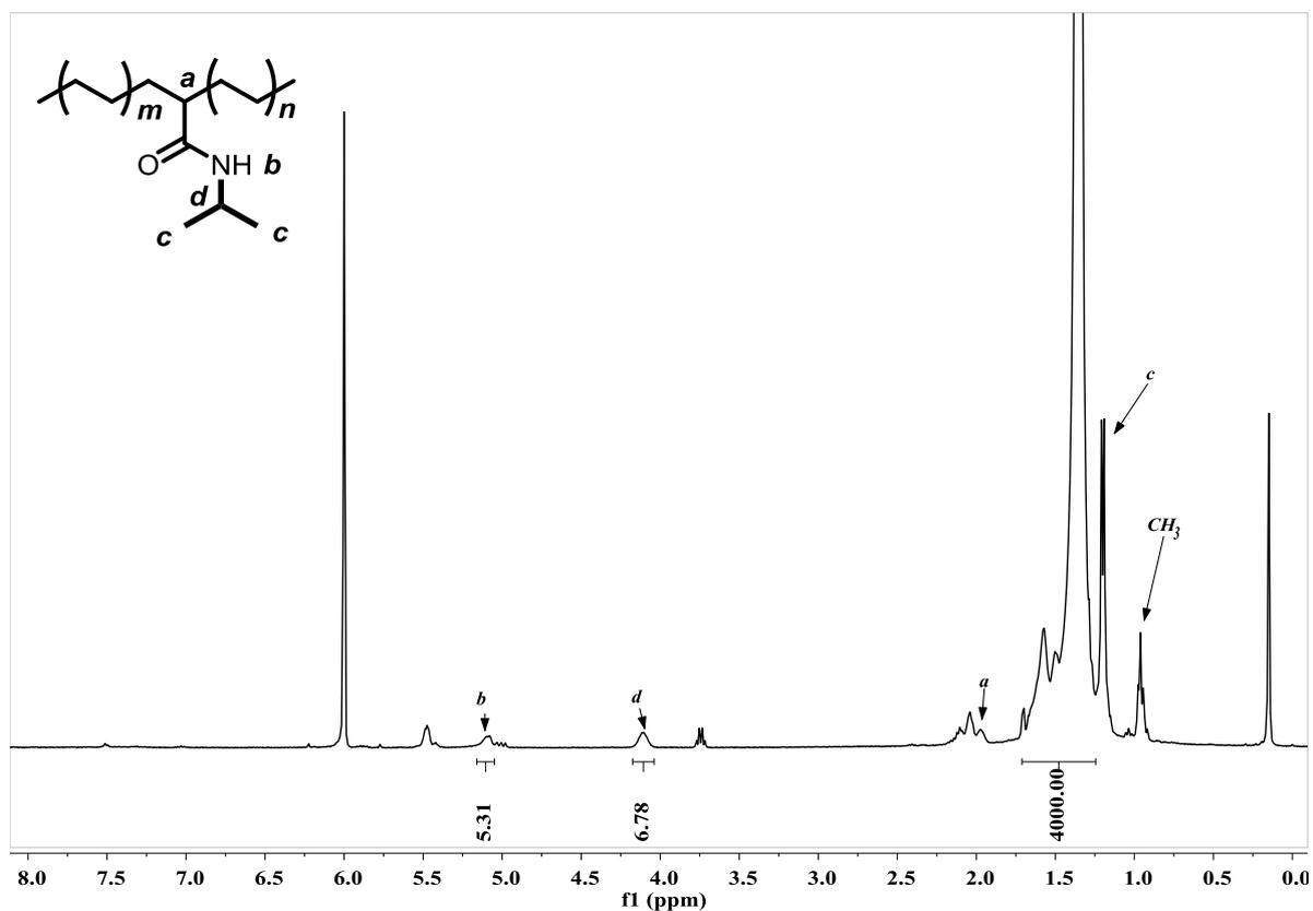
**Figure S46.** <sup>1</sup>H NMR spectrum (400 MHz, C<sub>2</sub>D<sub>2</sub>Cl<sub>4</sub>, 100 °C) of the E-NIPAA copolymer from table 2, entry 13.
