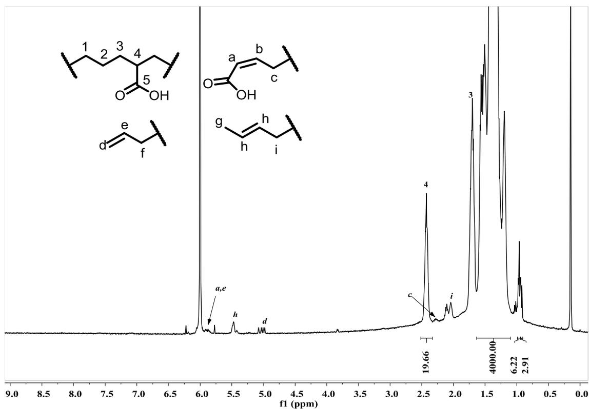
**Figure S45.** <sup>1</sup>H NMR spectrum (400 MHz, C<sub>2</sub>D<sub>2</sub>Cl<sub>4</sub>, 100 °C) of the E-AA copolymer from table 2, entry 12.
