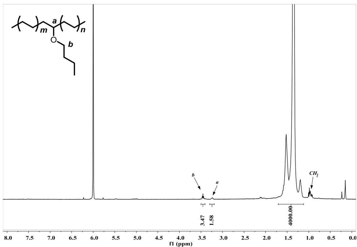
**Figure S48.**  $^1\text{H}$  NMR spectrum (400 MHz,  $\text{C}_2\text{D}_2\text{Cl}_4$ , 100  $^\circ\text{C}$ ) of the E-BVE copolymer from table 2, entry 15.
