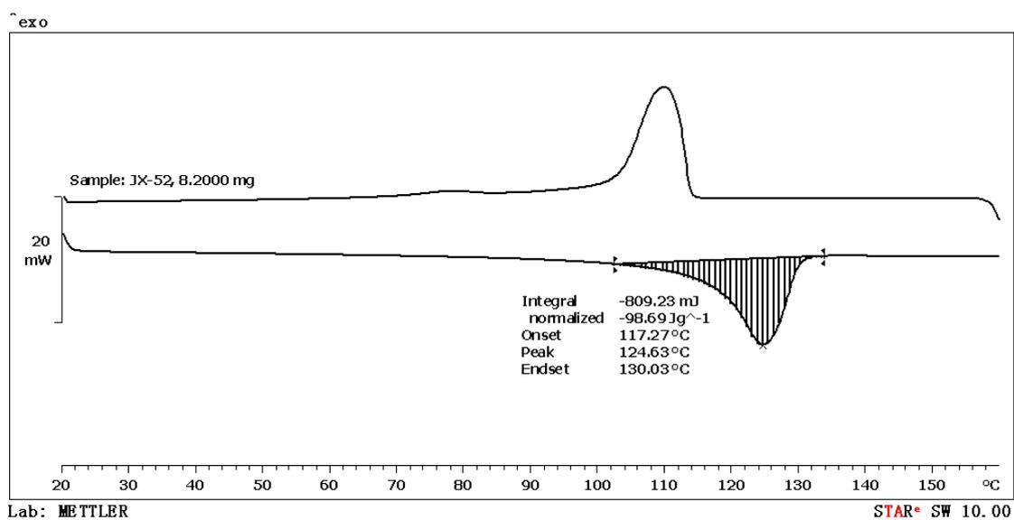
**Figure S83.** DSC data of the polymer from table 2, entry 9.
