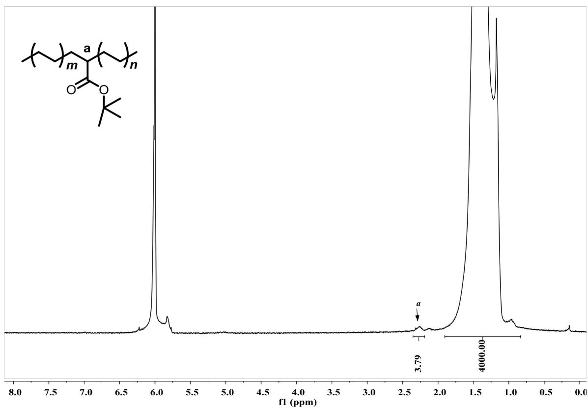
**Figure S44.**  $^1\text{H}$  NMR spectrum (400 MHz,  $\text{C}_2\text{D}_2\text{Cl}_4$ , 100  $^\circ\text{C}$ ) of the E-*t*BuA copolymer from table 2, entry 10.
