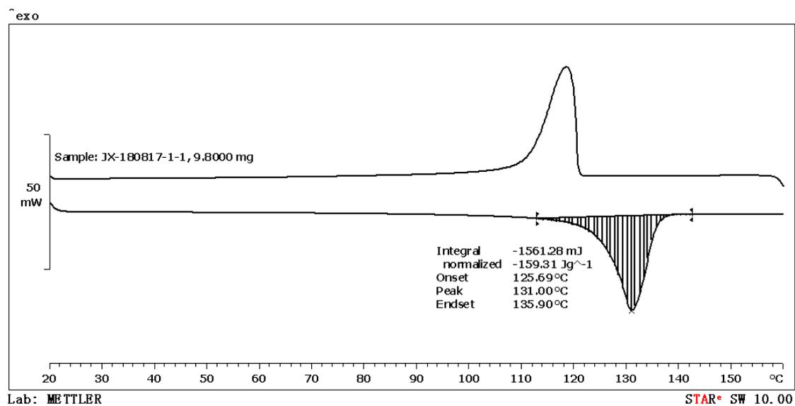
**Figure S88.** DSC data of the polymer from table 2, entry 18.
