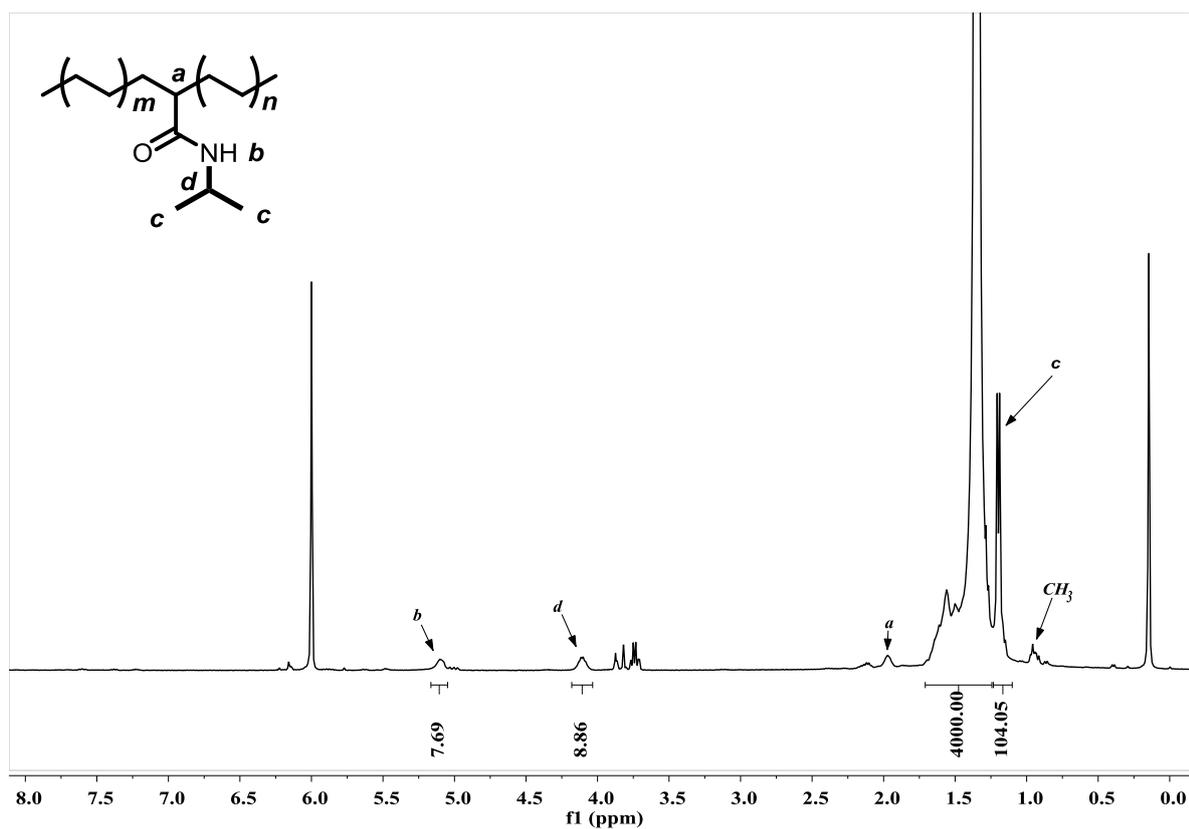
**Figure S47.**  $^1\text{H}$  NMR spectrum (400 MHz,  $\text{C}_2\text{D}_2\text{Cl}_4$ , 100  $^\circ\text{C}$ ) of the E-NIPAA copolymer from table 2, entry 14.
