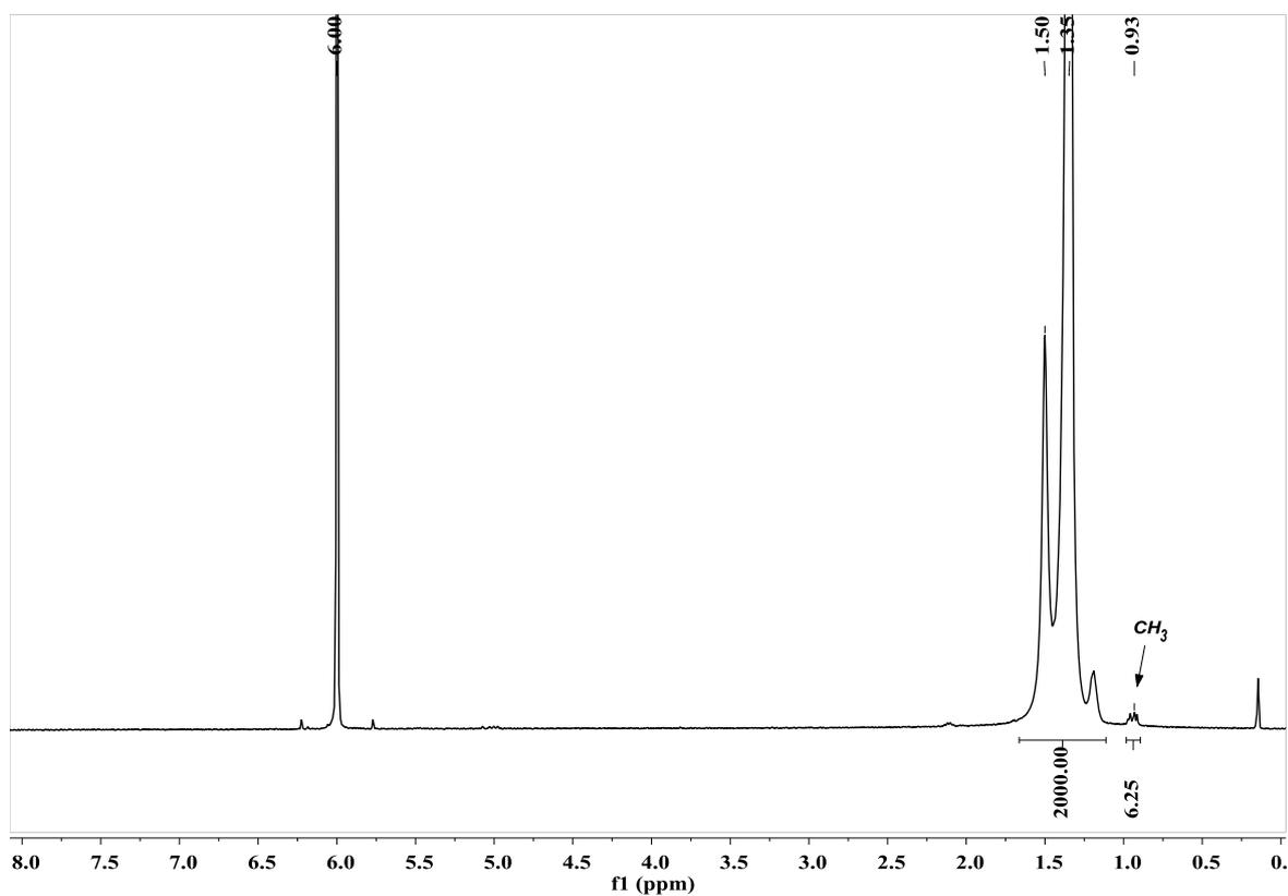
**Figure S34.**  $^1\text{H}$  NMR spectrum (400 MHz,  $\text{C}_2\text{D}_2\text{Cl}_4$ , 100  $^\circ\text{C}$ ) of the polymer from table 1, entry 10.
