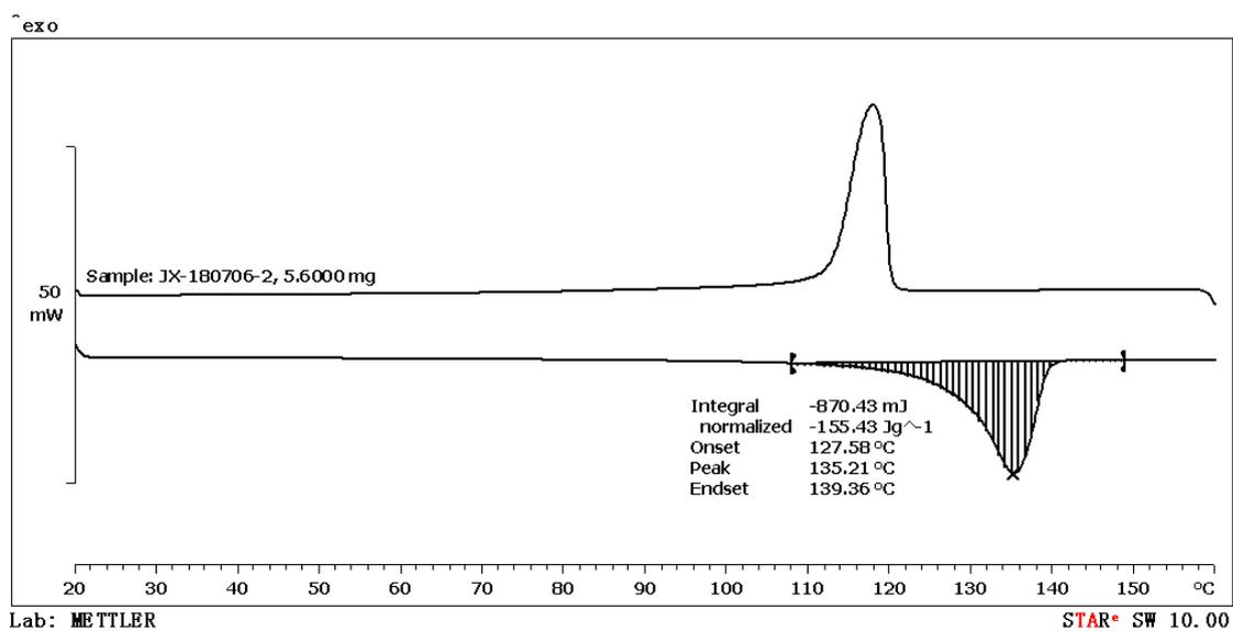
**Figure S73.** DSC data of the polymer from table 1, entry 3.
