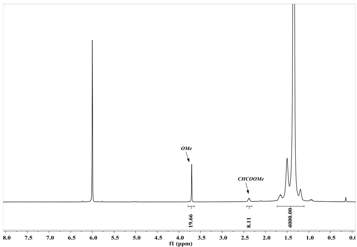
**Figure S42.** <sup>1</sup>H NMR spectrum (400 MHz, C<sub>2</sub>D<sub>2</sub>Cl<sub>4</sub>, 100 °C) of the E-MA copolymer from table 2, entry 8.
