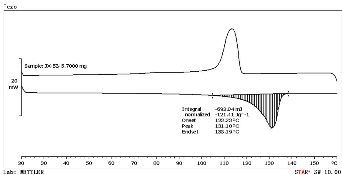
**Figure S84.** DSC data of the polymer from table 2, entry 10.
