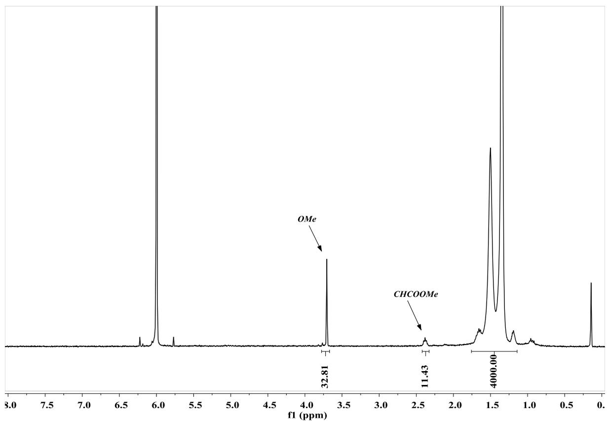
**Figure S38.** <sup>1</sup>H NMR spectrum (400 MHz, C<sub>2</sub>D<sub>2</sub>Cl<sub>4</sub>, 100 °C) of the E-MA copolymer from table 2, entry 4.
