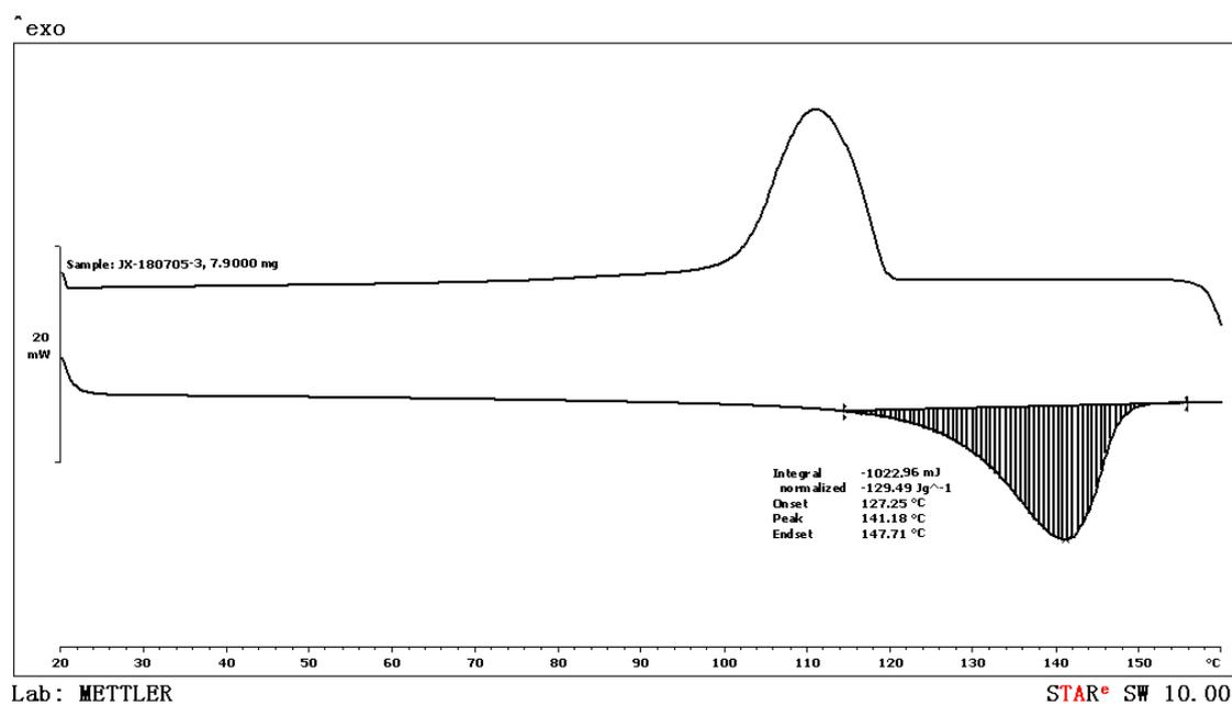
**Figure S75.** DSC data of the polymer from table 1, entry 6.
