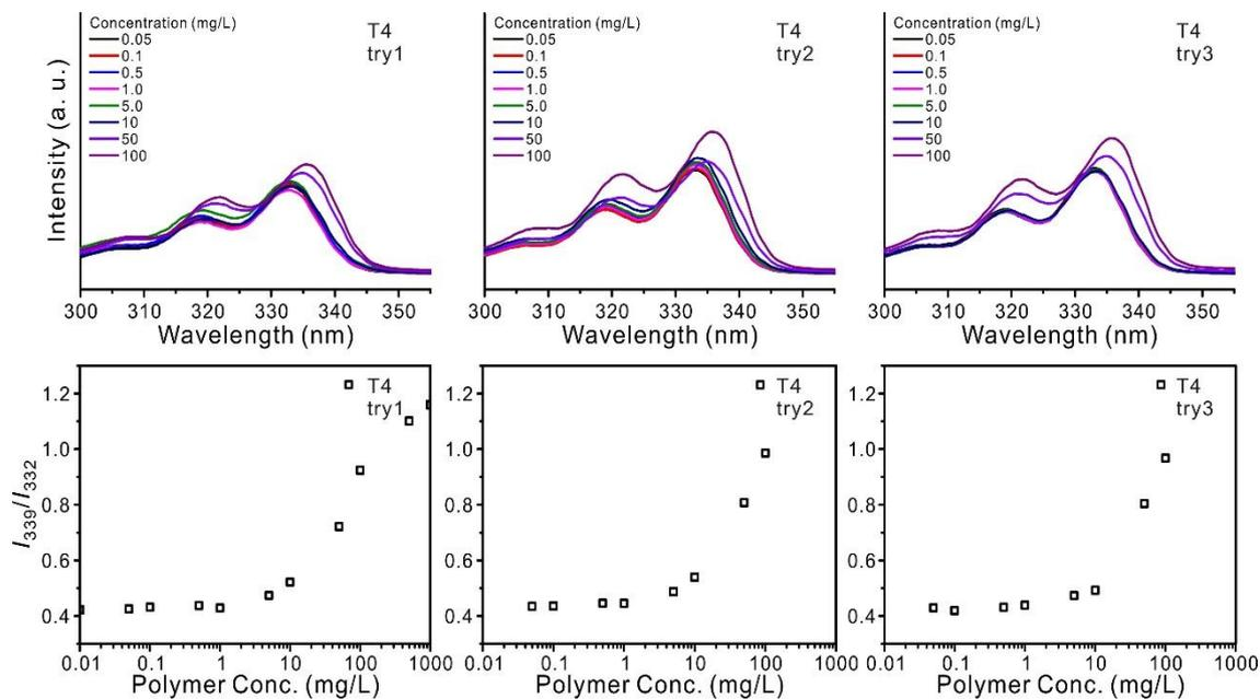
**Fig. S7** Excitation spectra of pyrene in aqueous solution and determination of CMC for PEG<sub>114</sub>-*b*-P(EEGE-*co*-TGE)<sub>0/27</sub> (**T4**) micelles ( $\lambda_{em} = 372$  nm). CMC was calculated *via* measurements of  $I_{339}/I_{332}$  as a function of polymer concentration using the fluorescence excitation spectra of pyrene.
