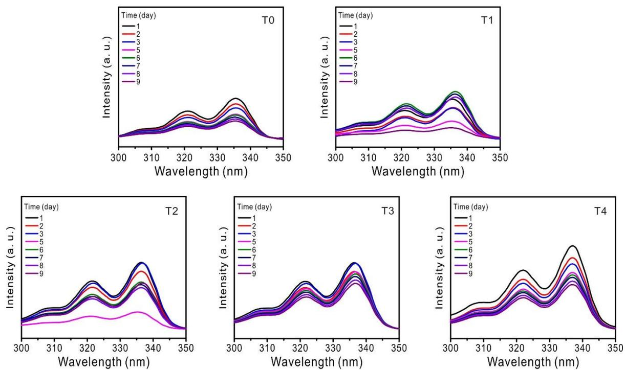
**Fig. S11** Changes in excitation spectra of pyrene encapsulated by **T0 – T4** micelles in pH 7.4 condition. The concentrations of all polymers are fixed to 0.10 mg/mL.
