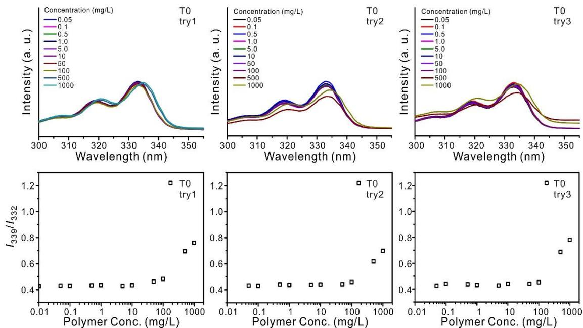
**Fig. S3** Excitation spectra of pyrene in aqueous solution and determination of CMC for PEG<sub>114</sub>-*b*-P(EEGE-*co*-TGE)<sub>27/0</sub> (**T0**) micelles ( $\lambda_{em} = 372$  nm). CMC was calculated *via* measurements of  $I_{339}/I_{332}$  as a function of polymer concentration using the fluorescence excitation spectra of pyrene.
