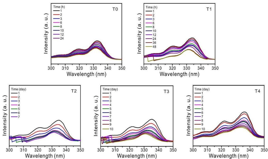
**Fig. S12** Changes in excitation spectra of pyrene encapsulated by **T0 – T4** micelles in pH 5.0 condition. The concentrations of all polymers are fixed to 0.10 mg/mL.
