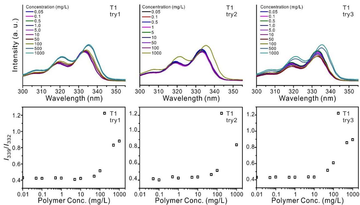
**Fig. S4** Excitation spectra of pyrene in aqueous solution and determination of CMC for PEG<sub>114</sub>-*b*-P(EEGE-*co*-TGE)<sub>21/6</sub> (T1) micelles ( $\lambda_{em} = 372$  nm). CMC was calculated *via* measurements of  $I_{339}/I_{332}$  as a function of polymer concentration using the fluorescence excitation spectra of pyrene.
