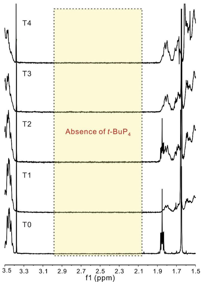
**Fig. S16** Expanded <sup>1</sup>H NMR spectra of PEG<sub>114</sub>-*b*-P(EEGE-*co*-TGE)<sub>*m/n*</sub> copolymers (**T0**–**T4**), displaying the clear disappearance of the residual phosphazene base, *t*-BuP<sub>4</sub>.
