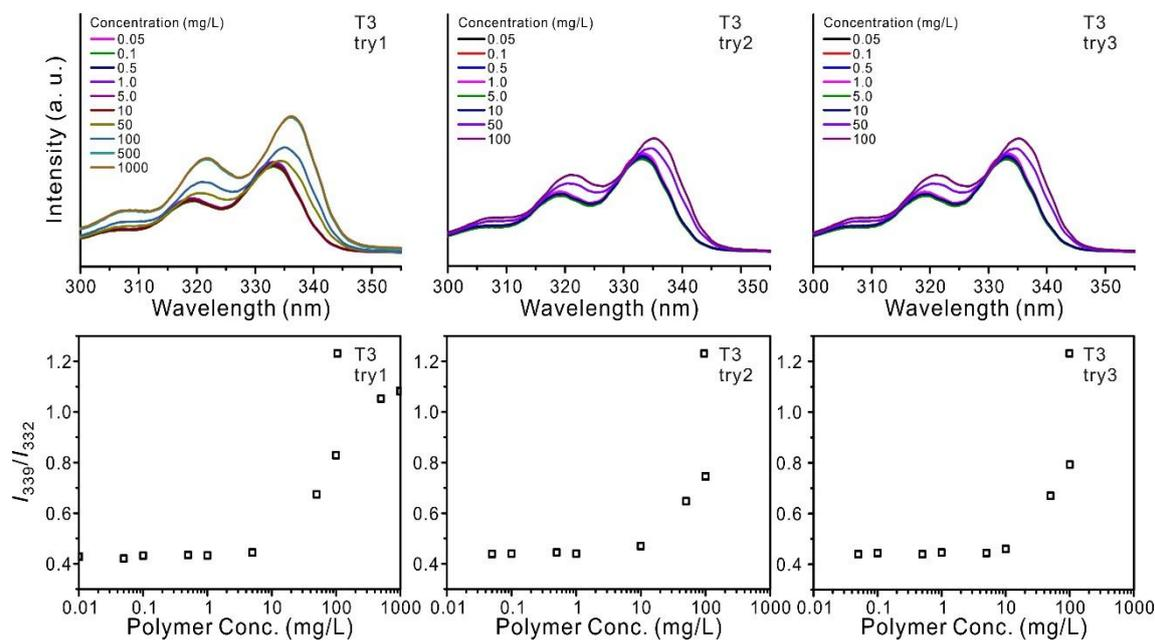
**Fig. S6** Excitation spectra of pyrene in aqueous solution and determination of CMC for PEG<sub>114</sub>-*b*-P(EEGE-*co*-TGE)<sub>7/19</sub> (**T3**) micelles ( $\lambda_{\text{cm}} = 372$  nm). CMC was calculated *via* measurements of  $I_{339}/I_{332}$  as a function of polymer concentration using the fluorescence excitation spectra of pyrene.
