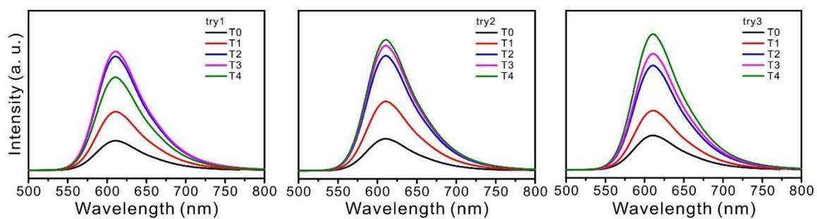
**Fig. S10** Emission spectra of Nile Red in acetone after freeze-drying of aqueous solution of all **T0 – T4** micelles for the calculation of encapsulation efficiency ( $\lambda_{\text{ex}} = 480 \text{ nm}$ ).
