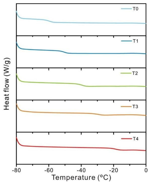
**Fig. S2** DSC thermograms for PEG<sub>114</sub>-*b*-P(EEGE-*co*-TGE)<sub>m/n</sub> copolymers (**T0** – **T4**). The melting temperature of PEG block was observed at 50 – 54 °C.
