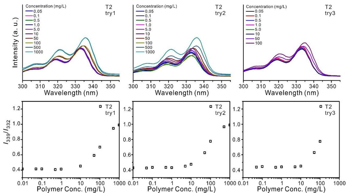
**Fig. S5** Excitation spectra of pyrene in aqueous solution and determination of CMC for PEG<sub>114</sub>-*b*-P(EEGE-*co*-TGE)<sub>14/14</sub> (T2) micelles ( $\lambda_{em} = 372$  nm). CMC was calculated *via* measurements of  $I_{339}/I_{332}$  as a function of polymer concentration using the fluorescence excitation spectra of pyrene.
