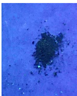
Figure S15. Visual fluorescence photograph of P2-3-CuCl under 365 nm UV lamp.
