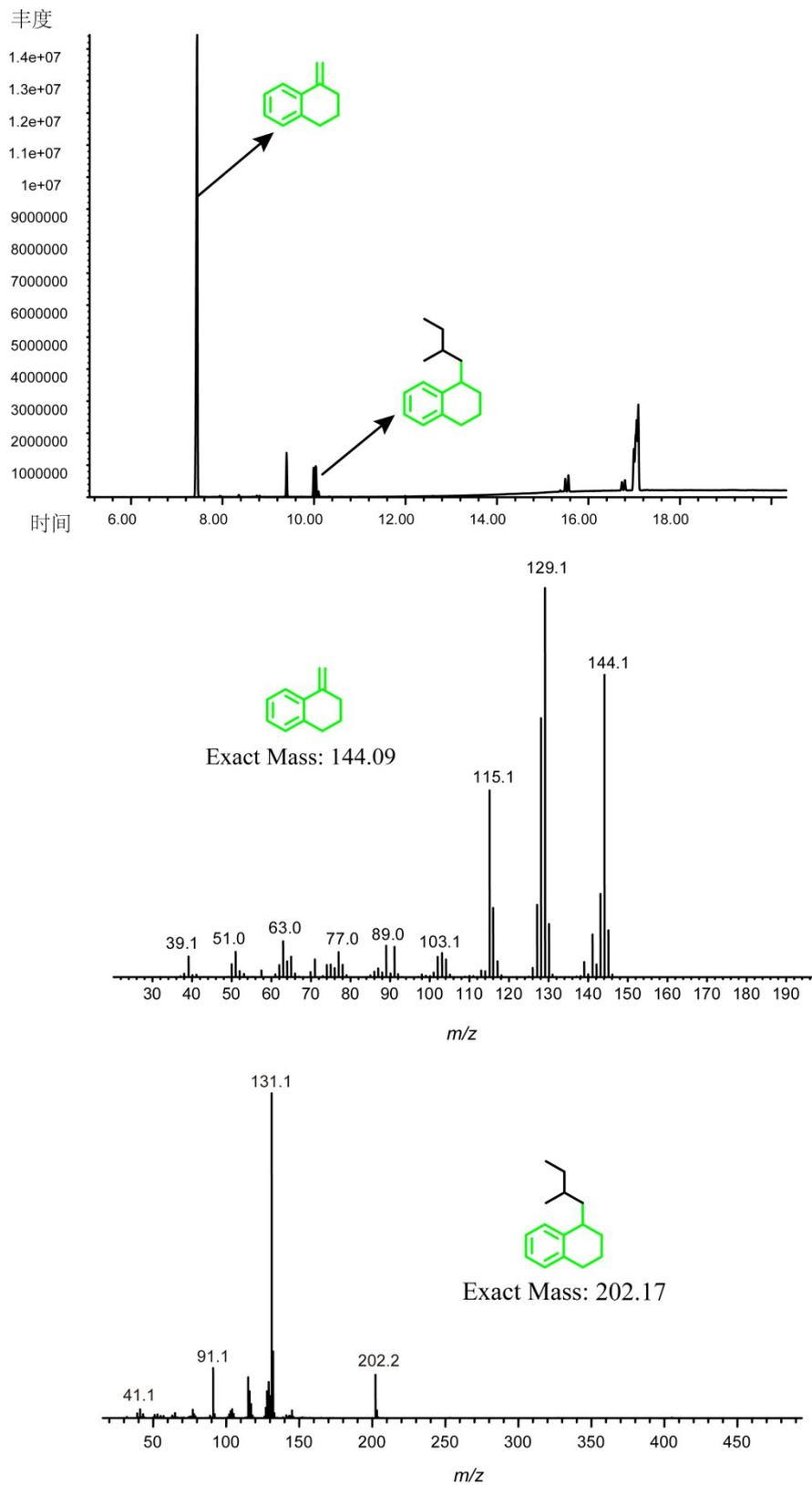
Fig. S8. GC curves and mass spectra of THNE and Mono-adducts THNE during living anionic homopolymerization
