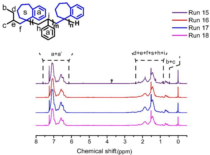
Fig. S13.  $^1\text{H}$  NMR spectra result of the copolymer of THBE with St
