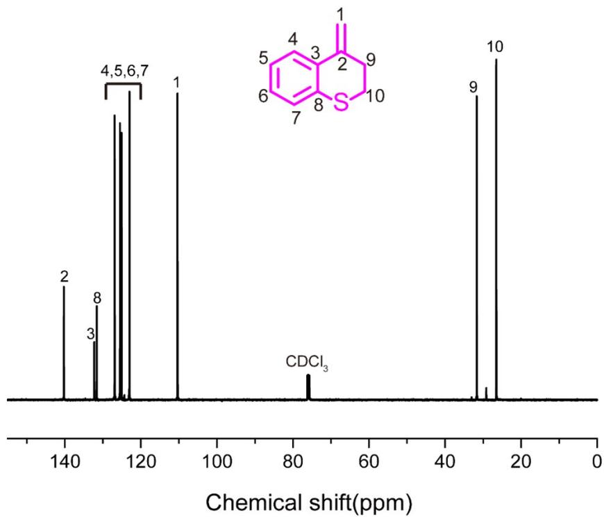
Fig. S19. <sup>13</sup>C NMR spectra of META
