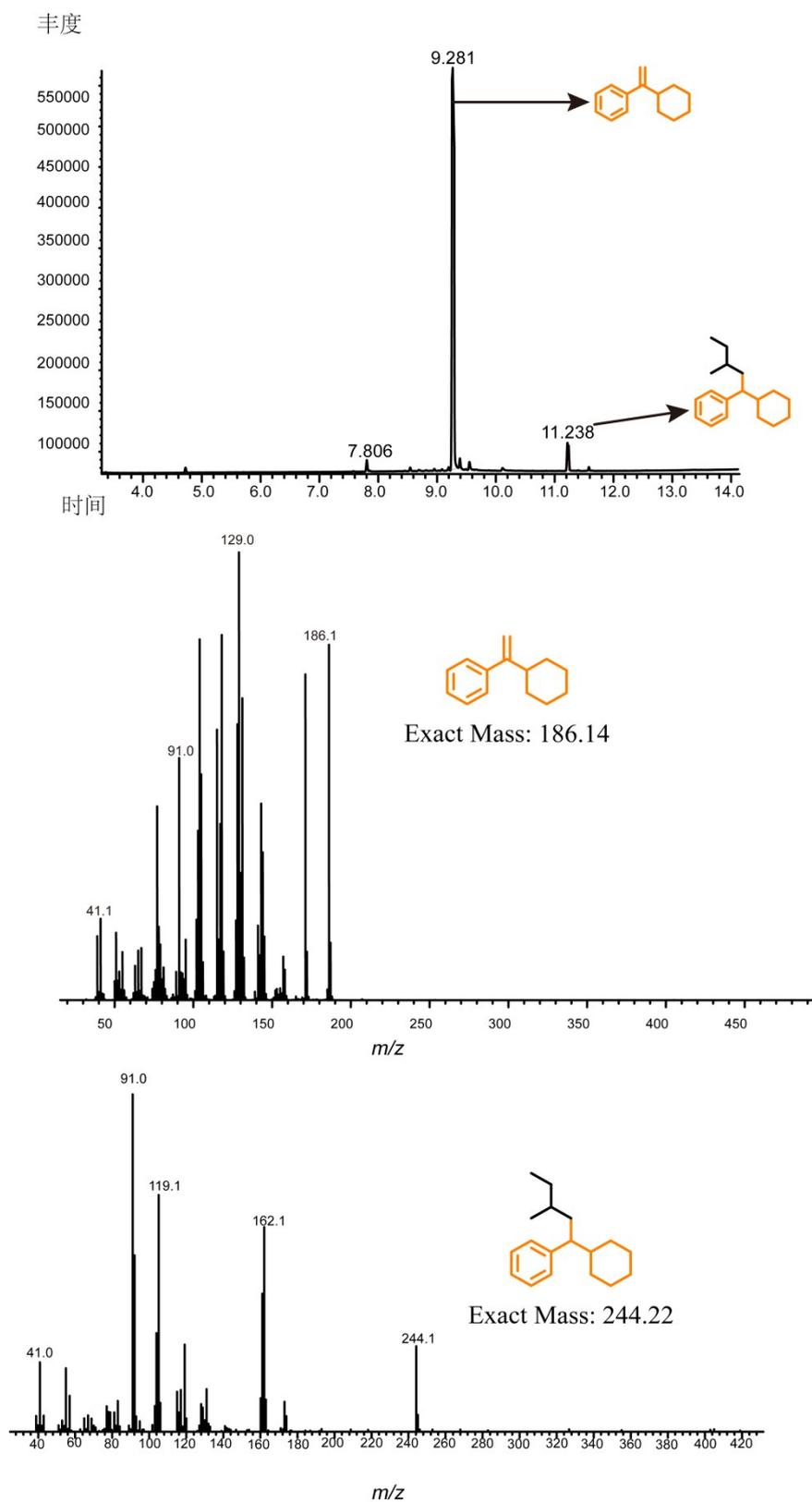
Fig.S7. GC curves and mass spectra of CHBE and Mono-adducts CHBE during living anionic homopolymerization
