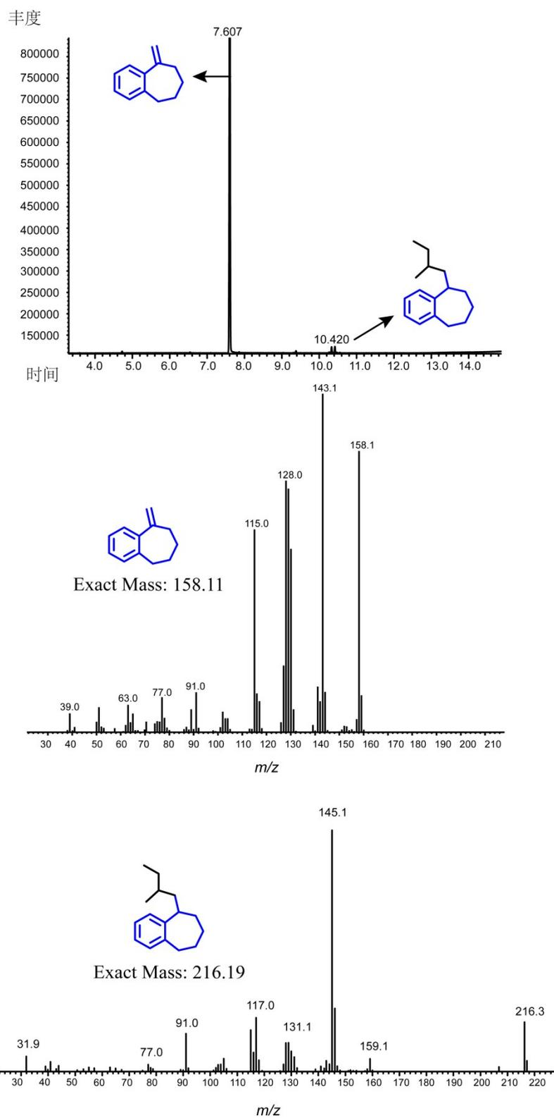
Fig. S9. GC curves and mass spectra of THBE and Mono-adducts THBE during living anionic homopolymerization
