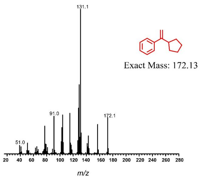
Fig.S1.<sup>1</sup>H NMR and EI-mass spectra of CPBE
