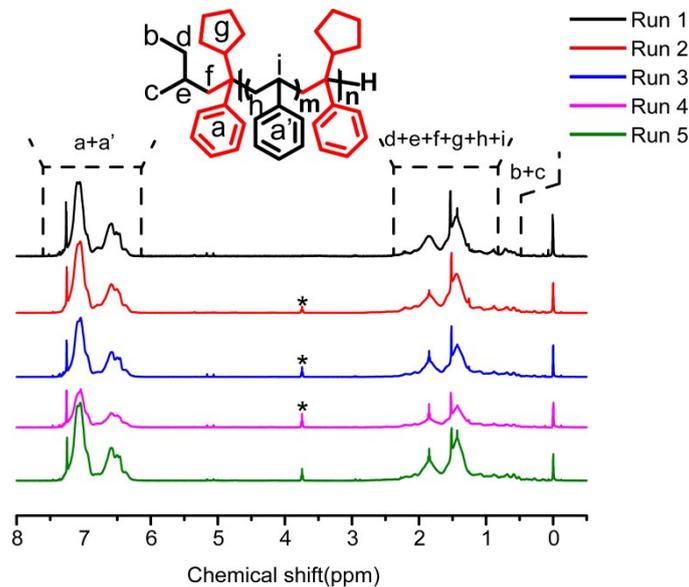
Fig.S11.  $^1\text{H}$  NMR spectra result of the copolymer of CPBE with St
