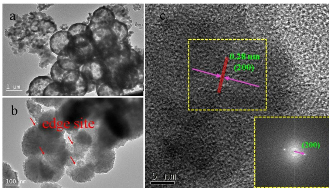
**Figure S4.** TEM images (a and b) and HRTEM image (c) of the  $\text{NiS}_2$ , and the inset is FFT (fast-Fourier transform) image obtained from the yellow square region.
