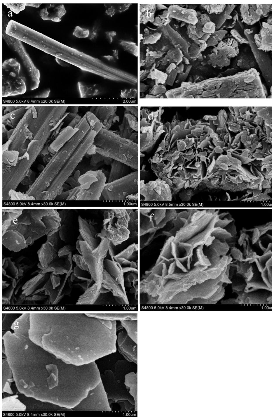
**Figure S1.** SEM images of precursors: (a) Ni/Co=1/0, (b) Ni/Co=4/1, (c) Ni/Co=3/1, (d) Ni/Co=1/1, (e) Ni/Co=1/3, (f) Ni/Co=1/4, and (g) Ni/Co=0/1
