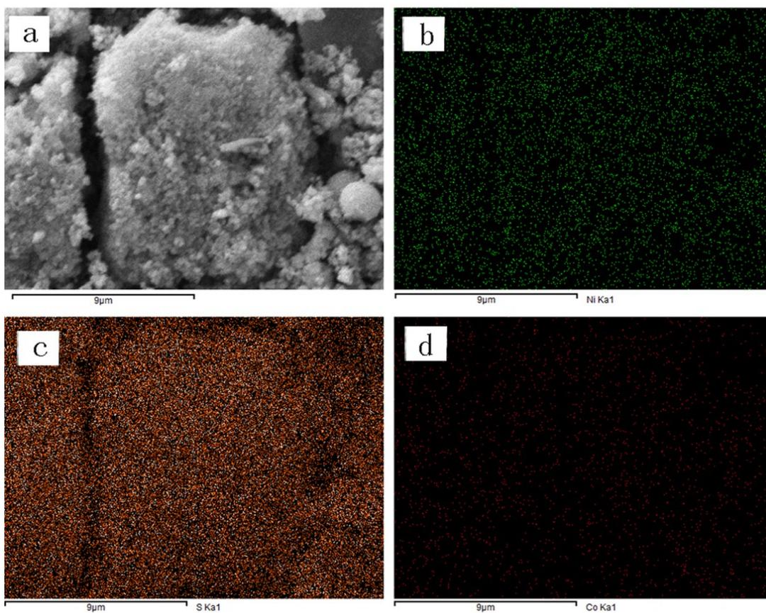
**Figure S3.** Elemental mapping of the  $\text{Ni}_{0.75}\text{Co}_{0.25}\text{S}_2$ .
