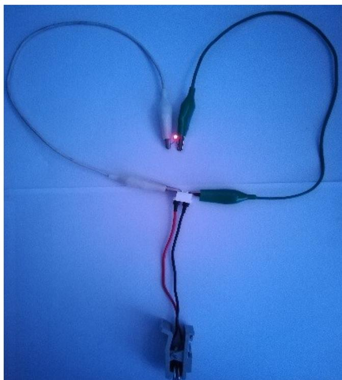
**Figure S5.** A photograph of a red LED lighted up by two supercapacitors in series
