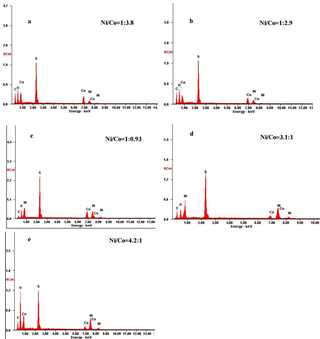
**Figure S2.** EDS spectra of samples: (a)  $\text{Ni}_{0.2}\text{Co}_{0.8}\text{S}_2$ , (b)  $\text{Ni}_{0.25}\text{Co}_{0.75}\text{S}_2$ , (c)
