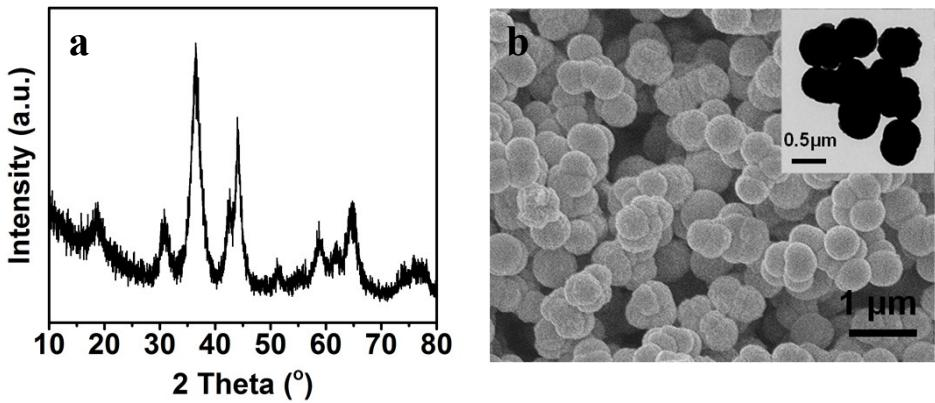
Fig.S7 (a) The XRD pattern and (b) SEM image of the obtained *s*-Co<sub>2</sub>-Ni<sub>1</sub>-O (solid spheres), the inset is the corresponding TEM image. As shown in Fig. S7a, XRD pattern shows the *s*-Co<sub>2</sub>-Ni<sub>1</sub>-O can be indexed to spinel NiCo<sub>2</sub>O<sub>4</sub>, SEM and TEM images shown in Fig. S7b reveal that *s*-Co<sub>2</sub>-Ni<sub>1</sub>-O is composed of solid spheres with size of 0.5-0.8 μm.
