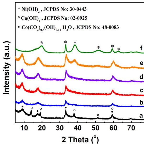
Fig. S3 XRD patterns of (a) CoI, (b) *h*-C<sub>6</sub>N<sub>1</sub>I, (c) *h*-C<sub>2</sub>N<sub>1</sub>I (d) *h*-C<sub>1</sub>N<sub>1</sub>I (e) *h*-C<sub>1</sub>N<sub>6</sub>I and (f) NiI.
