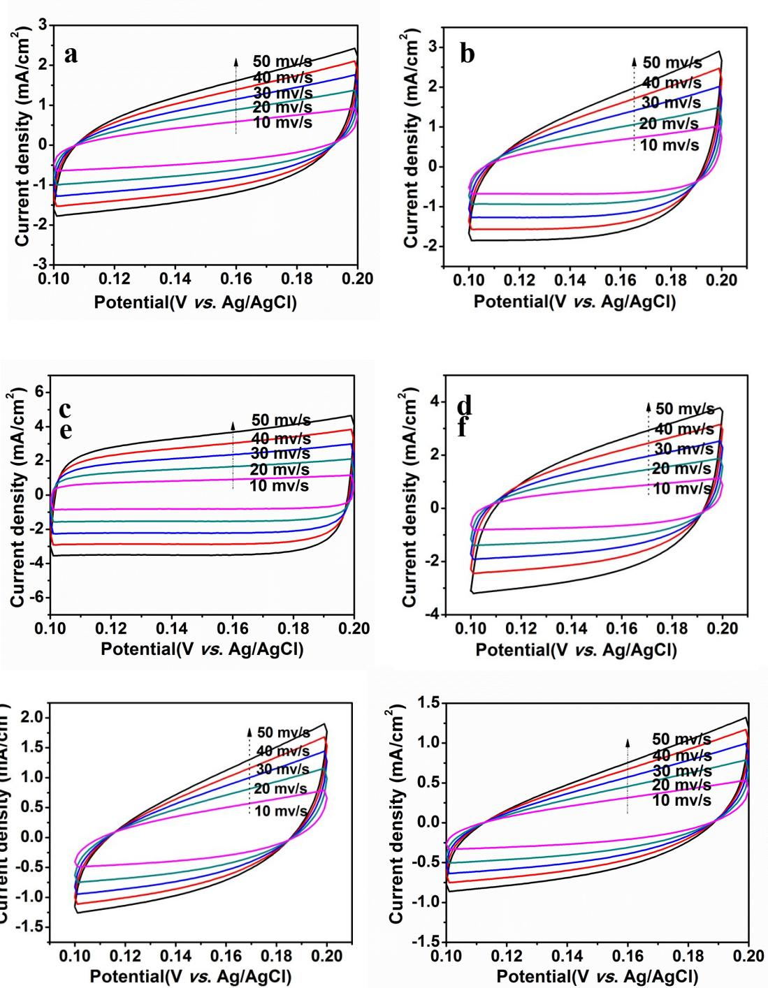
Fig.S10 Cyclic voltammetry (CV) curves of (a)  $\text{Co}_3\text{O}_4$ , (b)  $\text{Co}_6\text{-Ni}_1\text{-O}$ , (c)  $\text{Co}_2\text{-Ni}_1\text{-O}$  (d)  $\text{Co}_1\text{-Ni}_1\text{-O}$  (e)  $\text{Co}_1\text{-Ni}_6\text{-O}$  and (f)  $\text{NiO}$  tested at various scan rates from 10 to 50  $\text{mV s}^{-1}$ .
