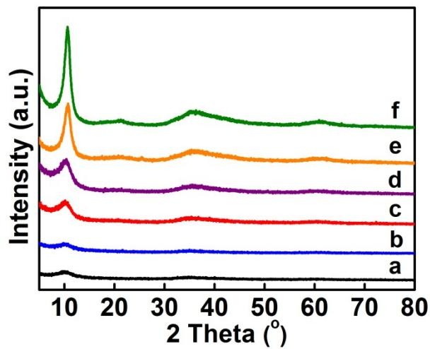
Fig. S1 XRD patterns of (a) s-CoA, (b) *s*-C<sub>6</sub>N<sub>1</sub>A, (c) *s*-C<sub>2</sub>N<sub>1</sub>A (d) *s*-C<sub>1</sub>N<sub>1</sub>A (e) *s*-C<sub>1</sub>N<sub>6</sub>A and (f) s-NiA.
