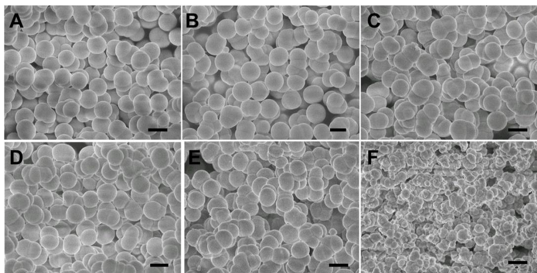
Fig. S2 SEM images of (A) s-CoA, (B) *s*-C<sub>6</sub>N<sub>1</sub>A, (C) *s*-C<sub>2</sub>N<sub>1</sub>A (D) *s*-C<sub>1</sub>N<sub>1</sub>A (E) *s*-C<sub>1</sub>N<sub>6</sub>A and (F) s-NiA. Scale bar: 1μm
