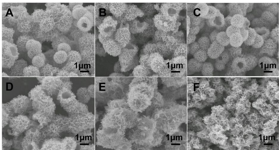
Fig.S5 SEM images of (A) Co<sub>3</sub>O<sub>4</sub>, (B) Co<sub>6</sub>-Ni<sub>1</sub>-O, (C) Co<sub>2</sub>-Ni<sub>1</sub>-O (D) Co<sub>1</sub>-Ni<sub>1</sub>-O (E) Co<sub>1</sub>-Ni<sub>6</sub>-O and (F) NiO.
