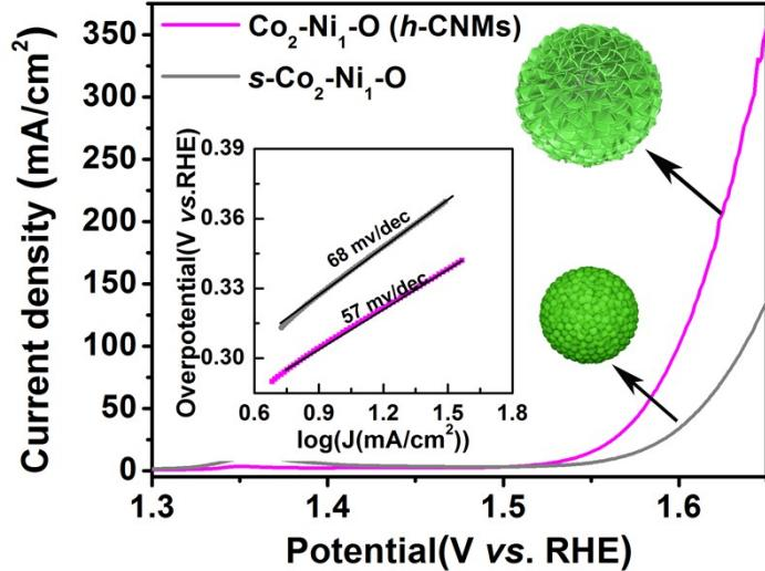
Fig. S8 LSV curves of Co<sub>2</sub>-Ni<sub>1</sub>-O and *s*-Co<sub>2</sub>-Ni<sub>1</sub>-O, the inset is the corresponding Tafel slopes.
