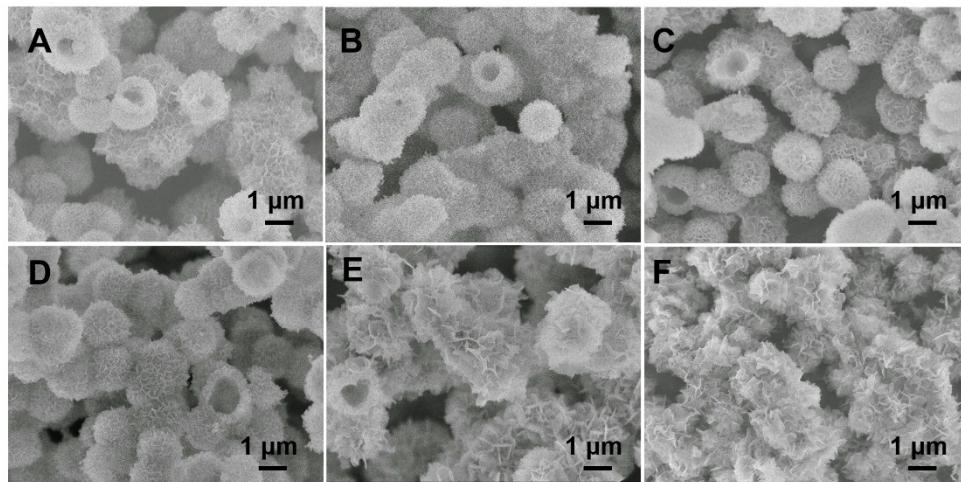
Fig. S4 SEM images of (A) CoI, (B)  $h$ -C<sub>6</sub>N<sub>1</sub>I, (C)  $h$ -C<sub>2</sub>N<sub>1</sub>I (D)  $h$ -C<sub>1</sub>N<sub>1</sub>I (E)  $h$ -C<sub>1</sub>N<sub>6</sub>I and (F) NiI.
