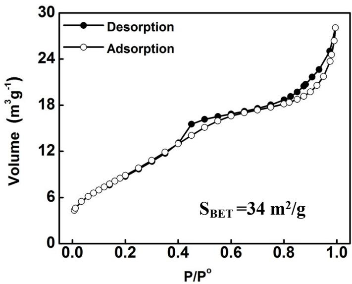
Fig. S9 N<sub>2</sub> adsorption-desorption isotherms of s-Co<sub>2</sub>-Ni<sub>1</sub>-O.
