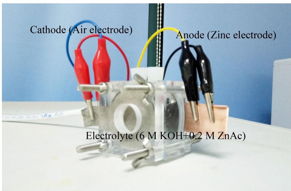
**Figure S5** The self-assembled rechargeable Zn-air battery test installation: the cathode (red electrode clip) was the carbon cloth and nickel foam; the anode (black electrode clip) was the zinc flake conducted by the copper slice; the electrolyte was 6 M KOH aqueous solution containing 0.2 M ZnAc.
