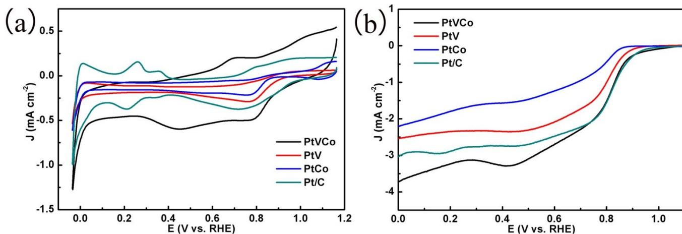
**Figure S4** (a) CV curves of PtVCo, PtV, PtCo and commercial Pt/C under static condition in 0.1 M KOH solution at a scan rate of 10 mV s<sup>-1</sup>. (b) LSV curves of PtVCo, PtV, PtCo and commercial Pt/C in a O<sub>2</sub>-saturated 0.1 M KOH solution at a rotation rate of 1600 rpm.
