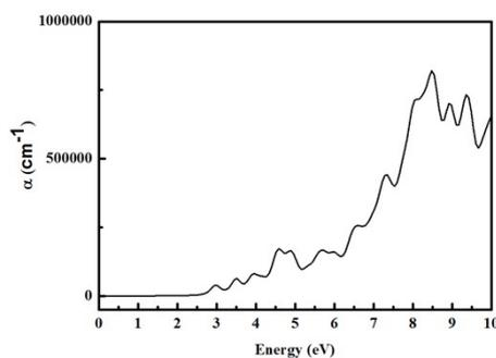
Figure S2 The theoretical Absorption spectrum of SnO<sub>2</sub> by HSE06.
