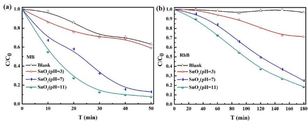
Figure S6 (a) and (b) Photocatalytic degradation curves of MB and RhB at pH (= 3, 7, 11), respectively.
