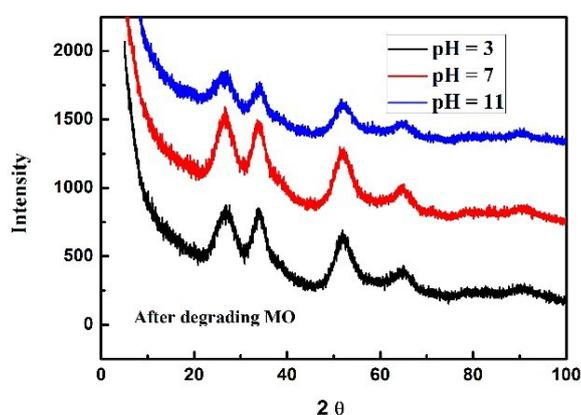
Figure S12 XRD patterns of SnO<sub>2</sub> after the photocatalytic reaction of degrading MO (pH=3, 7, 11), respectively.
