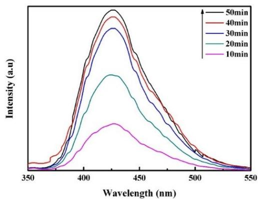
Figure S14. Hydroxyl radical ·OH detecting photoluminescence (PL) spectra of SnO<sub>2</sub> in TA solution under UV light irradiation.
