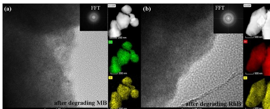
Figure S10 (a) and (b). TEM image, Elemental mapping in HADDF image and Electron diffraction image of photo-catalyst SnO<sub>2</sub> after degrading MB and RhB (pH=7), respectively.
