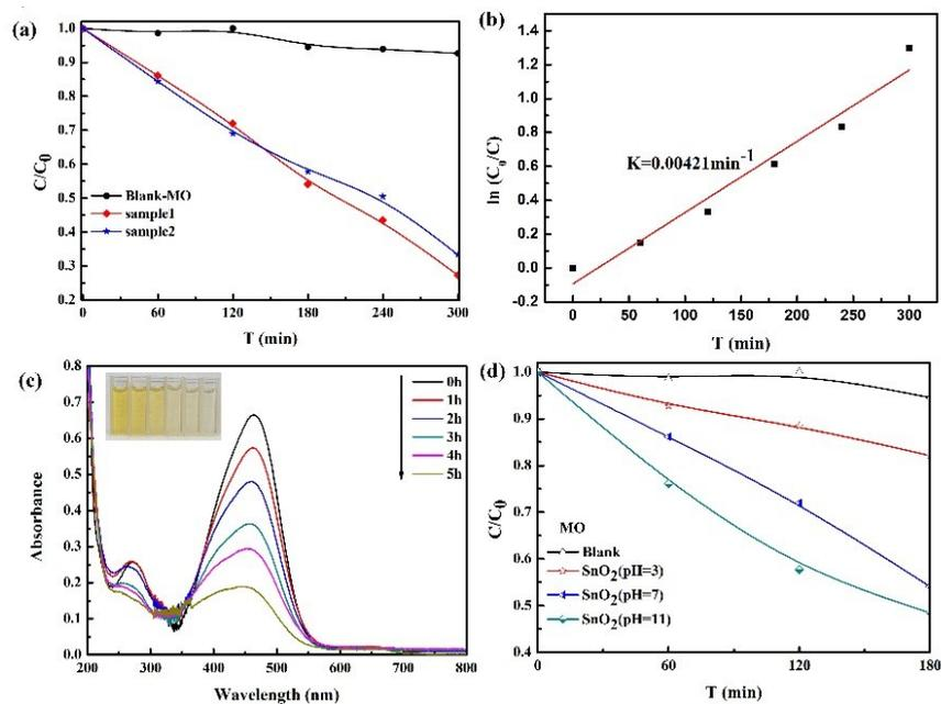
Figure S11 (a) photocatalytic degradation curves of MO. (b) The corresponding  $\ln C_0/C$  as a function of time. (c) UV visible absorption of MO as function of irradiation time for nano-particle SnO<sub>2</sub> (inset: the photograph for different irradiation time). (d) Photocatalytic degradation curves of MO at pH (=3, 7, 11).
