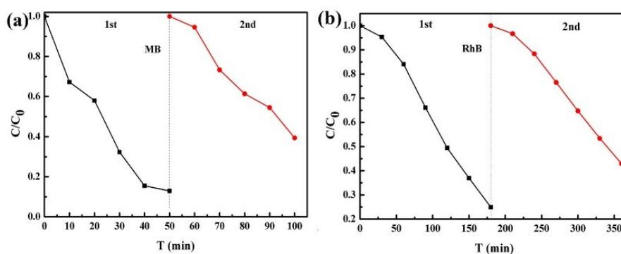
Figure S7 (a) and (b) the cycle performance of amorphous SnO<sub>2</sub> for photo-degradation of MB and RhB, respectively.
