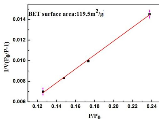
Fig S3. The specific surface area determination is performance by BET measurement with  $\text{N}_2$  absorption at 77K.
