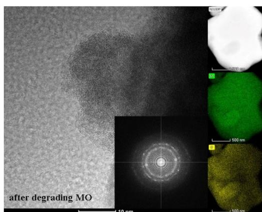
Figure S13 TEM image, Elemental mapping in HADDF image and Electron diffraction image of photo-catalyst SnO<sub>2</sub> after degrading MO (pH=7), respectively.
