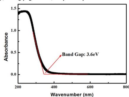
Figure S1 UV-vis spectrum of SnO<sub>2</sub>.
