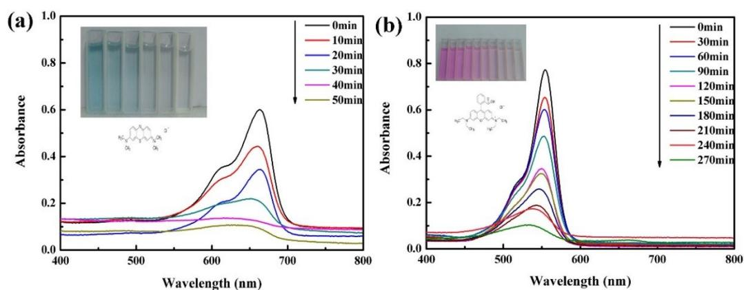
Figure S4 (a) and (b) UV visible absorption of MB and RhB as function of irradiation time for amorphous  $\text{SnO}_2$ , respectively (inset: the photograph for different irradiation time).
