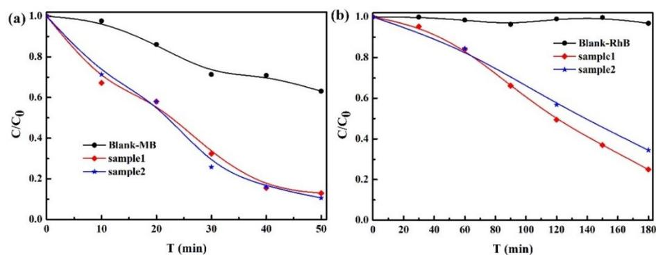
Figure S8 (a) and (b). Photocatalytic degradation curves of MB and RhB using different batches of SnO<sub>2</sub>, respectively.
