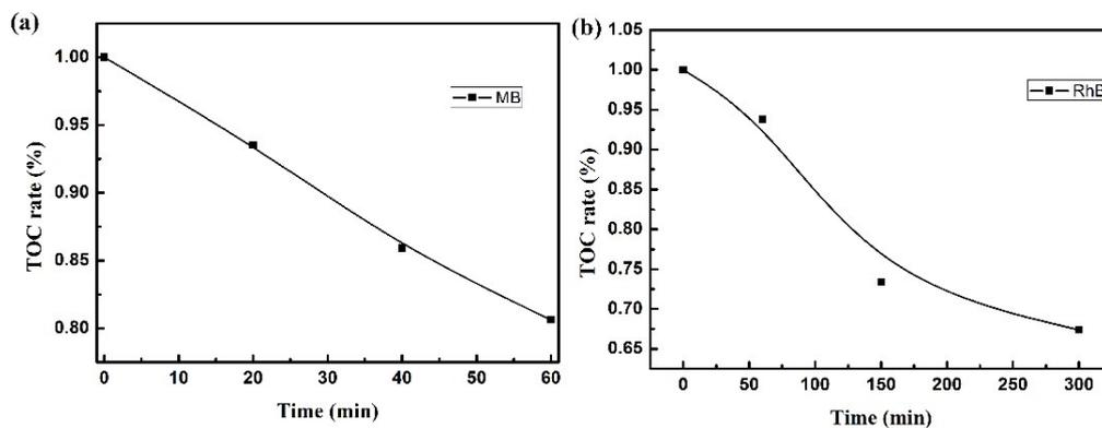
Figure S5 (a) and (b) TOC curve of MB and RhB photocatalytic degradation by nano particle  $\text{SnO}_2$ , respectively.
