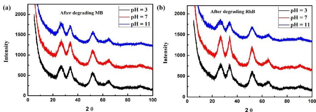
Figure S9 (a) and (b) XRD patterns of SnO<sub>2</sub> after the photocatalytic reaction of degrading MB and RhB (pH=3, 7, 11), respectively.
