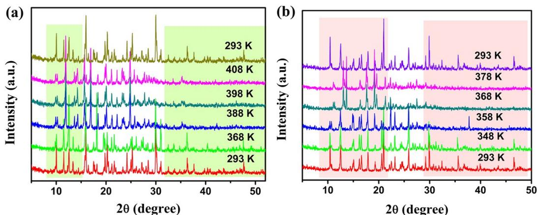
**Fig. S5** Variable-temperature PXRD patterns of compounds **1** (a) and **2** (b).
