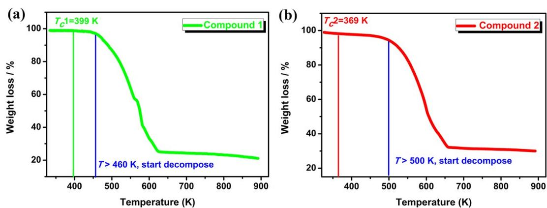
**Fig. S3** TGA curves for **1** (a) and **2** (b).
