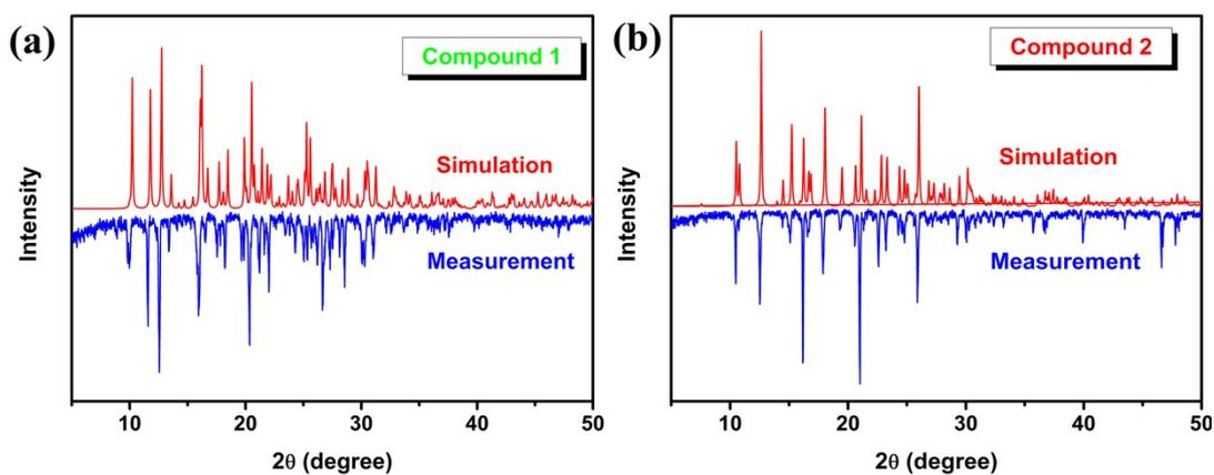
**Fig. S2** Experimental powder diffraction (PXRD) patterns of compounds **1** (a) and **2** (b), which match very well with the simulated patterns in terms of the crystal structures at 293 K, respectively.
