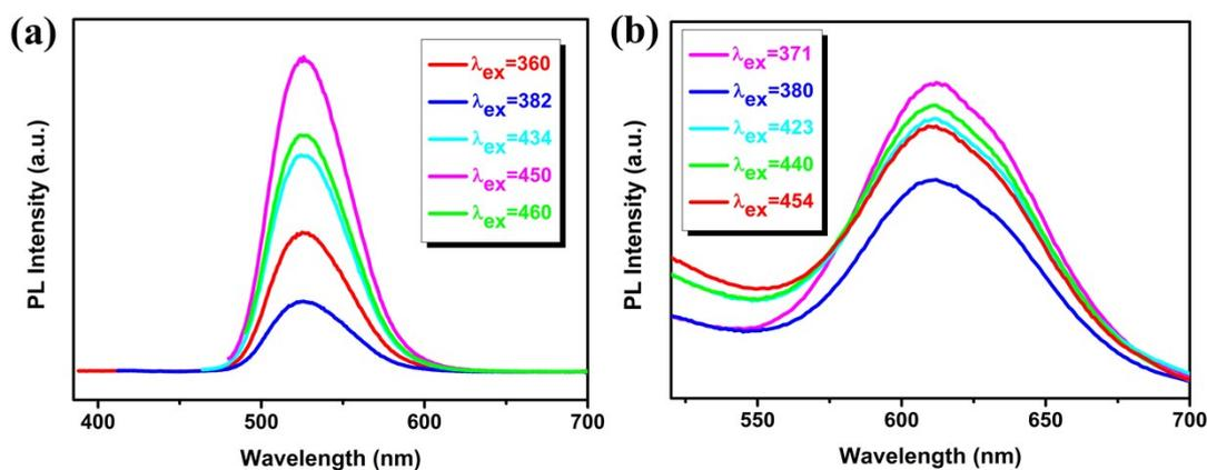
**Fig. S10** The emission spectra of **1** (a) at the excitation wavelength of 360 nm, 382 nm, 434 nm, 450 nm and 460 nm and **2** (b) at 371 nm, 380 nm, 423 nm, 440 nm and 454 nm.
