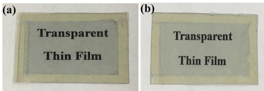
**Fig. S11** Transparent thin films of **1** (a) and **2** (b) were fabricated on PET substrates plane by spin-coating method.
