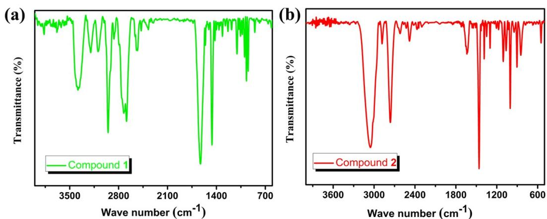
**Fig. S1** Infrared (IR) spectra of solids **1** (a) and **2** (b) in KBr pellet recorded on a Shimadzu model IR-60 spectrometer at room temperature.
