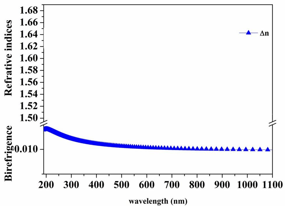
**Fig. S10** The obtained birefringence of  $\text{Li}_3\text{KB}_9\text{O}_{15}\text{F}$ .
