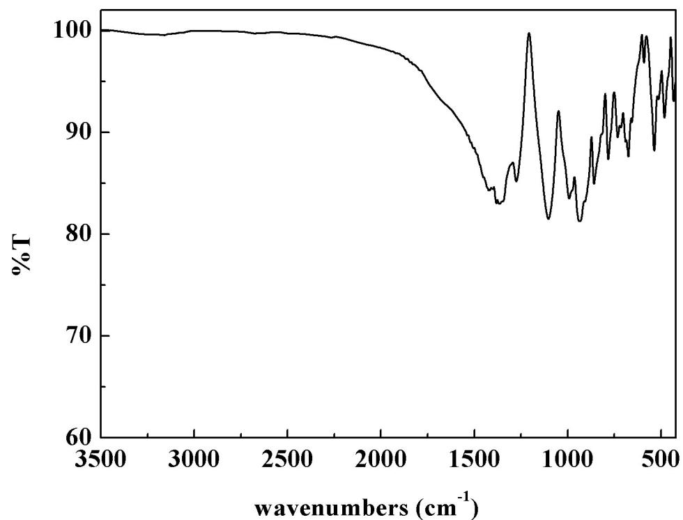
**Fig. S9** Infrared spectrum of  $\text{Li}_3\text{KB}_9\text{O}_{15}\text{F}$ .
