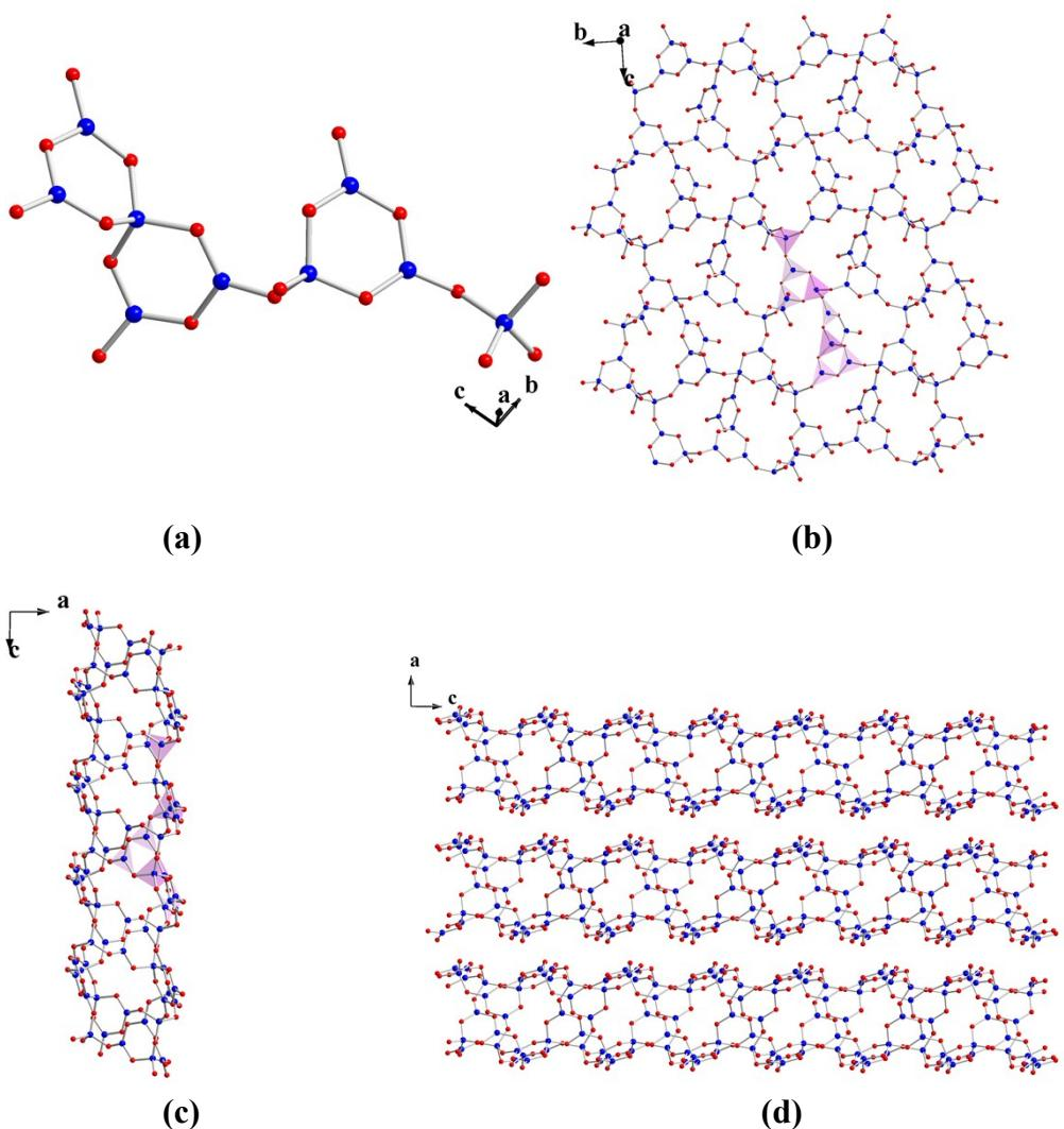
**Fig. S7** Crystal structure of  $\text{Na}_2\text{B}_6\text{O}_{10}$ . (a) FBB  $\text{B}_9\text{O}_{19}$ ; (b) The 2D layered structure viewed in the  $bc$  plane for single chains; (c) and (d) The double-layered structure viewed along the  $b$  axis.
