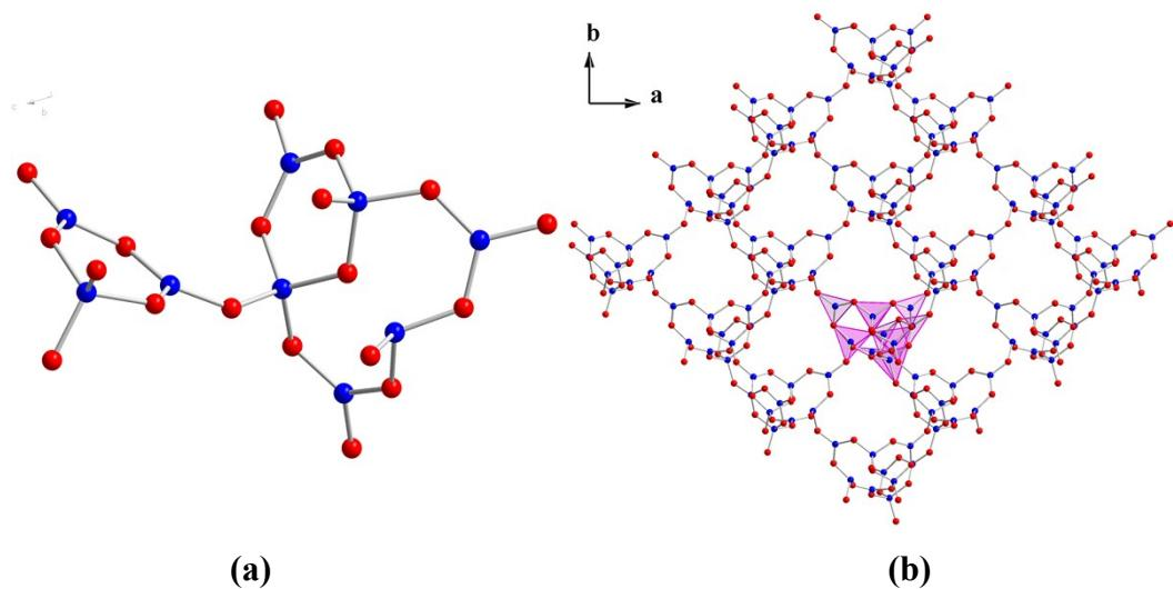
**Fig. S8** Crystal structure of  $\text{Na}_2\text{B}_9\text{O}_{15}(\text{H}_2\text{O})(\text{H}_3\text{O})$ . (a) FBB  $\text{B}_9\text{O}_{19}$ ; (b) The 3D open framework formed through sharing O atoms between  $\text{B}_3\text{O}_7$  and  $\text{B}_6\text{O}_{13}$  clusters, in which big channels are observed along the *b* axis.
