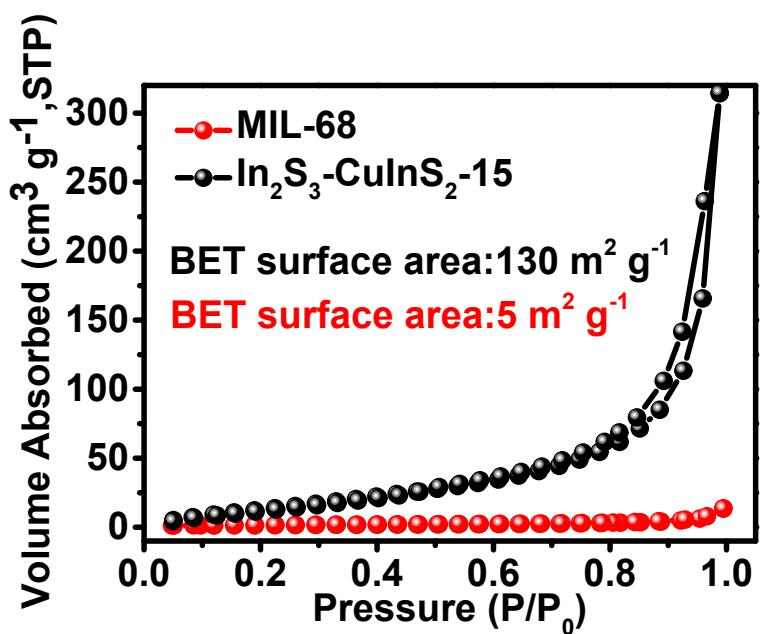
**Figure S10.** N<sub>2</sub> adsorption-desorption isotherms of MIL-68 and In<sub>2</sub>S<sub>3</sub>-CuInS<sub>2</sub>-15.
