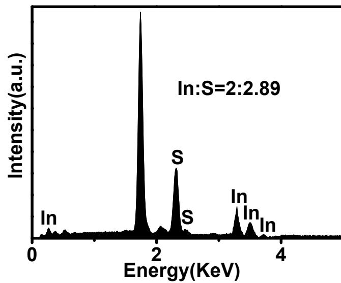
**Figure S3.** EDX spectrum  $\text{In}_2\text{S}_3$ .
