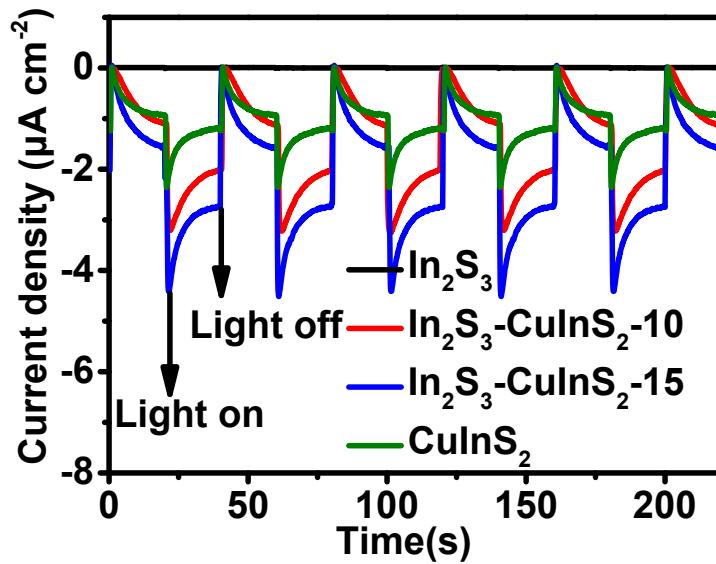
**Figure S15.** The transient photocurrent responses of  $\text{In}_2\text{S}_3$ ,  $\text{In}_2\text{S}_3\text{-CuInS}_2\text{-10}$ ,  $\text{In}_2\text{S}_3\text{-CuInS}_2\text{-15}$  and  $\text{CuInS}_2$ .
