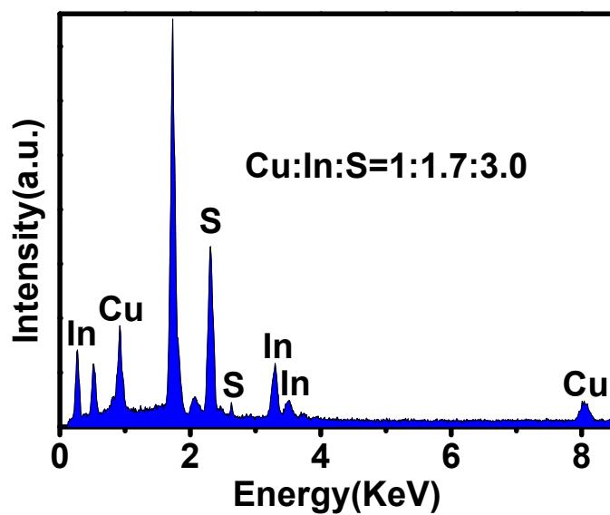
**Figure S5.** EDX spectrum of  $\text{In}_2\text{S}_3$ - $\text{CuInS}_2$ -15.
