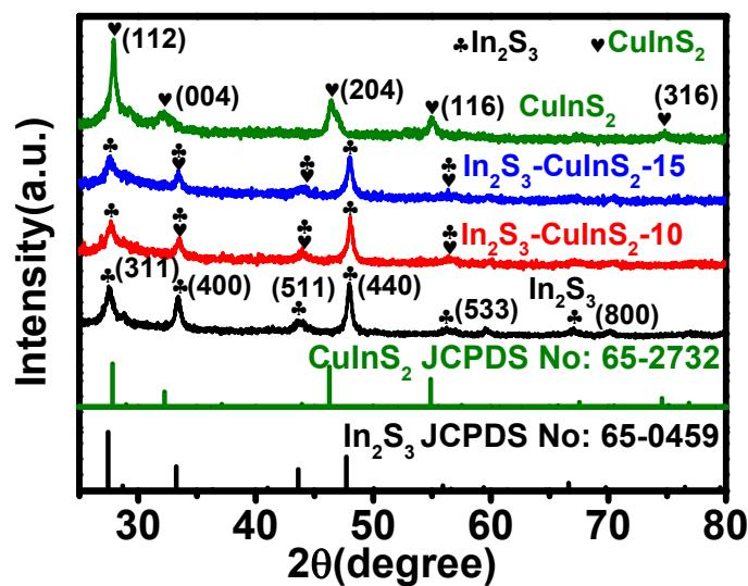
Figure S2. Standard XRD patterns of standard In<sub>2</sub>S<sub>3</sub> and CuInS<sub>2</sub>, XRD patterns of In<sub>2</sub>S<sub>3</sub>, In<sub>2</sub>S<sub>3</sub>-CuInS<sub>2</sub>-10, In<sub>2</sub>S<sub>3</sub>-CuInS<sub>2</sub>-15 and CuInS<sub>2</sub>.
