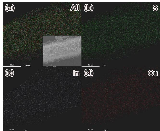
**Figure S7.** Elemental mapping images of  $\text{In}_2\text{S}_3\text{-CuInS}_2\text{-15}$ .
