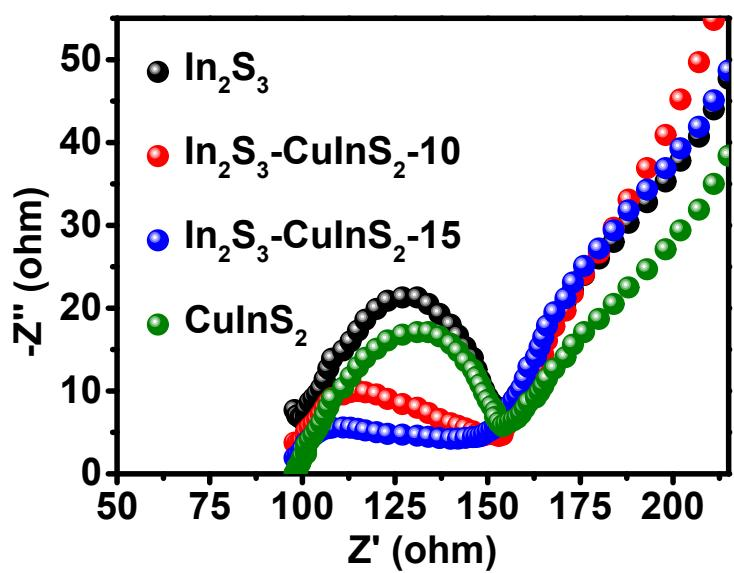
**Figure S16.** Electrochemical impedance spectroscopy (EIS) plots of  $\text{In}_2\text{S}_3$ ,  $\text{In}_2\text{S}_3\text{-CuInS}_2\text{-10}$ ,  $\text{In}_2\text{S}_3\text{-CuInS}_2\text{-15}$  and  $\text{CuInS}_2$ .
