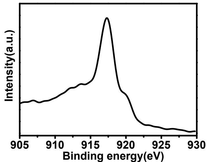
**Figure S11.** The Auger electron spectroscopy of Cu.
