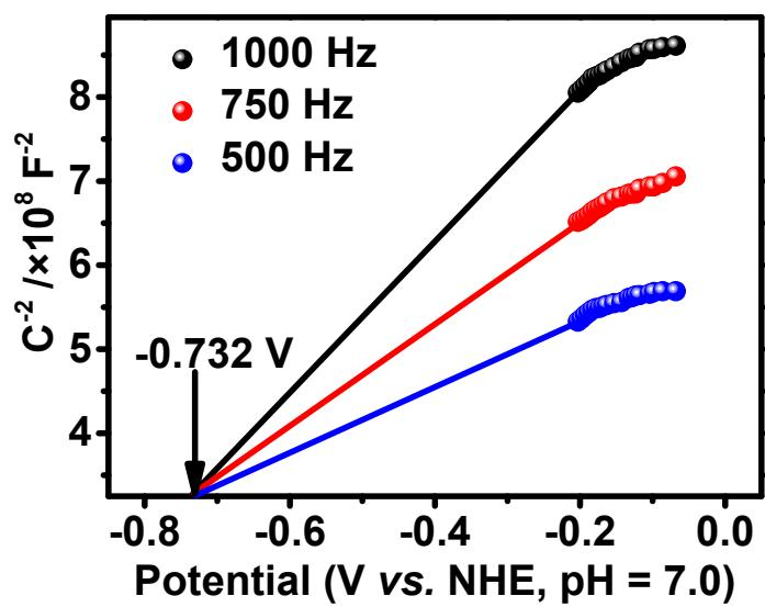
Figure S12. Mott-Schottky plots of pure  $\text{In}_2\text{S}_3$ .
