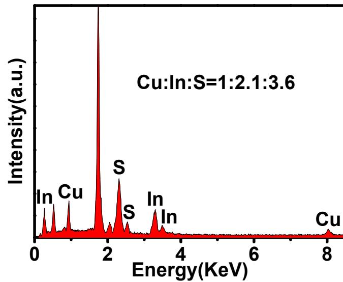
**Figure S4.** EDX spectrum of  $\text{In}_2\text{S}_3\text{-CuInS}_2\text{-10}$ .
