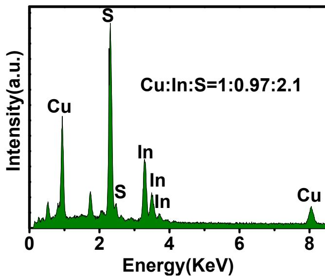
**Figure S6.** EDX spectrum of  $\text{CuInS}_2$ .
