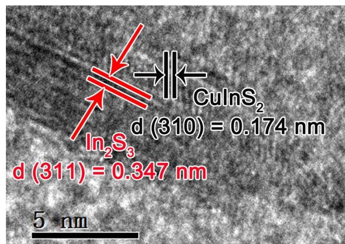
**Figure S8.** High-resolution TEM image of  $\text{In}_2\text{S}_3\text{-CuInS}_2\text{-15}$ .
