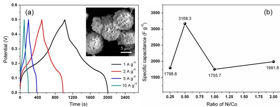
Fig. S12 (a) Galvanostatic charge/discharge curves of Ni-Co LDH with molar ratio of Ni/Co is 1:4, inset shows the SEM image. (b) Relationship plot between discharge specific capacitance and molar ratio of Ni/Co at current density of 1 A g<sup>-1</sup>.
