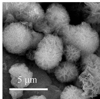
Fig. S13 SEM image of Ni-Co LDH 1/2 electrode after 3000 cycles.
