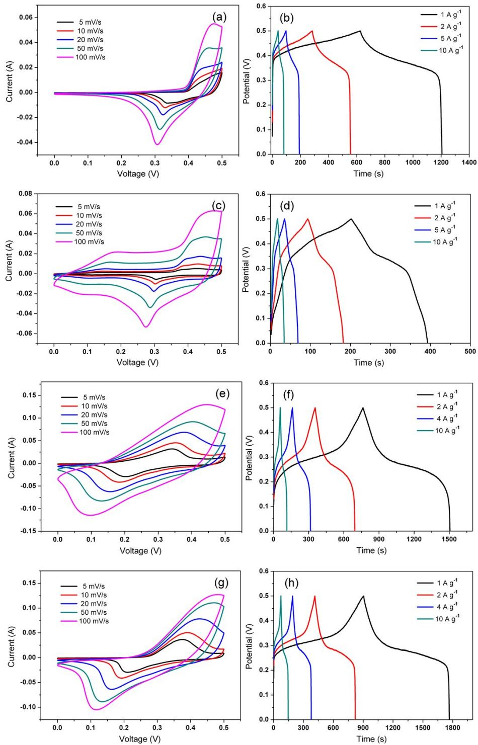
Fig. S11 CV and galvanostatic charge/discharge curves: (a) and (b)  $\text{Ni}(\text{OH})_2$  electrode, (c) and (d)  $\text{Co}(\text{OH})_2$  electrode, (e) and (f) Ni-Co LDH 1/1 electrode and (g) and (h) Ni-Co LDH 2/1 electrode.
