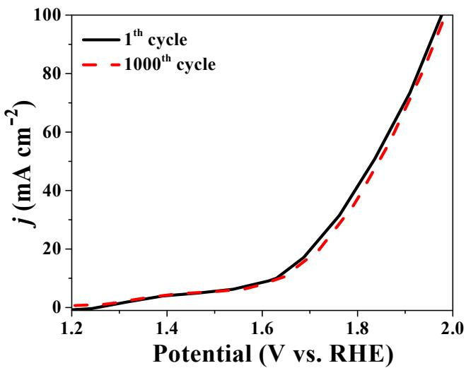
**Fig. S11** Polarization curves of Al-CoP/NF || Al-CoP/NF in a two-electrode setup for full water splitting before and after 1000 CV cycles with scan rate: 100 mV s<sup>-1</sup>.
