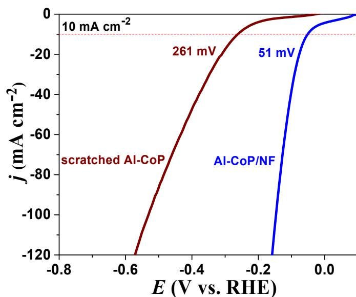
**Fig. S6** Comparison of HER polarization curves of Al-CoP/NF and scratched Al-CoP on Ni foam at a scan rate of  $2 \text{ mV s}^{-1}$  in  $0.5 \text{ M H}_2\text{SO}_4$ .
