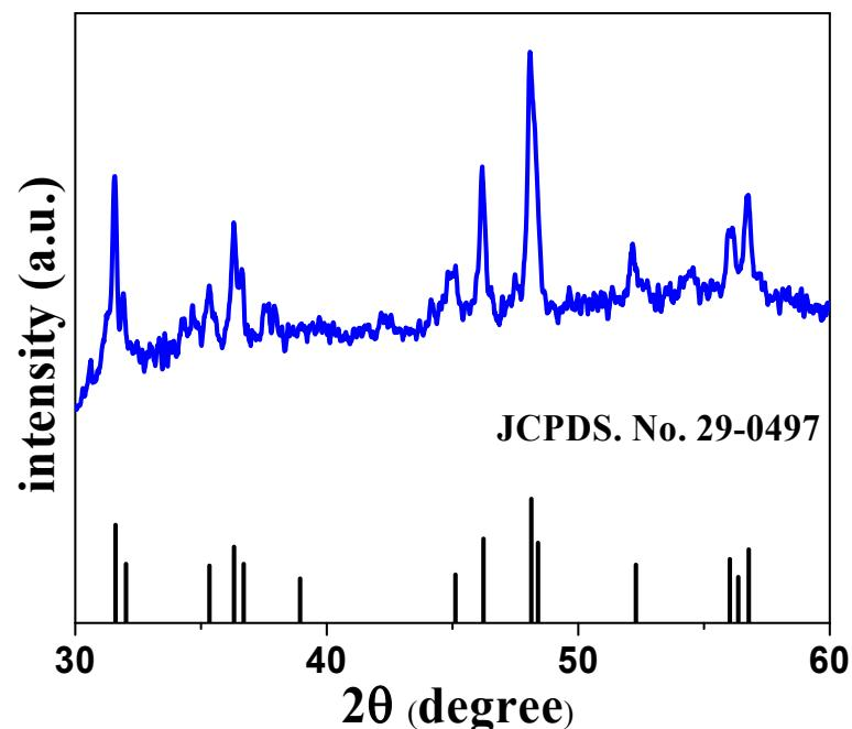
**Fig. S4** XRD pattern of Al-CoP/NF after long-term HER durability test.
