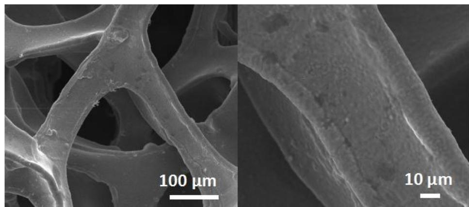
**Fig. S3** SEM image of pristine Ni foam.
