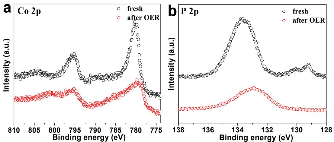
**Fig. S10** XPS spectra of Al-CoP in (a) Co 2p and (b) P 2p regions before and after OER.
