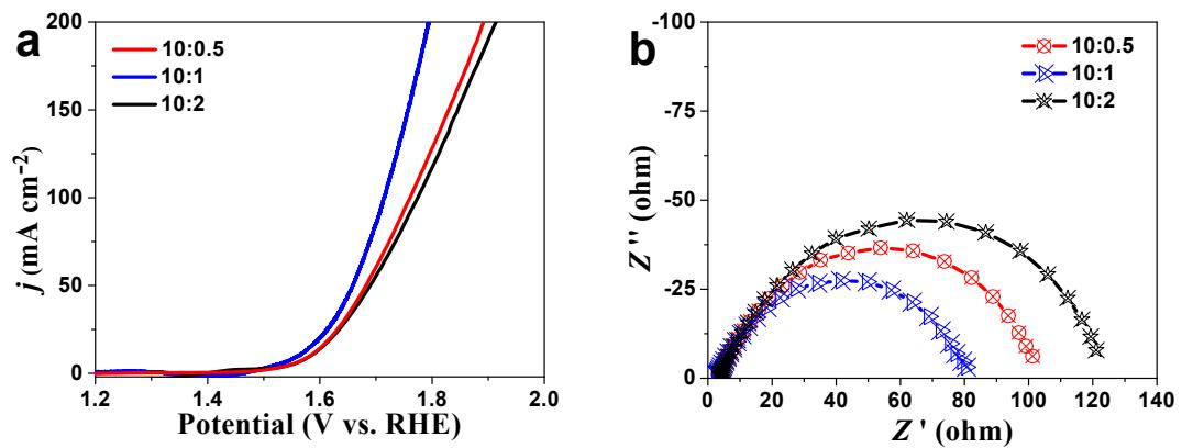
**Fig. S9** (a) Polarization curves for OER (scan rate:  $2 \text{ mV s}^{-1}$ ) and (b) the Nyquist plots of Al-CoP/NF with Co / Al ratios of 10 : 0.5, 10 : 1 and 10 : 2. All experiments were carried out in 1.0 M KOH.
