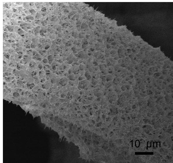
**Fig. S5** SEM image of Al-CoP/NF after long-term HER durability test.
