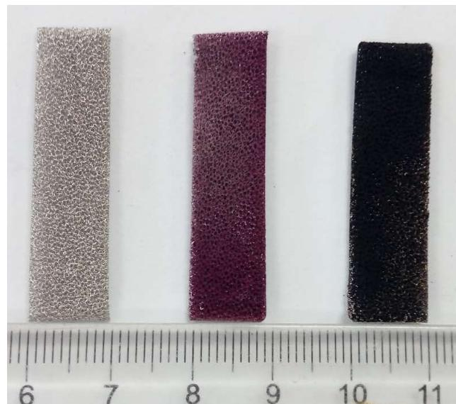
**Fig. S1** Digital photographs of pristine Ni foam, CoAl-LDH/NF and Al-CoP/NF (from left to right).
